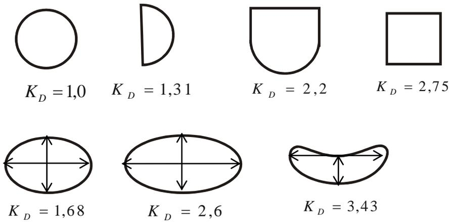
Figure Б.1 – Air intake geometry
