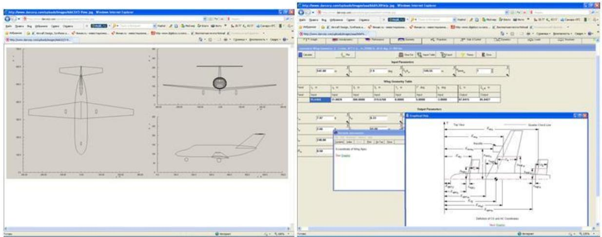
Figure 11.15 – The results of civil airplane conceptual design in AAA
