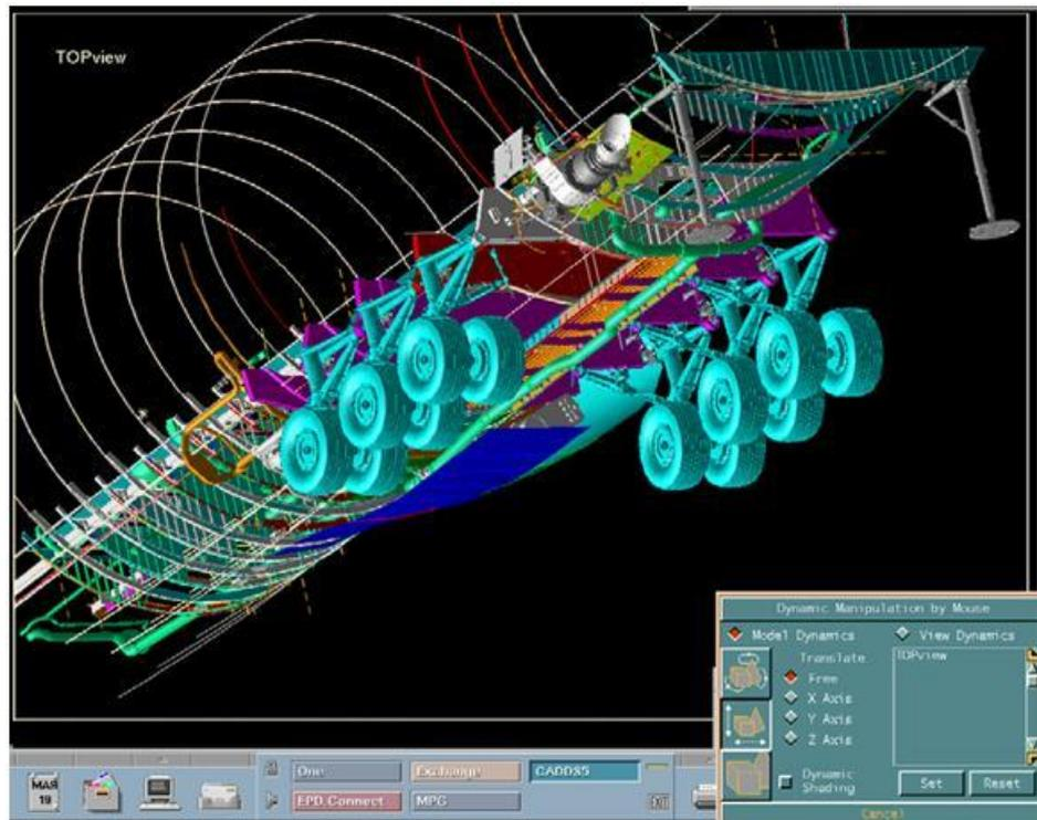
Figure 11.13 – Visualization of the model for the airplane space distribution in CAD/CAE/CAM [35]
