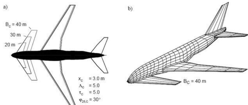
Figure 11.7 – Research of the passenger airplane with “canard” aerodynamic scheme [33]
