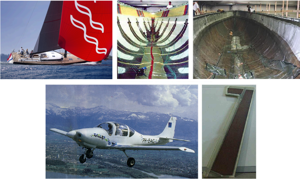
Figure 4.10 Example applications of vacuum infusion: Contest 67CS (upper row) and Eaglet rudder (lower row). Derivative from top left: Copyright 2016 by Contest Yachts, Reprinted with Permission.; Top middle and top right: Copyright 2006 by Lightweight Structures B.V., Reprinted with Permission; bottom row: TU Delft, (n.d.), 4.10-d.jpg and 4.10-e.jpg, Own Work.
