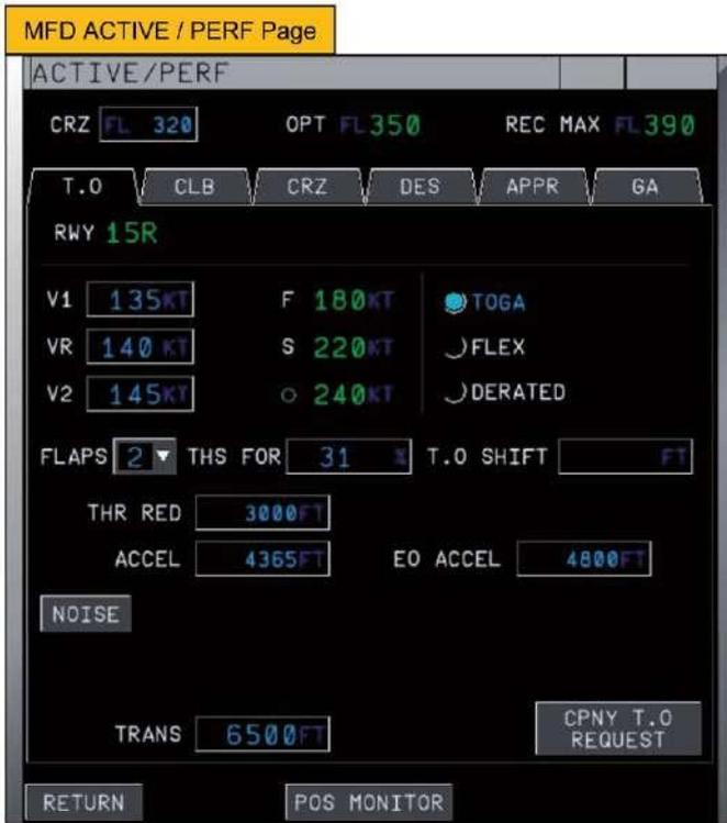
Fig 5.18. 'Active Performance' Page display on MFD (by courtesy of Airbus).
