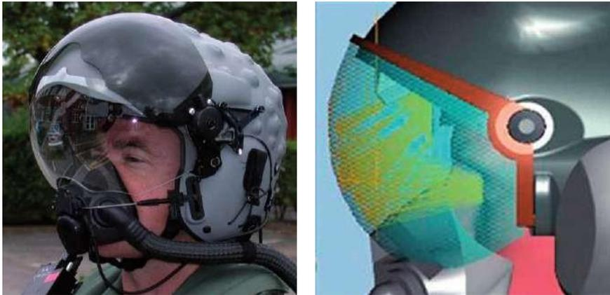
Fig 2.24. Eurofighter Typhoon binocular visor projected HMD (by courtesy of BAE Systems).
