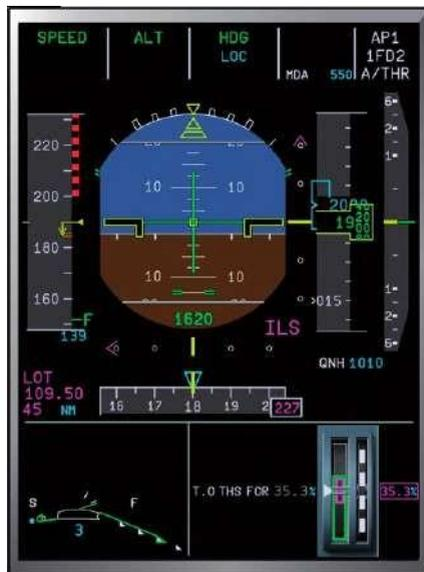
Fig 2.25. Primary flight display (by courtesy of Airbus).
