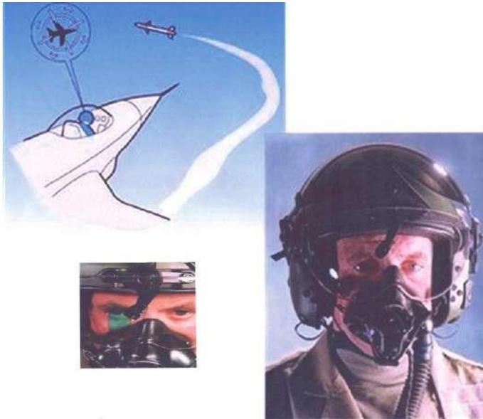
Fig 2.20. Helmet mounted sight and off-boresight missile launch (by courtesy of BAE Systems)
