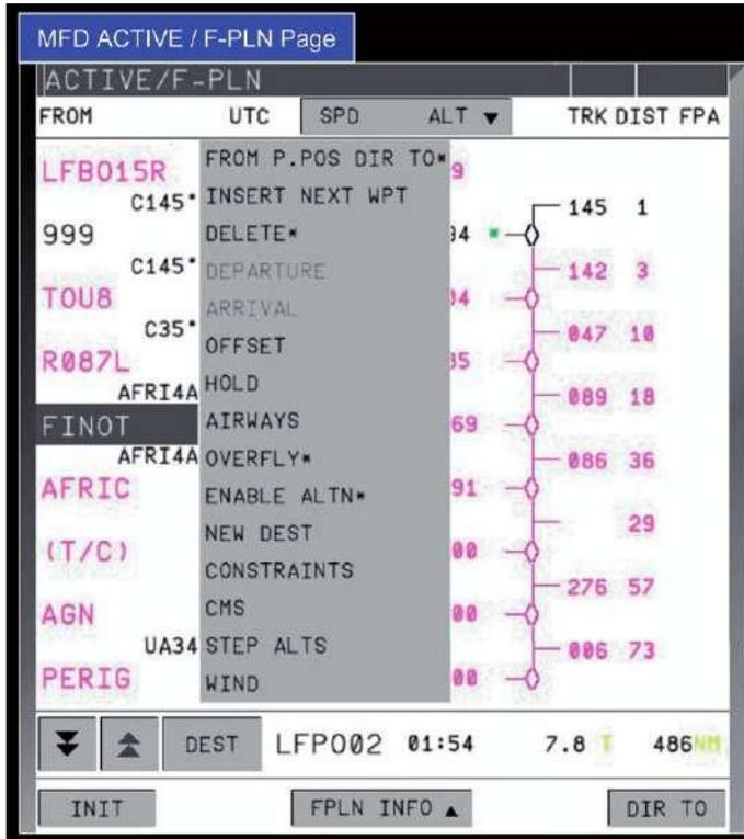
Fig 5.17. 'Active Flight Plan' Page display on MFD (by courtesy of Airbus).
