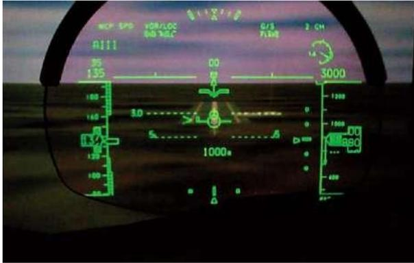
Fig 2.1. Head-up presentation of primary flight information (by courtesy of BAE Systems)
