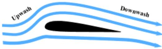
**Figure 4. Airflow Over a Wing[2]**
