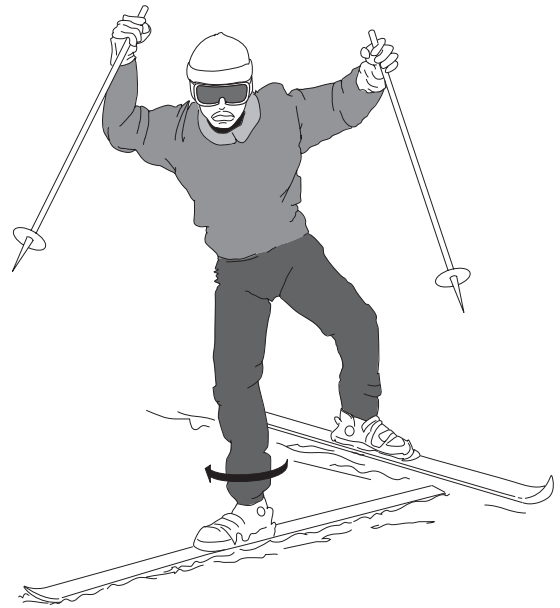
Fig. 24.6 Torsional loading. The skier's lower leg is torsionally loaded by the twisting action produced by a backward fall with the ski secured to the ground.
