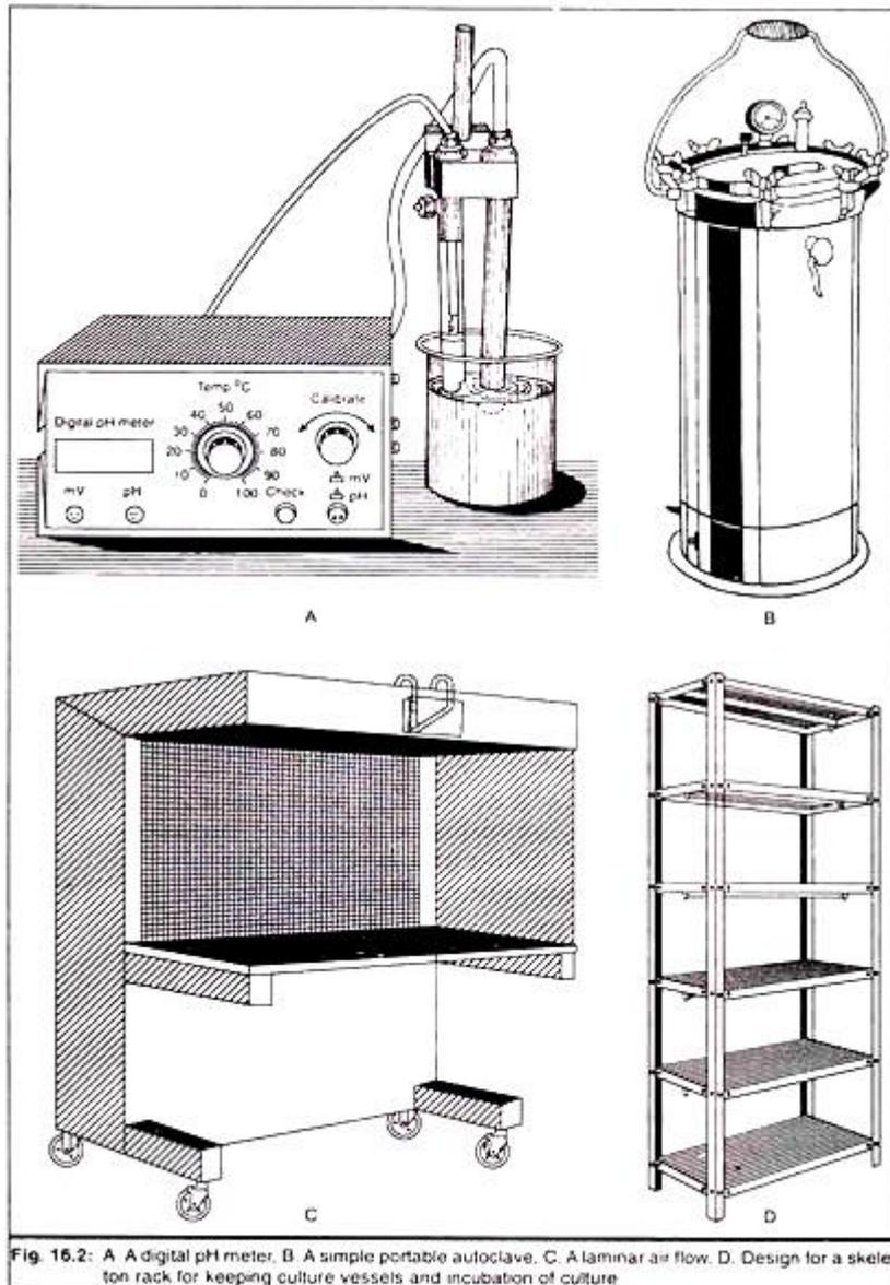
Fig. 16.2: A A digital pH meter, B A simple portable autoclave, C A laminar air flow, D. Design for a skeleton rack for keeping culture vessels and incubation of culture
