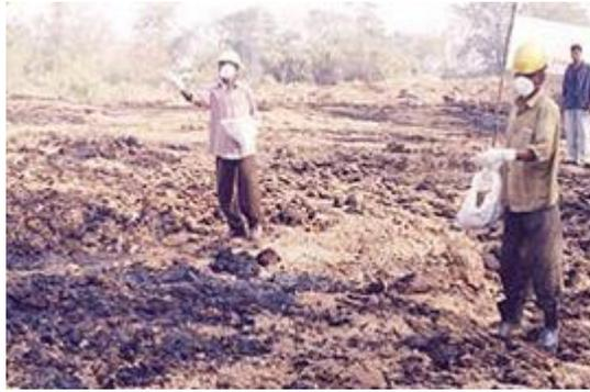
Application of Oilzapper on an oil-spill site in Assam
