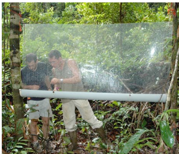
Photo 10: Single-vane window flight trap (French Guiana).
