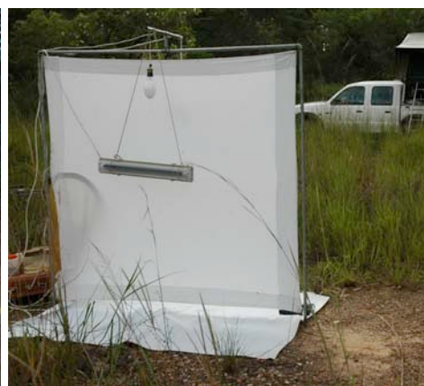
Photo 16: A light trap combining a mercury vapour bulb and a blacklight tube (Zambia).
