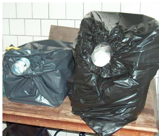
Photo 14: Emergence enclosure with collection receptacle (a plastic half-bottle).
