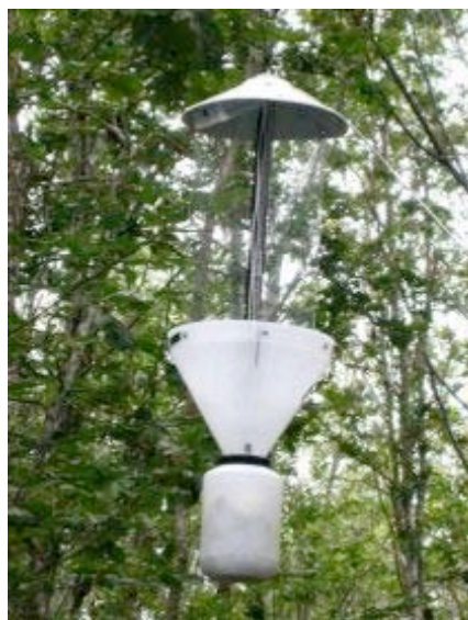
Photo 9: Automatically triggered light trap used in a comparative study of communities of nocturnal Lepidoptera (Bonneil, 2005).
