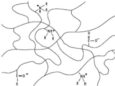
We have **immobilized pH gradient (IPGs)**. Here a gradient is incorporated covalently into a polyacrylamide gel at the time it is cast, using special buffers (one acidic and one basic, in different ratios along the gel).
