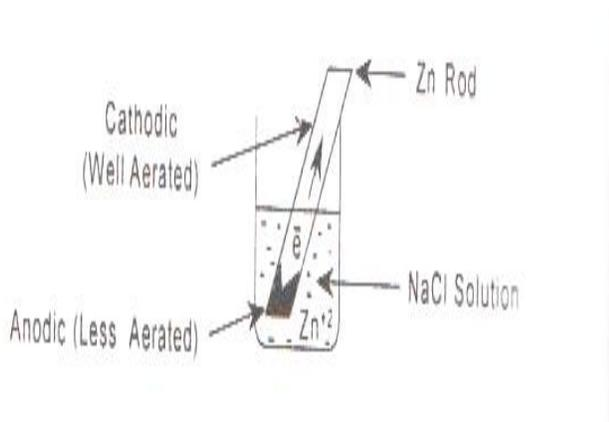
Fig.1.21Concen cell corrosion
