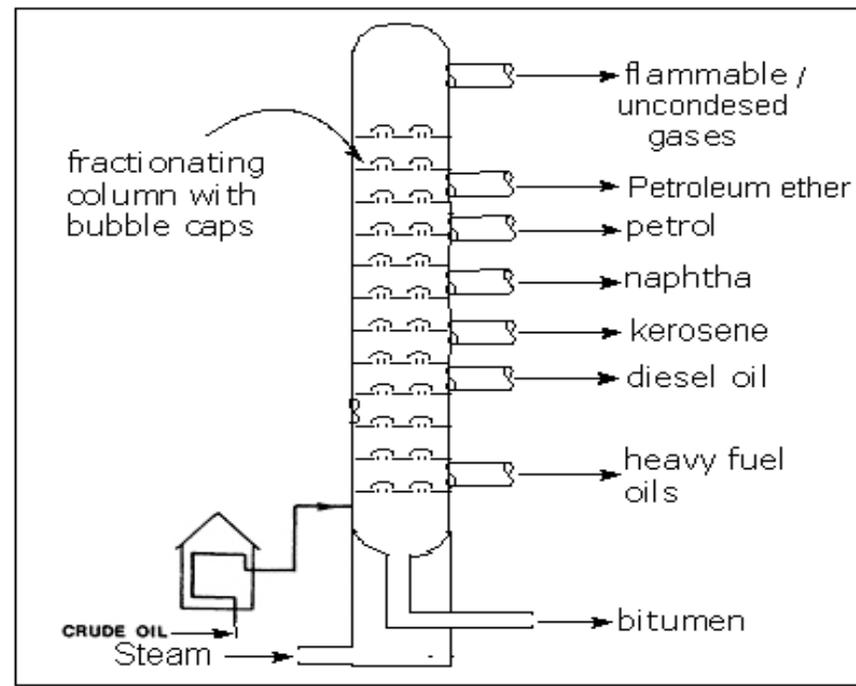
**Fig. 4.1 Refining of Petroleum**
