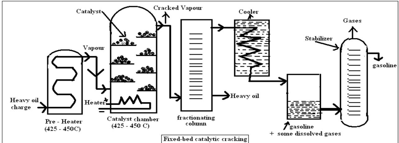
**Fig. 4.2 Fixed-Bed Catalytic Cracking**
