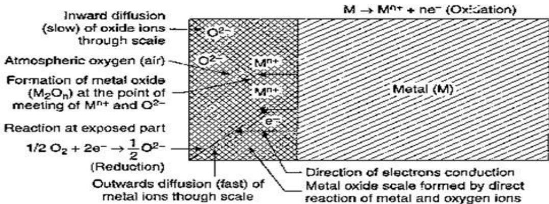
Fig.1.17 Oxidation corrosion
