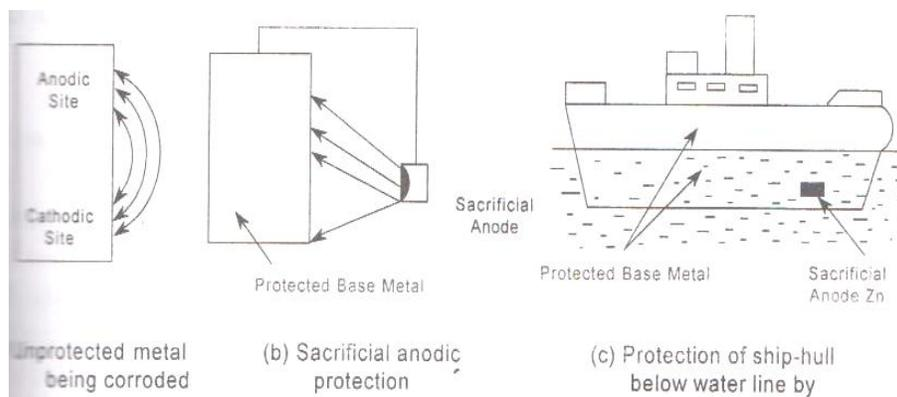
Fig.1.25 Sacrificial anode method: ship hull and underground water pipeline
