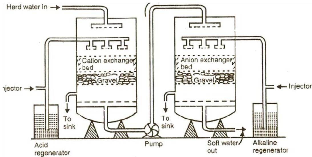
Fig3.6 Ion exchanger
