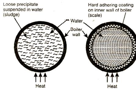
Fig3.2 Sludge Scale
