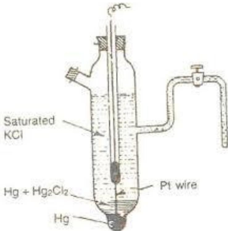
Fig1.11 Standard calomel electrode
