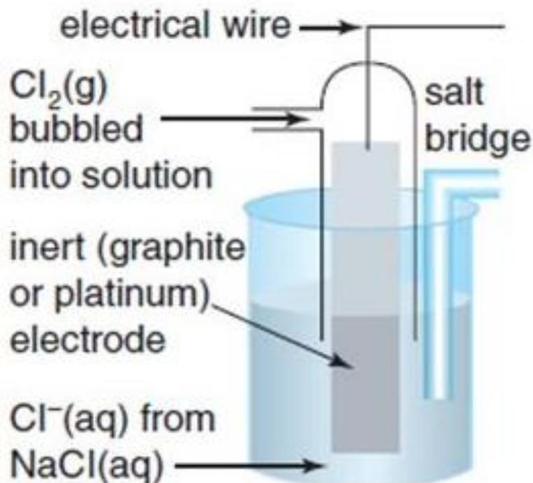
*Although gases are reactive, they are usually more difficult to manage in the laboratory. As a result, gaseous half-cells are not very common. In a gaseous half-cell, the gas bubbles over an inert electrode that is connected to the external wire. Its conjugate redox non-metal ion is in solution.*
