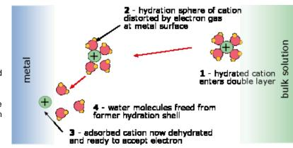
In the example of the Zn/Cu cell we have been using, the electrode reaction involves a metal and its hydrated cation; we call such electrodes *metal-metal ion* electrodes. There are a number of other kinds of electrodes which are widely encountered in electrochemistry and analytical chemistry.
