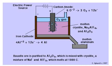
Fig. 26: Hall-Hérault cell for the production of aluminum
