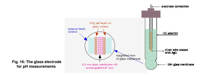
The potential of a glass electrode is given by a form of the Nernst equation very similar to that of an ordinary hydrogen electrode, but of course without the  $H_2$ :
