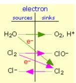
Fig. 9: Behavior of chlorine in water  $Cl_2$  can oxidize water (top) and also undergo disproportionation (bottom). In the latter process, one  $Cl_2$  molecule donates electrons to another.  $2H_2O + Cl_2 \rightarrow 2 Cl^- + O_2(g) + 4H^+$
