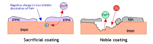
Fig. 23: Corrosion protection by sacrificial coating, and its reverse.
