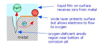
Fig. 22: Pitting corrosion netals are covered with thin lave
