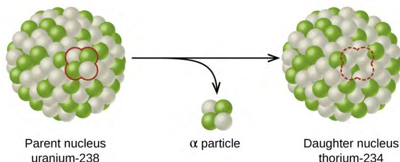
**Figure 21.5** A nucleus of uranium-238 (the parent nuclide) undergoes  $\alpha$  decay to form thorium-234 (the daughter nuclide). The alpha particle removes two protons (green) and two neutrons (gray) from the uranium-238 nucleus.
