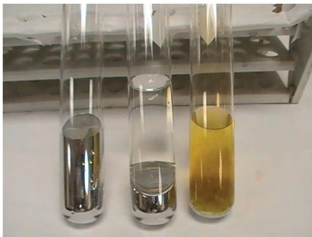
**Figure 18.8** From left to right: Hg(l), Hg + concentrated HCl, Hg + concentrated HNO<sub>3</sub>. (credit: Sahar Atwa)
