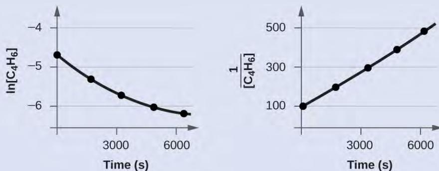
**Figure 12.11** These two graphs show first- and second-order plots for the dimerization of  $C_4H_6$ . Since the first-order plot (left) is not linear, we know that the reaction is not first order. The linear trend in the second-order plot (right) indicates that the reaction follows second-order kinetics.
