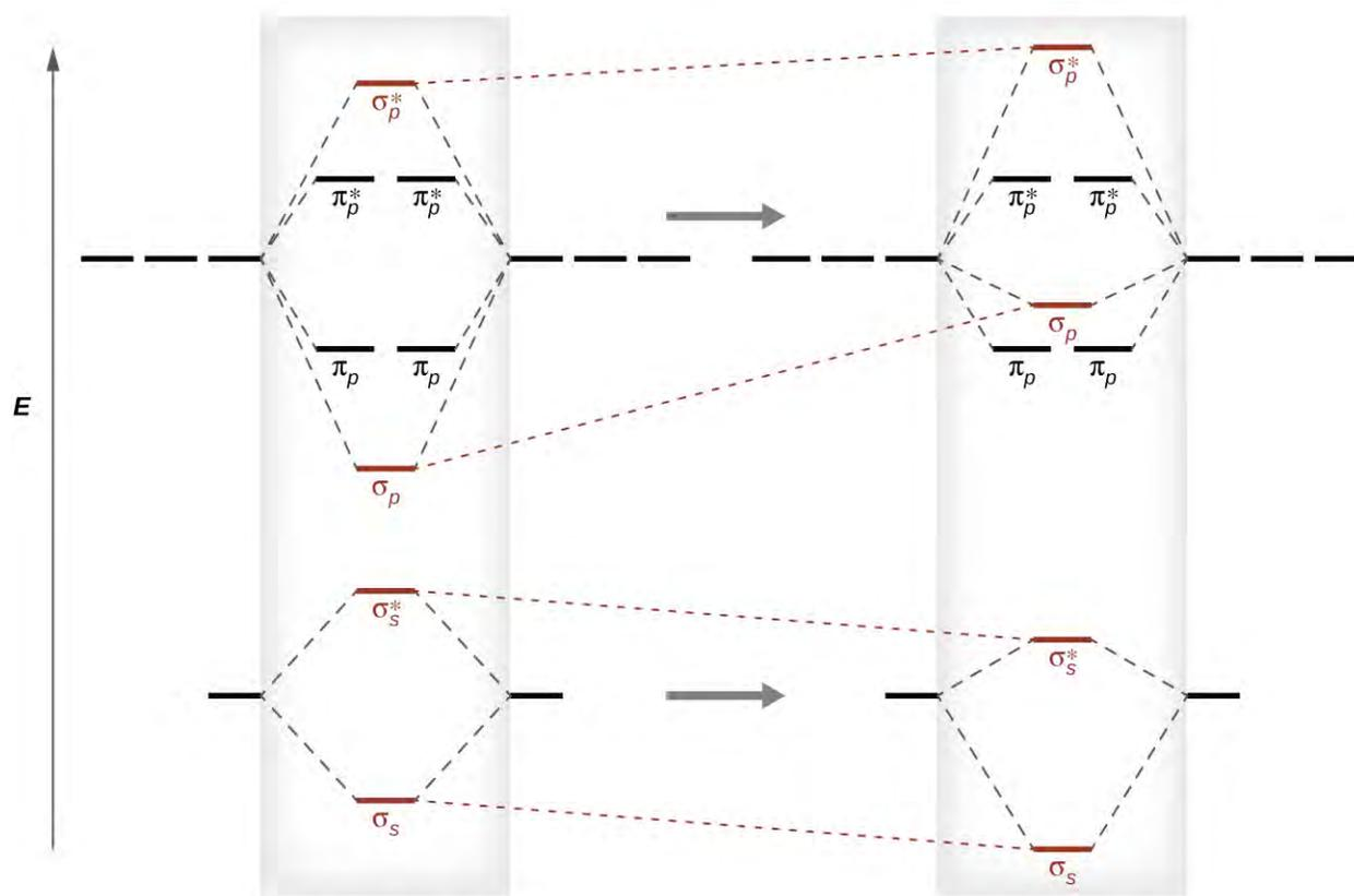
**Figure 8.38** Without mixing, the MO pattern occurs as expected, with the  $\sigma_p$  orbital lower in energy than the  $\pi_p$  orbitals. When s-p mixing occurs, the orbitals shift as shown, with the  $\sigma_p$  orbital higher in energy than the  $\pi_p$  orbitals.
