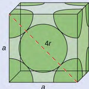
(a) In an FCC structure, Ca atoms contact each other across the diagonal of the face, so the length of the diagonal is equal to four Ca atomic radii ( $d = 4r$ ). Two adjacent edges and the diagonal of the face form a right triangle, with the length of each side equal to 558.8 pm and the length of the hypotenuse equal to four Ca atomic radii:
