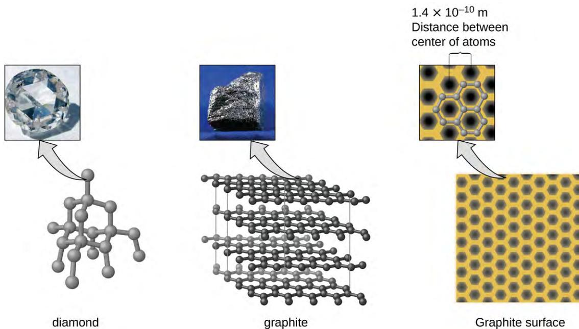
**Figure 10.43** Diamond is extremely hard because of the strong bonding between carbon atoms in all directions. Graphite (in pencil lead) rubs off onto paper due to the weak attractions between the carbon layers. An image of a graphite surface shows the distance between the centers of adjacent carbon atoms. (credit left photo: modification of work by Steve Jurvetson; credit middle photo: modification of work by United States Geological Survey)
