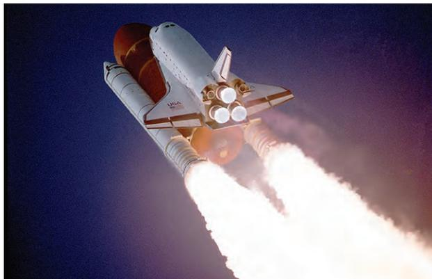
**Figure 18.28** Before the fleet's retirement in 2011, liquid hydrogen and liquid oxygen were used in the three main engines of a space shuttle. Two compartments in the large tank held these liquids until the shuttle was launched. (credit: "reynernmedia"/Flickr)
