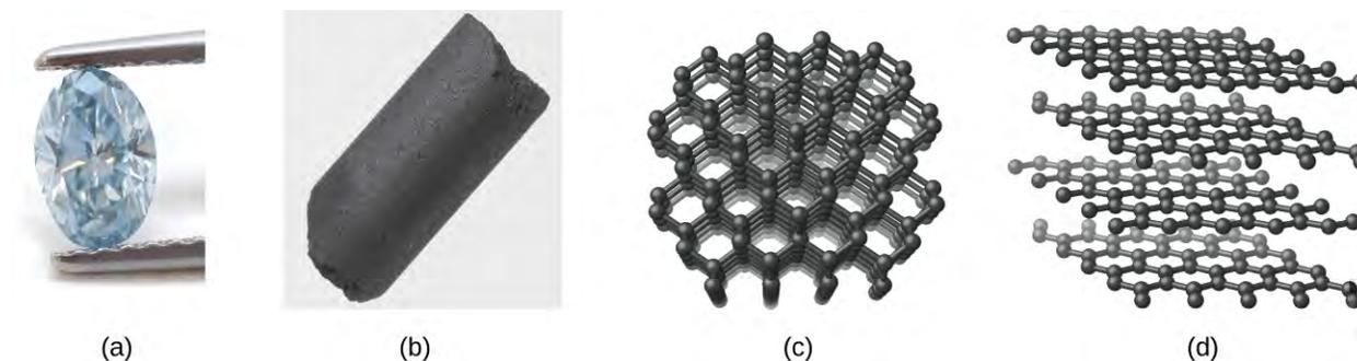
**Figure 18.20** (a) Diamond and (b) graphite are two forms of carbon. (c) In the crystal structure of diamond, the covalent bonds form three-dimensional tetrahedrons. (d) In the crystal structure of graphite, each planar layer is composed of six-membered rings. (credit a: modification of work by "Fancy Diamonds"/Flickr; credit b: modification of work from <http://images-of-elements.com/carbon.php>)
