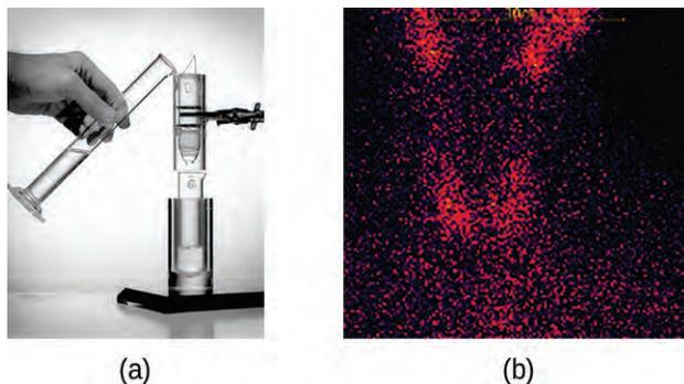
**Figure 21.25** (a) The first Tc-99m generator (circa 1958) is used to separate Tc-99 from Mo-99. The  $\text{MoO}_4^{2-}$  is retained by the matrix in the column, whereas the  $\text{TcO}_4^-$  passes through and is collected. (b) Tc-99 was used in this scan of the neck of a patient with Grave's disease. The scan shows the location of high concentrations of Tc-99. (credit a: modification of work by the Department of Energy; credit b: modification of work by "MBq"/Wikimedia Commons)
