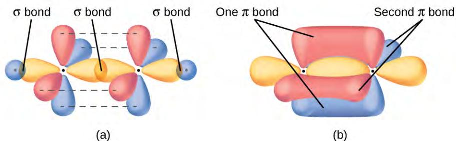
**Figure 8.25** (a) In the acetylene molecule,  $C_2H_2$ , there are two C–H  $\sigma$  bonds and a  $C \equiv C$  triple bond involving one C–C  $\sigma$  bond and two C–C  $\pi$  bonds. The dashed lines, each connecting two lobes, indicate the side-by-side overlap of the four unhybridized  $p$  orbitals. (b) This shows the overall outline of the bonds in  $C_2H_2$ . The two lobes of each of the  $\pi$  bonds are positioned across from each other around the line of the C–C  $\sigma$  bond.
