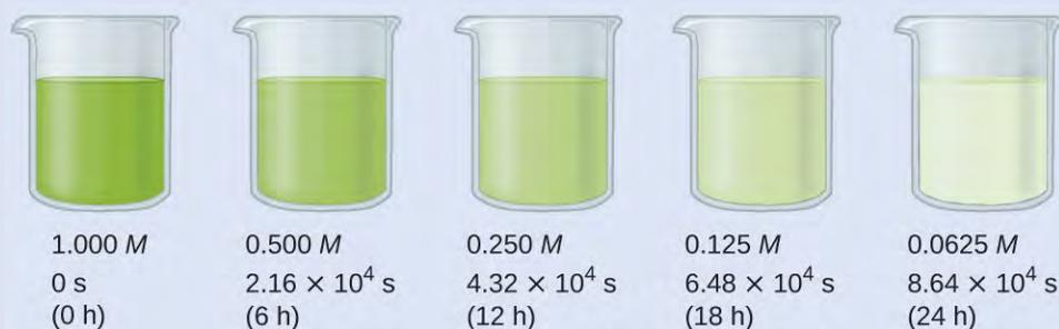
**Figure 12.13** The decomposition of  $\text{H}_2\text{O}_2$  ( $2\text{H}_2\text{O}_2 \rightarrow 2\text{H}_2\text{O} + \text{O}_2$ ) at  $40^\circ\text{C}$  is illustrated. The intensity of the color symbolizes the concentration of  $\text{H}_2\text{O}_2$  at the indicated times;  $\text{H}_2\text{O}_2$  is actually colorless.
