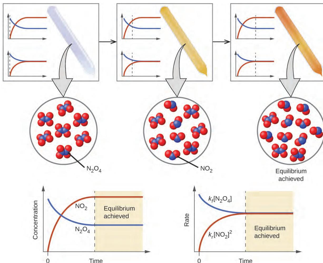
**Figure 13.2** A mixture of  $\text{NO}_2$  and  $\text{N}_2\text{O}_4$  moves toward equilibrium. Colorless  $\text{N}_2\text{O}_4$  reacts to form brown  $\text{NO}_2$ . As the reaction proceeds toward equilibrium, the color of the mixture darkens due to the increasing concentration of  $\text{NO}_2$ .
