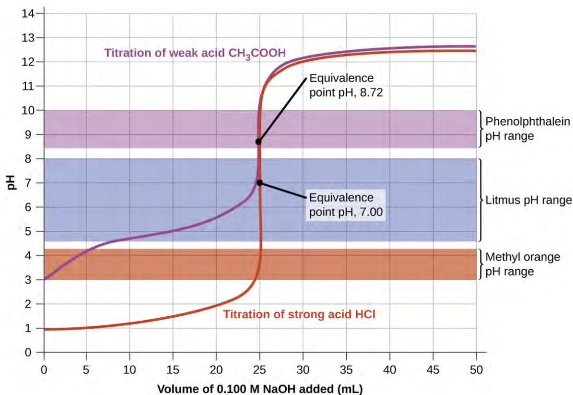
**Figure 14.23** The graph shows a titration curve for the titration of 25.00 mL of 0.100 M  $\text{CH}_3\text{CO}_2\text{H}$  (weak acid) with 0.100 M NaOH (strong base) and the titration curve for the titration of HCl (strong acid) with NaOH (strong base). The pH ranges for the color change of phenolphthalein, litmus, and methyl orange are indicated by the shaded areas.
