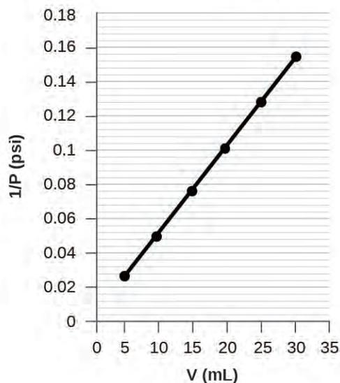
**Figure 9.13** When a gas occupies a smaller volume, it exerts a higher pressure; when it occupies a larger volume, it exerts a lower pressure (assuming the amount of gas and the temperature do not change). Since  $P$  and  $V$  are inversely proportional, a graph of  $\frac{1}{P}$  vs.  $V$  is linear.
