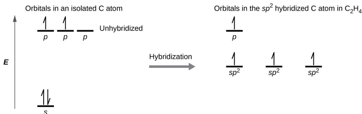
**Figure 8.22** In ethene, each carbon atom is  $sp^2$  hybridized, and the  $sp^2$  orbitals and the  $p$  orbital are singly occupied. The hybrid orbitals overlap to form  $\sigma$  bonds, while the  $p$  orbitals on each carbon atom overlap to form a  $\pi$  bond.
