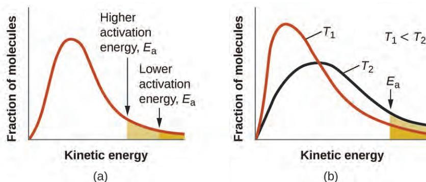
**Figure 12.17** (a) As the activation energy of a reaction decreases, the number of molecules with at least this much energy increases, as shown by the shaded areas. (b) At a higher temperature,  $T_2$ , more molecules have kinetic energies greater than  $E_a$ , as shown by the yellow shaded area.
