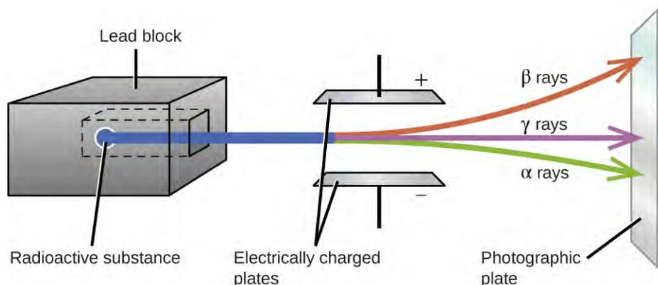
**Figure 21.6** Alpha particles, which are attracted to the negative plate and deflected by a relatively small amount, must be positively charged and relatively massive. Beta particles, which are attracted to the positive plate and deflected a relatively large amount, must be negatively charged and relatively light. Gamma rays, which are unaffected by the electric field, must be uncharged.
