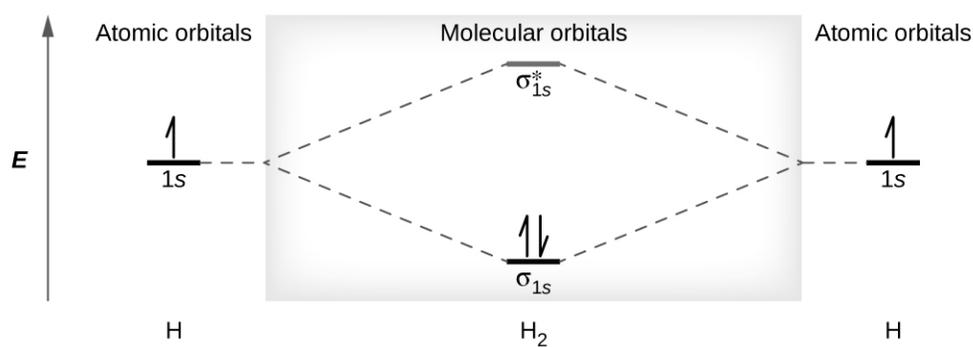
**Figure 8.35** The molecular orbital energy diagram predicts that  $H_2$  will be a stable molecule with lower energy than the separated atoms.
