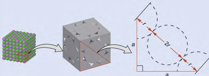
Drawing a right triangle on the face of the unit cell, we see that the length of the diagonal is equal to four chloride radii (one radius from each corner chloride and one diameter—which equals two radii—from the chloride ion in the center of the face), so  $d = 4r$ . From the Pythagorean theorem, we have:
