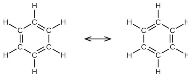
**Figure 8.26** Each carbon atom in benzene,  $C_6H_6$ , is  $sp^2$  hybridized, independently of which resonance form is considered. The electrons in the  $\pi$  bonds are not located in one set of  $p$  orbitals or the other, but rather delocalized throughout the molecule.
