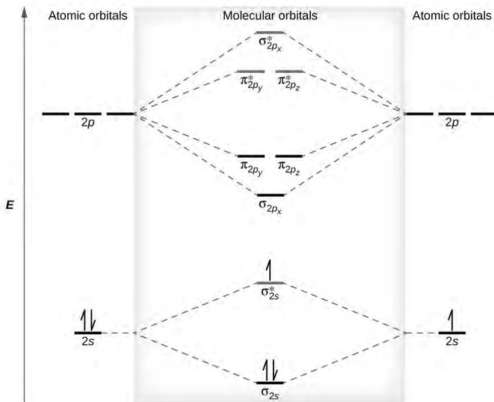
**Figure 8.34** This is the molecular orbital diagram for the homonuclear diatomic  $\text{Be}_2^+$ , showing the molecular orbitals of the valence shell only. The molecular orbitals are filled in the same manner as atomic orbitals, using the Aufbau principle and Hund's rule.
