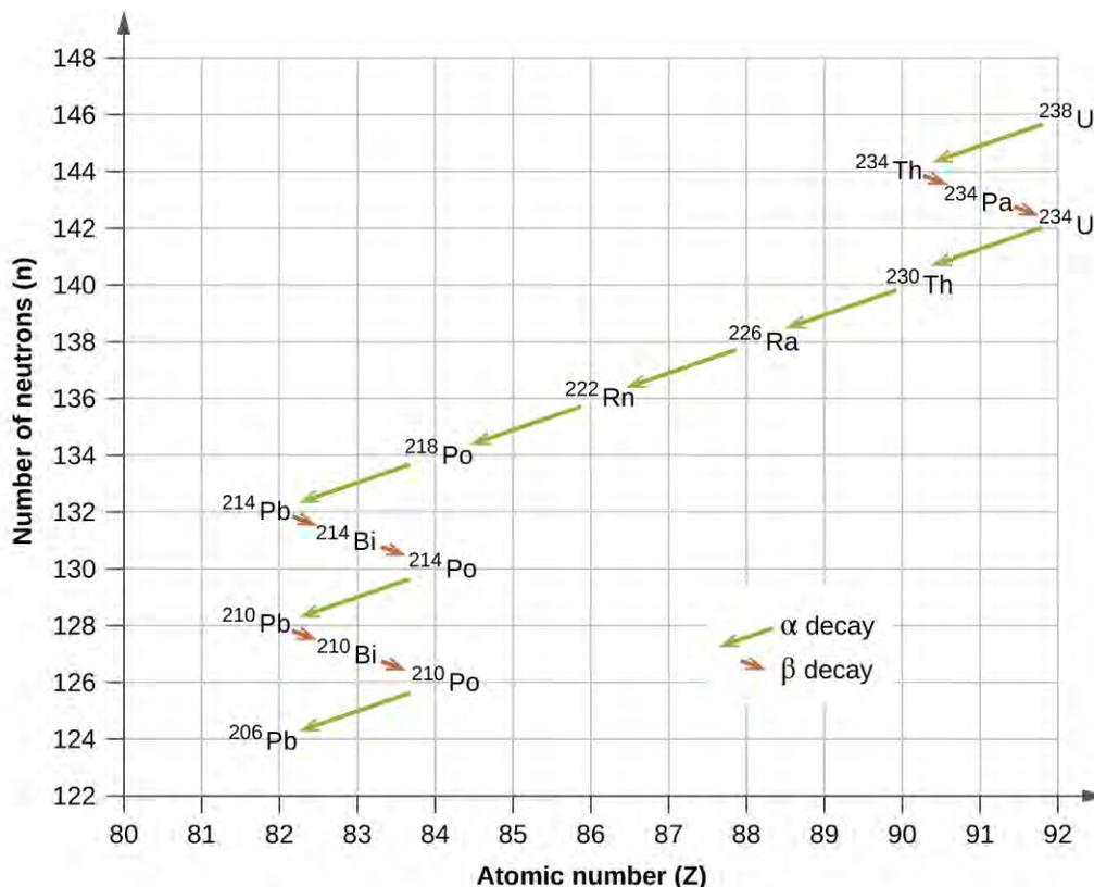
**Figure 21.9** Uranium-238 undergoes a radioactive decay series consisting of 14 separate steps before producing stable lead-206. This series consists of eight  $\alpha$  decays and six  $\beta$  decays.
