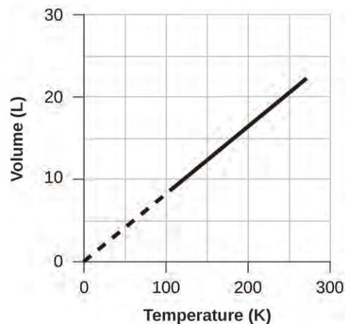
**Figure 9.12** The volume and temperature are linearly related for 1 mole of methane gas at a constant pressure of 1 atm. If the temperature is in kelvin, volume and temperature are directly proportional. The line stops at 111 K because methane liquefies at this temperature; when extrapolated, it intersects the graph's origin, representing a temperature of absolute zero.
