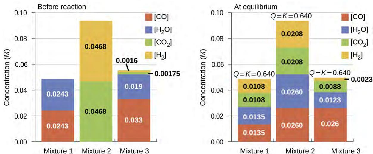
**Figure 13.7** Concentrations of three mixtures are shown before and after reaching equilibrium at 800 °C for the so-called water gas shift reaction:  $\text{CO}(g) + \text{H}_2\text{O}(g) \rightleftharpoons \text{CO}_2(g) + \text{H}_2(g)$ .
