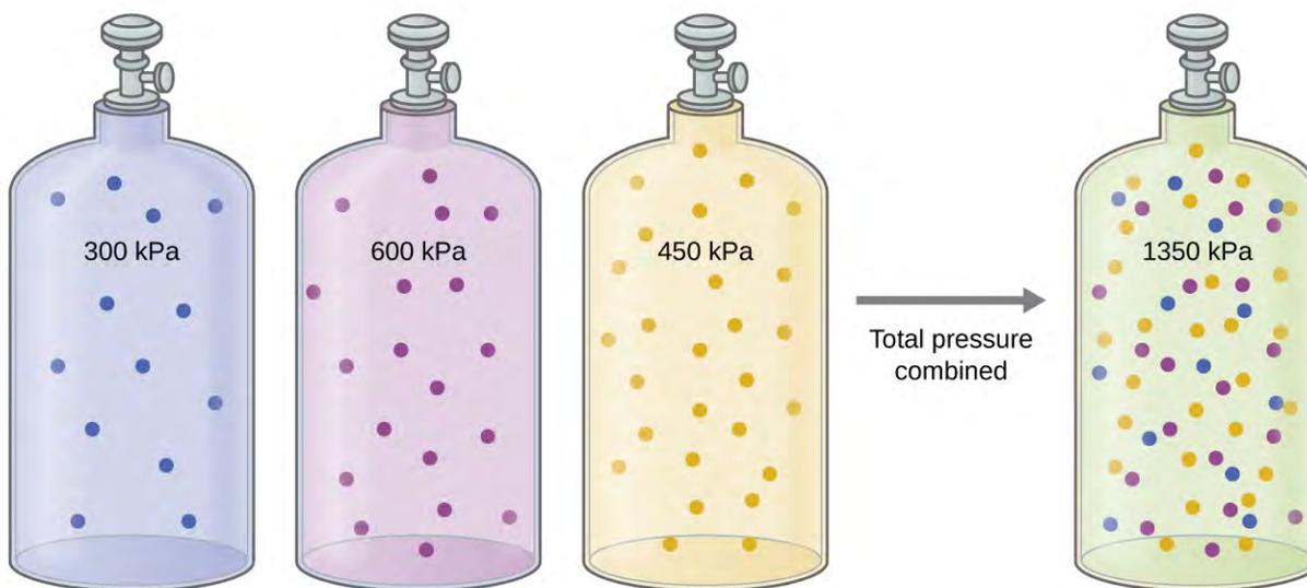
**Figure 9.20** If equal-volume cylinders containing gas A at a pressure of 300 kPa, gas B at a pressure of 600 kPa, and gas C at a pressure of 450 kPa are all combined in the same-size cylinder, the total pressure of the mixture is 1350 kPa.
