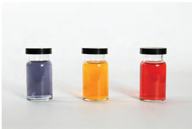
**Figure 19.38** The partially filled  $d$  orbitals of the stable ions  $\text{Cr}^{3+}(\text{aq})$ ,  $\text{Fe}^{3+}(\text{aq})$ , and  $\text{Co}^{2+}(\text{aq})$  (left, center and right, respectively) give rise to various colors. (credit: Sahar Atwa)
