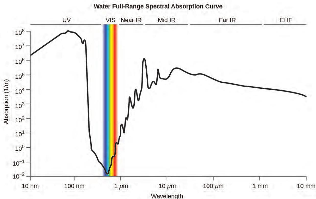
**Figure E1** Water full-range spectral absorption curve. This curve shows the full-range spectral absorption for water. The y-axis signifies the absorption in 1/cm. If we divide 1 by this value, we will obtain the length of the path (in cm) after which the intensity of a light beam passing through water decays by a factor of the base of the natural logarithm  $e$  ( $e = 2.718281828$ ).
