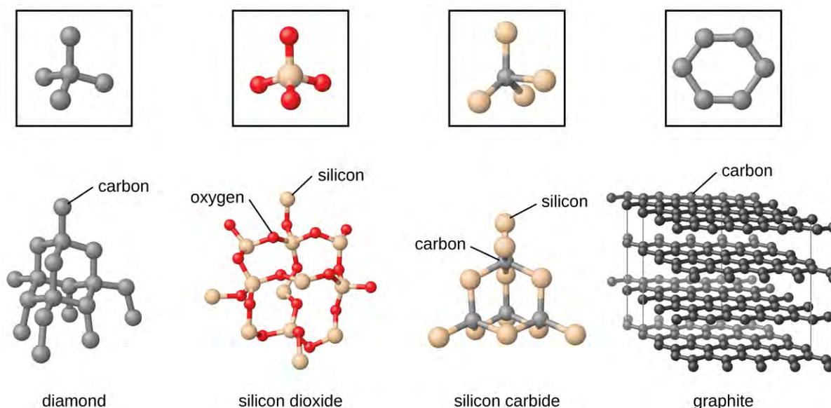
**Figure 10.41** A covalent crystal contains a three-dimensional network of covalent bonds, as illustrated by the structures of diamond, silicon dioxide, silicon carbide, and graphite. Graphite is an exceptional example, composed of planar sheets of covalent crystals that are held together in layers by noncovalent forces. Unlike typical covalent solids, graphite is very soft and electrically conductive.
