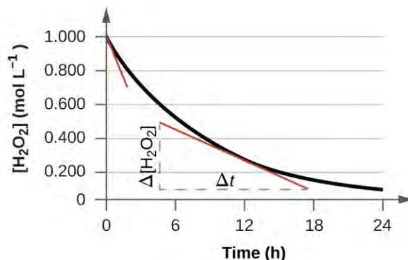
**Figure 12.3** This graph shows a plot of concentration versus time for a 1.000 M solution of  $\text{H}_2\text{O}_2$ . The rate at any instant is equal to the opposite of the slope of a line tangential to this curve at that time. Tangents are shown at  $t = 0$  h (“initial rate”) and at  $t = 10$  h (“instantaneous rate” at that particular time).
