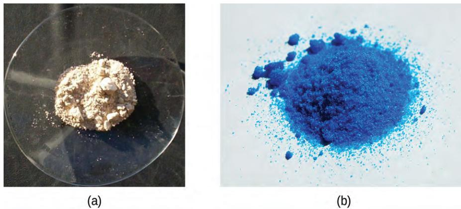
**Figure 19.40** (a) Copper(I) complexes with  $d^{10}$  configurations such as  $\text{CuI}$  tend to be colorless, whereas (b)  $d^9$  copper(II) complexes such as  $\text{Cu}(\text{NO}_3)_2 \cdot 5\text{H}_2\text{O}$  are brightly colored.
