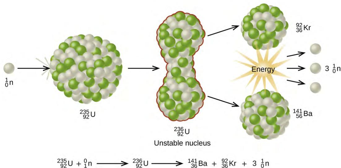
**Figure 21.14** When a slow neutron hits a fissionable U-235 nucleus, it is absorbed and forms an unstable U-236 nucleus. The U-236 nucleus then rapidly breaks apart into two smaller nuclei (in this case, Ba-141 and Kr-92) along with several neutrons (usually two or three), and releases a very large amount of energy.
