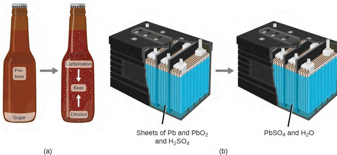
**Figure 1.8** (a) The mass of beer precursor materials is the same as the mass of beer produced: Sugar has become alcohol and carbonation. (b) The mass of the lead, lead oxide plates, and sulfuric acid that goes into the production of electricity is exactly equal to the mass of lead sulfate and water that is formed.
