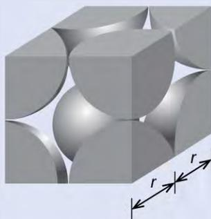
(a) Two adjacent Po atoms contact each other, so the edge length of this cell is equal to two Po atomic radii:
