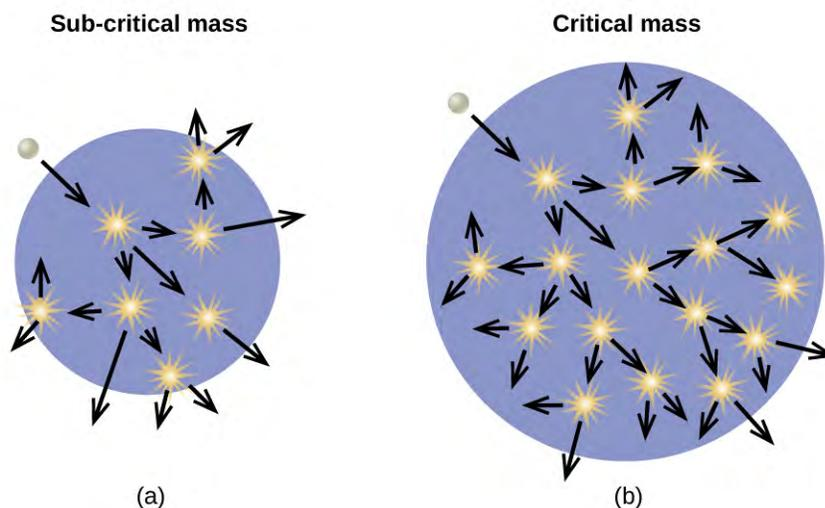
**Figure 21.17** (a) In a subcritical mass, the fissile material is too small and allows too many neutrons to escape the material, so a chain reaction does not occur. (b) In a critical mass, a large enough number of neutrons in the fissile material induce fission to create a chain reaction.
