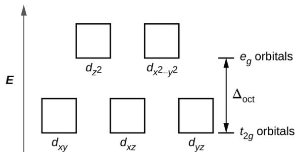
**Figure 19.34** In octahedral complexes, the  $e_g$  orbitals are destabilized (higher in energy) compared to the  $t_{2g}$  orbitals because the ligands interact more strongly with the  $d$  orbitals at which they are pointed directly.
