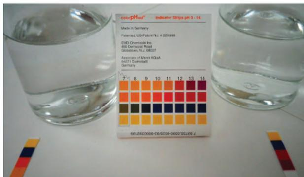
**Figure 14.10** pH paper indicates that a 0.1- $M$  solution of  $\text{NH}_3$  (left) is weakly basic. The solution has a pOH of 3 ( $[\text{OH}^-] = 0.001 M$ ) because the weak base  $\text{NH}_3$  only partially reacts with water. A 0.1- $M$  solution of  $\text{NaOH}$  (right) has a pOH of 1 because  $\text{NaOH}$  is a strong base. (credit: modification of work by Sahar Atwa)
