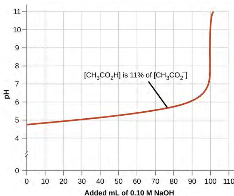
**Figure 14.20** The graph, an illustration of buffering action, shows change of pH as an increasing amount of a 0.10-M NaOH solution is added to 100 mL of a buffer solution in which, initially,  $[\text{CH}_3\text{CO}_2\text{H}] = 0.10\text{ M}$  and  $[\text{CH}_3\text{CO}_2^-] = 0.10\text{ M}$ .
