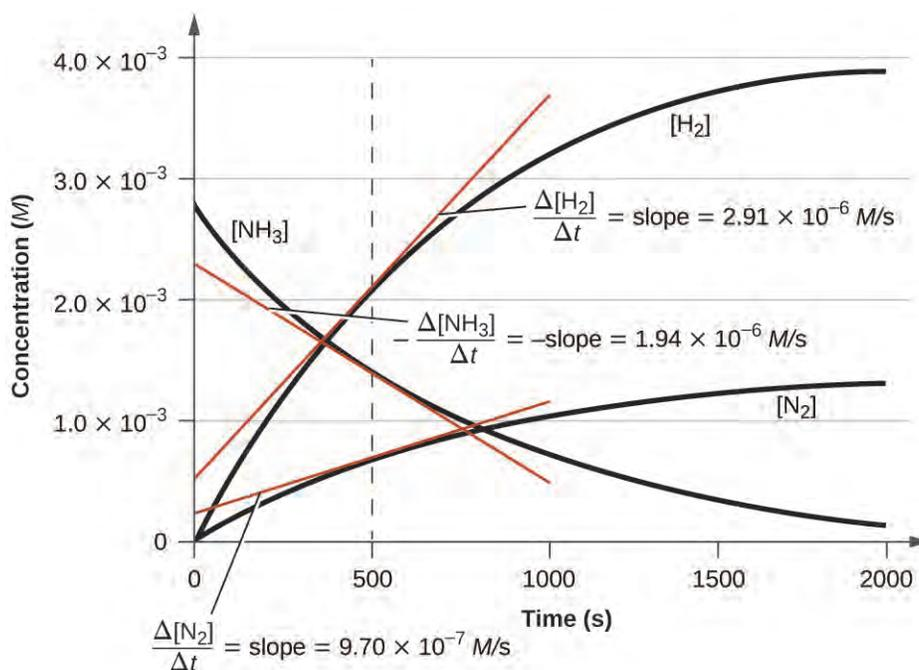
**Figure 12.5** This graph shows the changes in concentrations of the reactants and products during the reaction  $2\text{NH}_3 \rightarrow 3\text{N}_2 + \text{H}_2$ . The rates of change of the three concentrations are related by their stoichiometric factors, as shown by the different slopes of the tangents at  $t = 500$  s.
