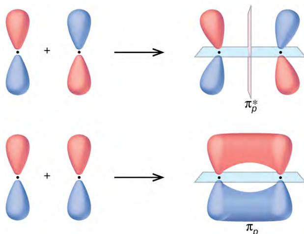
**Figure 8.31** Side-by-side overlap of each two  $p$  orbitals results in the formation of two  $\pi$  molecular orbitals. Combining the out-of-phase orbitals results in an antibonding molecular orbital with two nodes. One contains the axis, and one contains the perpendicular. Combining the in-phase orbitals results in a bonding orbital. There is a node (blue line) directly along the internuclear axis, but the orbital is located between the nuclei (red dots) above and below this node.
