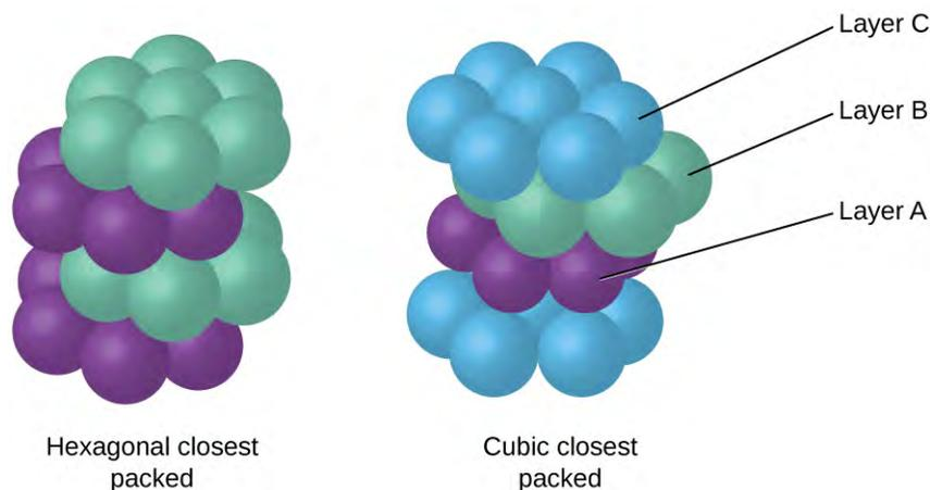
**Figure 10.54** In both types of closest packing, atoms are packed as compactly as possible. Hexagonal closest packing consists of two alternating layers (ABABAB...). Cubic closest packing consists of three alternating layers (ABCABCABC...).
