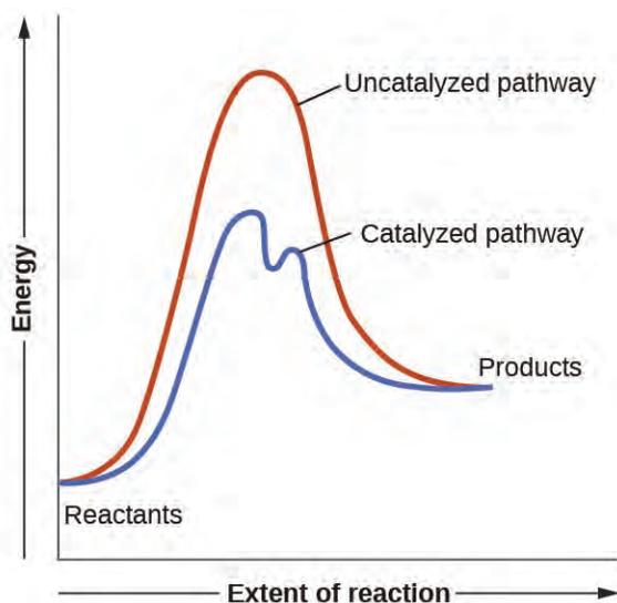
**Figure 12.22** This potential energy diagram shows the effect of a catalyst on the activation energy. The catalyst provides a different reaction path with a lower activation energy. As shown, the catalyzed pathway involves a two-step mechanism (note the presence of two transition states) and an intermediate species (represented by the valley between the two transitions states).
