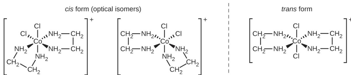
**Figure 19.24** Three isomeric forms of  $[Co(en)_2Cl_2]^+$  exist. The *trans* isomer, formed when the chlorines are positioned at a  $180^\circ$  angle, has very different properties from the *cis* isomers. The mirror images of the *cis* isomer form a pair of optical isomers, which have identical behavior except when reacting with other enantiomers.
