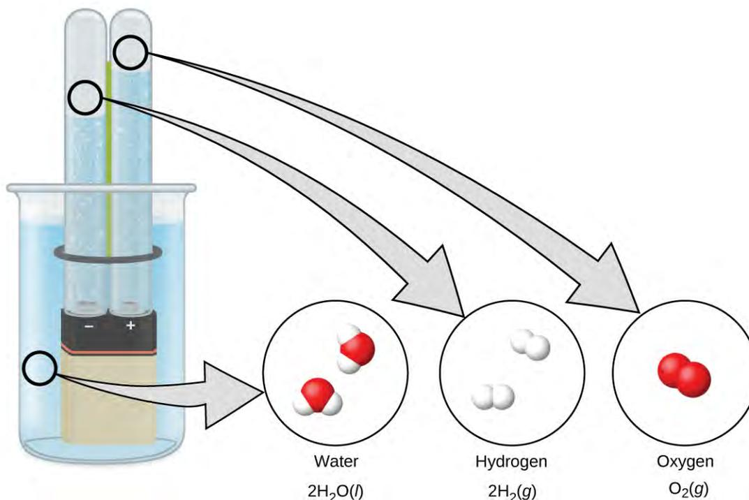
**Figure 1.15** The decomposition of water is shown at the macroscopic, microscopic, and symbolic levels. The battery provides an electric current (microscopic) that decomposes water. At the macroscopic level, the liquid separates into the gases hydrogen (on the left) and oxygen (on the right). Symbolically, this change is presented by showing how liquid  $\text{H}_2\text{O}$  separates into  $\text{H}_2$  and  $\text{O}_2$  gases.
