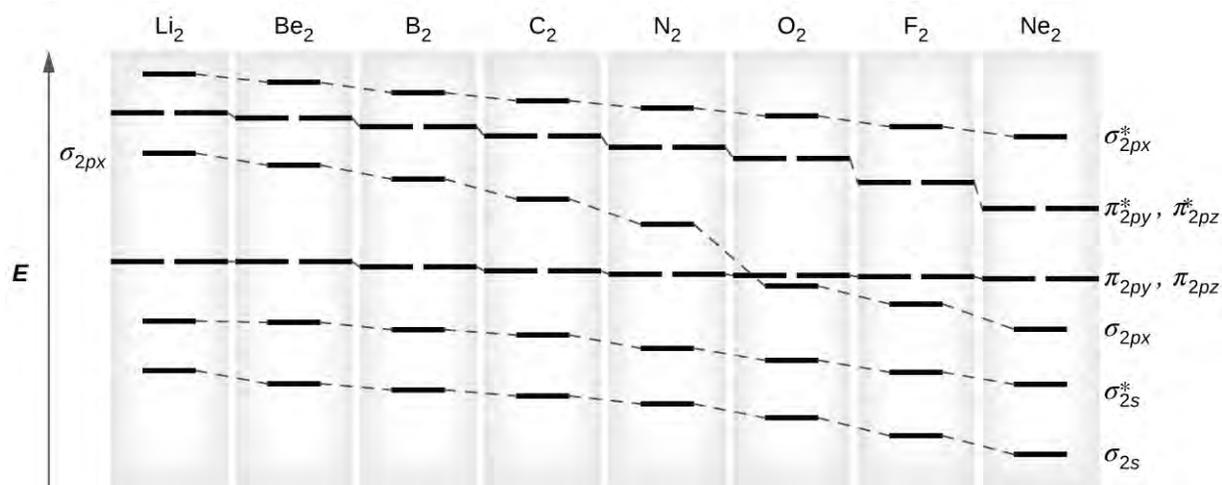
**Figure 8.37** This shows the MO diagrams for each homonuclear diatomic molecule in the second period. The orbital energies decrease across the period as the effective nuclear charge increases and atomic radius decreases. Between  $N_2$  and  $O_2$ , the order of the orbitals changes.
