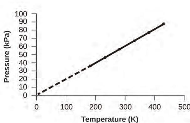
**Figure 9.11** For a constant volume and amount of air, the pressure and temperature are directly proportional, provided the temperature is in kelvin. (Measurements cannot be made at lower temperatures because of the condensation of the gas.) When this line is extrapolated to lower pressures, it reaches a pressure of 0 at  $-273\text{ }^{\circ}\text{C}$ , which is 0 on the kelvin scale and the lowest possible temperature, called absolute zero.
