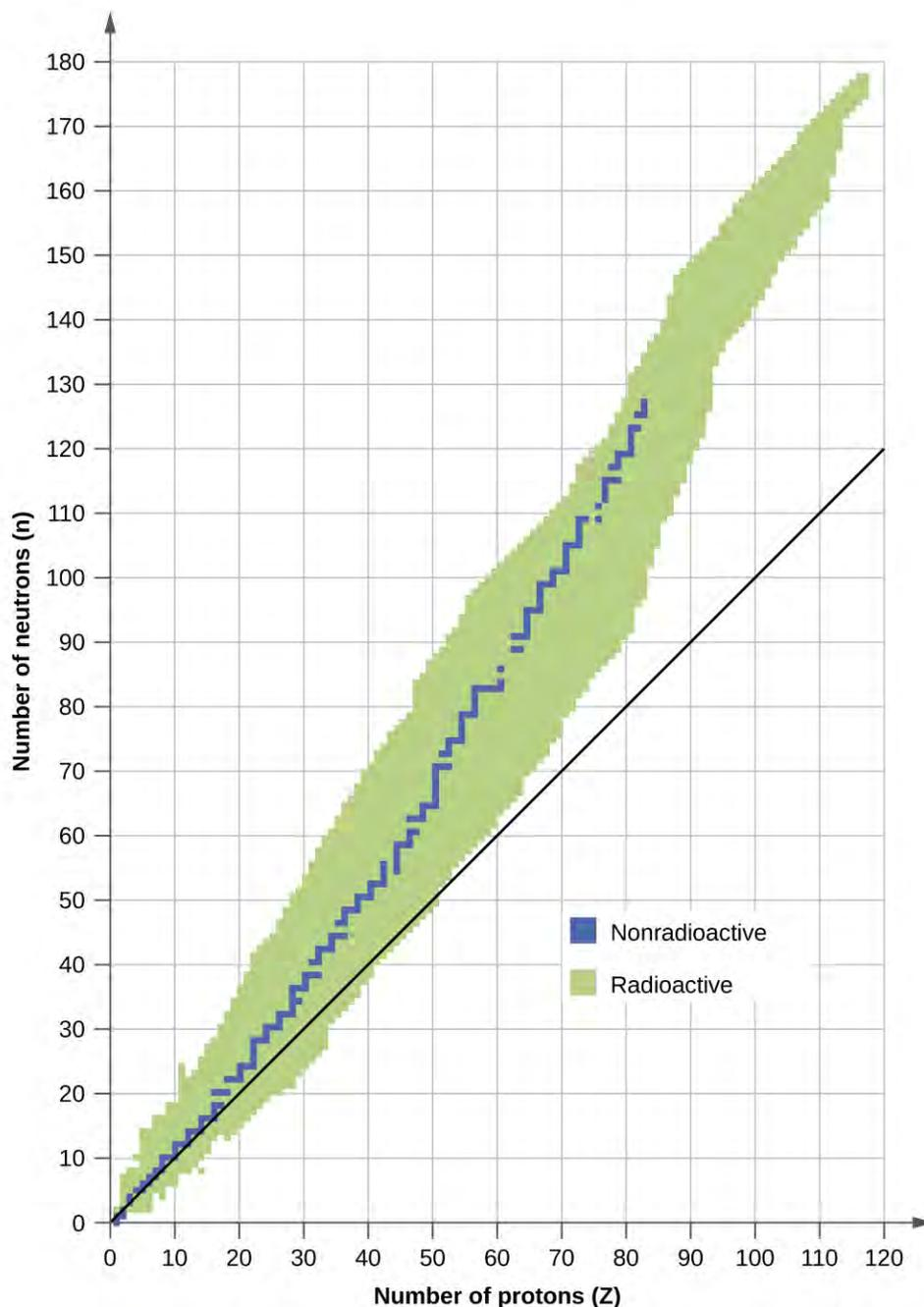
**Figure 21.2** This plot shows the nuclides that are known to exist and those that are stable. The stable nuclides are indicated in blue, and the unstable nuclides are indicated in green. Note that all isotopes of elements with atomic numbers greater than 83 are unstable. The solid line is the line where  $n = Z$ .
