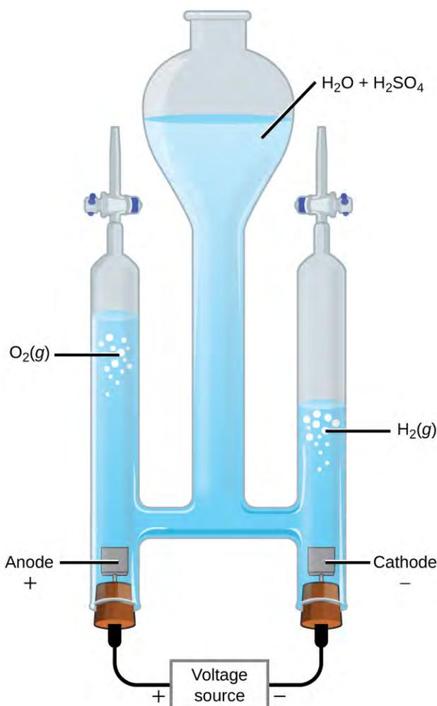
**Figure 17.20** Water decomposes into oxygen and hydrogen gas during electrolysis. Sulfuric acid was added to increase the concentration of hydrogen ions and the total number of ions in solution, but does not take part in the reaction. The volume of hydrogen gas collected is twice the volume of oxygen gas collected, due to the stoichiometry of the reaction.
