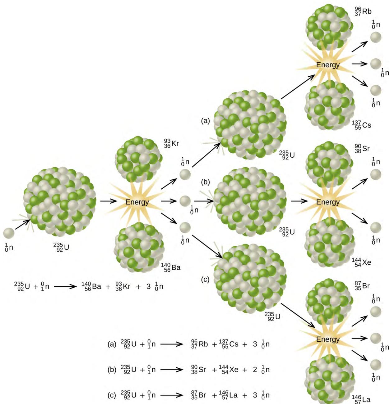
**Figure 21.16** The fission of a large nucleus, such as U-235, produces two or three neutrons, each of which is capable of causing fission of another nucleus by the reactions shown. If this process continues, a nuclear chain reaction occurs.
