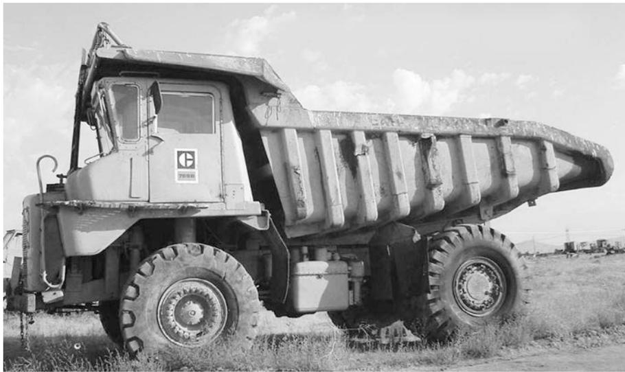
Figure 5.27: 40 ton Rear Dump Truck
