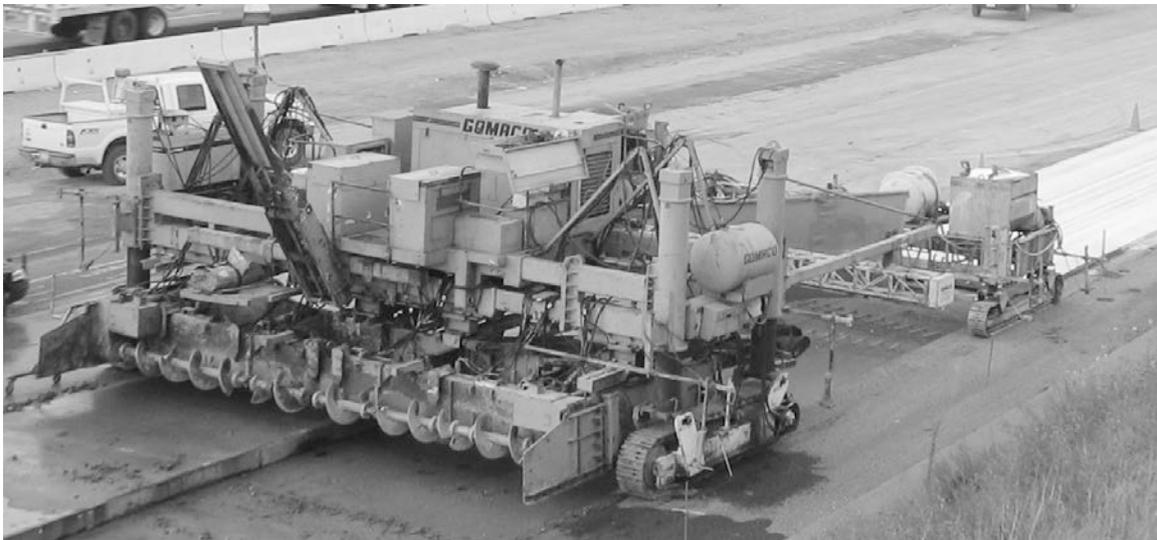
Figure 5.35: Large Grade Trimmer/Reclaimer/Paver
