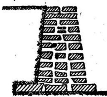
2. **Ashlar Masonry:** This type of masonry is built from accurately dressed stones with uniform and fine joints of about 3mm thickness by arranging the stone blocks in various patterns. The backing of ashlar masonry walls may be built of ashlar masonry or rubble masonry. The size of stones blocks should be in proportion to wall thickness. The various types of masonry can be classified under the following categories .
