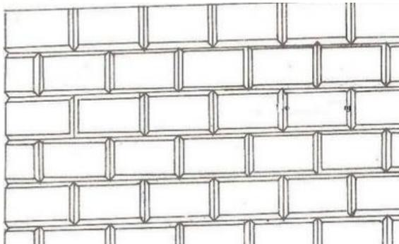
(v) **Ashlar block-in-course masonry:** This type of ashlar masonry occupies an intermediate position between the rubble masonry and the ashlar masonry. The faces of the stones are generally hammer-dressed and thickness of mortar joints does not exceed 6mm. The depth of courses varies from 200mm to 300mm. This type of construction is used for heavy engineering works such as retaining walls, sea walls bridges, public buildings etc.
