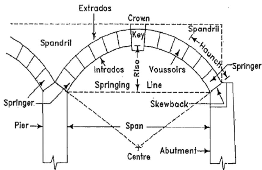
Abutment :This is the end support of an arch.
