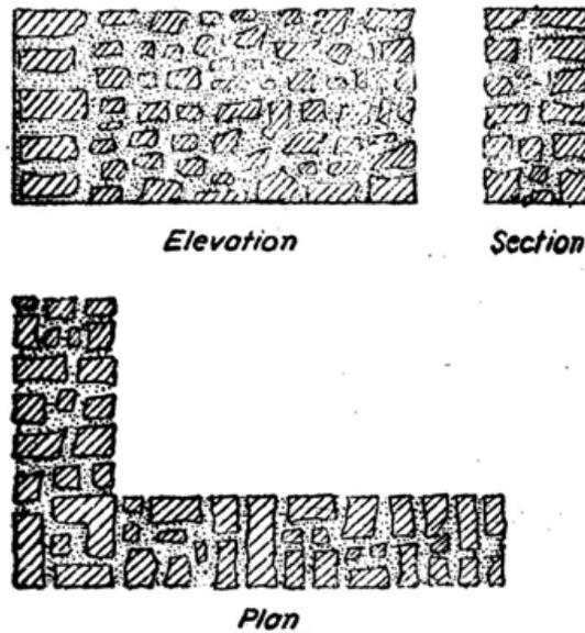
(iii)**Coursed squared rubble:** This type of masonry is made up of hammer squared stones facing with bonded backing of uncoursed random rubble masonry. The stones employed in each course are of equal height. The backing and facing construction, should be carried simultaneously. In order to avoid thick mortar joints, small chips may be used as shown in the fig
