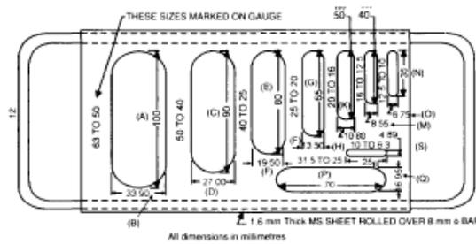
Fig. 6.4 Thickness Gauge
