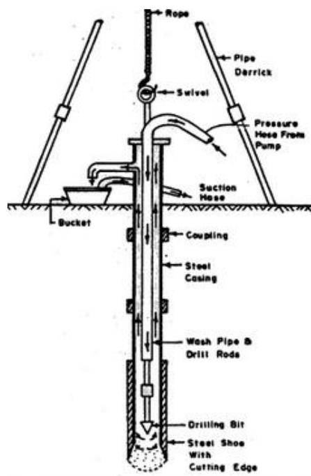
(c) Rotary boring: is a very fast method of advancing hole in both rocks and soils. A drill bit, fixed to the lower end of the drill rods, is rotated by a suitable chuck and is always kept in firm contact with the bottom of the hole. A drilling mud usually a water solution of bentonite with or without other admixtures is continuously forced down to the hollow drill rods. The mud returning upwards brings the cuttings to the surface.
