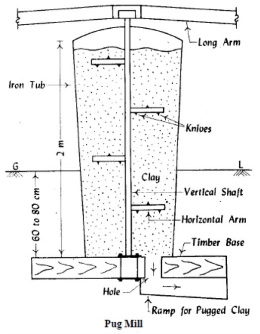
**Process:-** Clay with water is placed in pug mill from the top. When the vertical staff is rotated by using electric pair, steam or diesel or turned by pair of bullocks. Clay is thoroughly mixed up by the actions of horizontal arms and knives when clay has been sufficiently pugged, hole at the bottom of tub, is opened cut and the pugged earth is taken out from ramp for the next operation of moulding.
