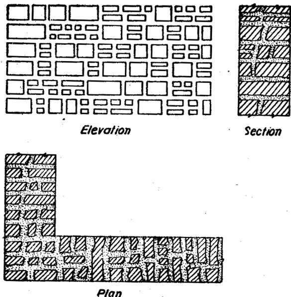
(iv)**Built to regular course:** In this type of stone masonry the uniform height stones are used in horizontal layers not less than 13cm in height. Generally, the stone beds are hammered or chisel dressed to a depth of atleast 10cm from the face. The stones are arranged in such a manner so that the vertical joints of two consecutive course do not coincide with each other as shown in fig
