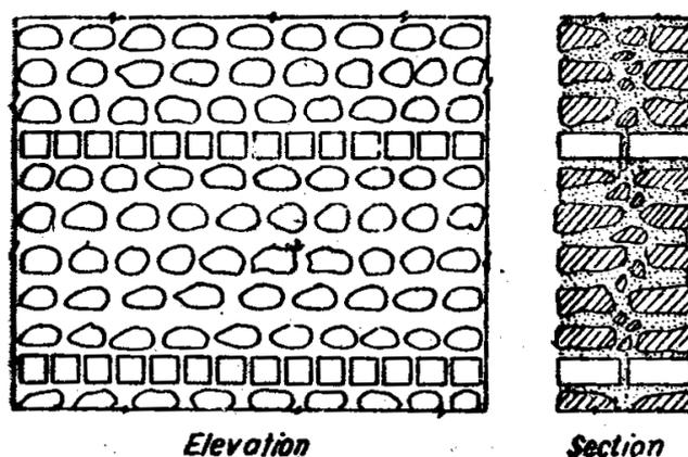
(vii) **Dry rubble masonry:** This type of masonry is used in the construction of retaining walls pitching earthen dams and canal slopes in the form of random rubble masonry without any mortar. The hallow spaces left around stones should be tightly packed with smaller stone pieces as shown in fig.
