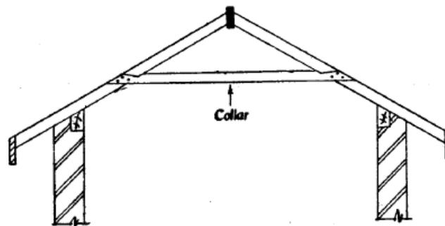
Fig 13.6 Collar beam roof
