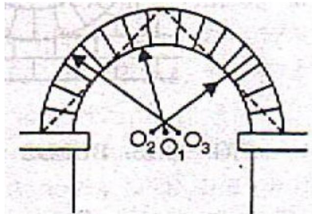
**8.Relieving Arch:** This arch is constructed either on a flat arch on a wooden lintel to provide greater strength. The ends of relieving arch should be carried sufficiently into the abutments. The relieving arch makes it possible to replace the decayed lintel later, without disturbing the stability of the structure.
