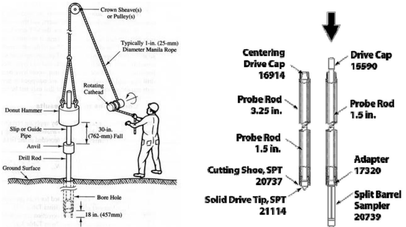
(iii) **Sub-surface sounding (SPT Test):** In this method, the resistance of the soil with depth is measured by means of a tool known as penetrometer under static or dynamic loading.
