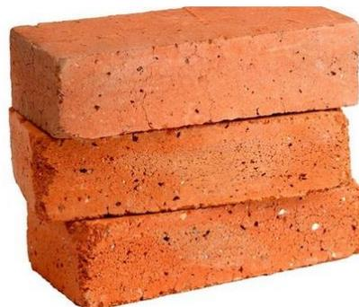
b. **Second class bricks:** These bricks are ground moulded and they are burnt in kilns. The surface of the bricks is somewhat rough and the shape is also slightly irregular. These bricks are commonly used at places where brick work is to be provided with a coat of plaster.
