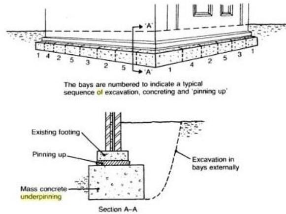
**Fig.1: Mass Concrete Underpinning**
