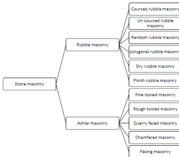
Depending upon the arrangement of stones in the construction, degree of refinement used in shaping the stone and finishing adopted, stone masonry can be classified as follows:
