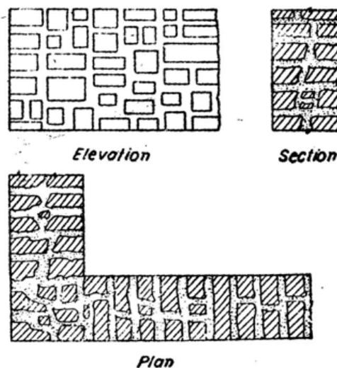
(ii) **Coursed random rubble:** This type of masonry is commonly used in the construction of low height walls of public buildings, residential buildings, abutment and piers of ordinary bridges. The stones of 5 to 20cm size are used in each course as shown in fig.
