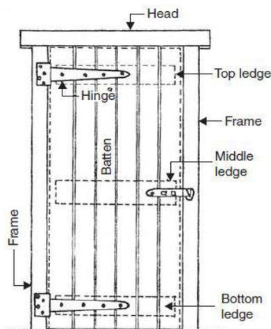
Fig. 8.21. Batted and ledged door
