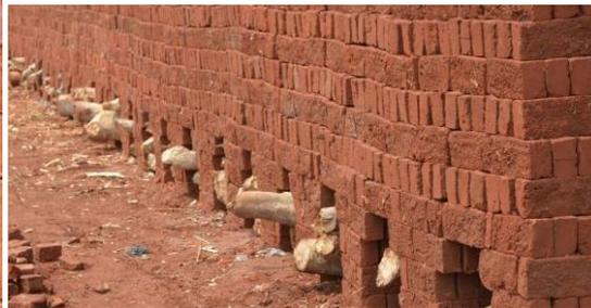
a. **First Class bricks:** These bricks are table moulded and of standard shape. The surface and edges of the bricks are sharp, square, smooth and straight. They comply with all the qualities of good bricks and are used for superior work of permanent nature.
