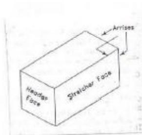
6. **Header:** it is the shorter face of the brick (11.4cm X 7.6cm) as seen in the elevation of the wall. A course of bricks in which all the bricks are laid as headers on facing is known as header course.
