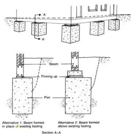
**Fig.3: Pier and Beam Underpinning Method**
