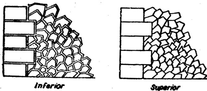
(vi) **Plint rubble masonry:** This type of masonry is used in the areas where the flint is available in plenty. The flint stones varying in thickness from 8 to 15cm and in length from 15 to 30cm are arranged in the facing in the form of coursed or uncoursed masonry as shown in fig
