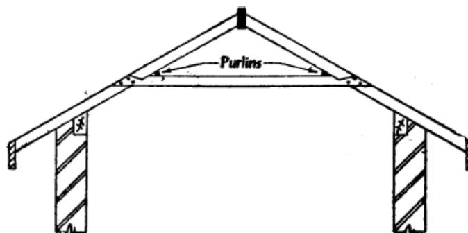
Fig 13.7 Double or Purlin roof
