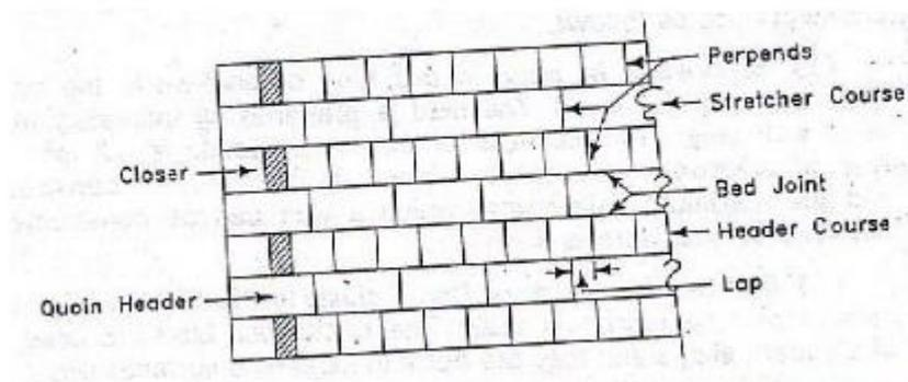
9. **Perpend:** It is a imaginary vertical line which includes the vertical joint separating two adjoining bricks.
