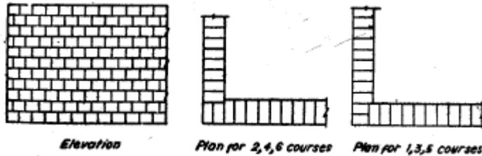
**Stretcher bond:** In this type of bond all the bricks are laid with their lengths in the direction of the wall. This pattern is used only for wall having thickness of 9cm only as shown in fig .
