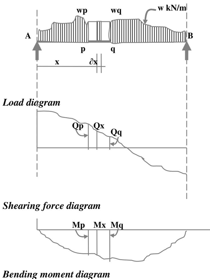
Figure 2. 10 variable load, shearing force and bending moment for a beam
