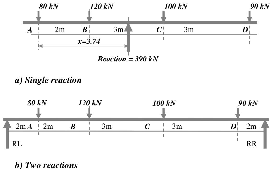
**Figure 2. 8 Beam reaction to parallel forces**
