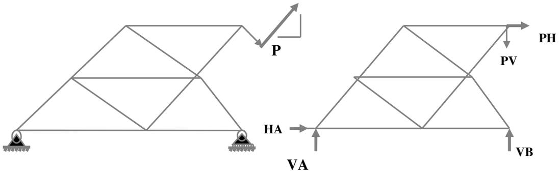
**Body ( a pin jointed structure**
