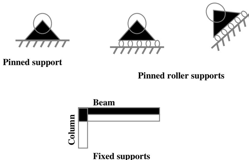
**Figure 2. 4 Different types of supports**
