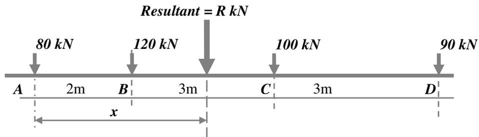
**Figure 2. 7 Addition of parallel forces**
