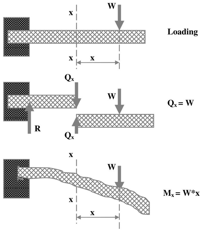
**Figure 2.9** Development of shearing force and bending moment in a cantilever beam
