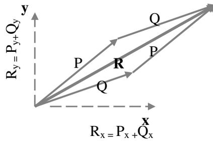
In the figure the forces P and Q are added to get one force R in magnitude and direction which can be obtained graphically. The vector components of R are the addition of vector components of Q and P. in the use of parallelogram rule the addition of the forces is interchangeable i.e.  $P+Q = Q+P$  .
