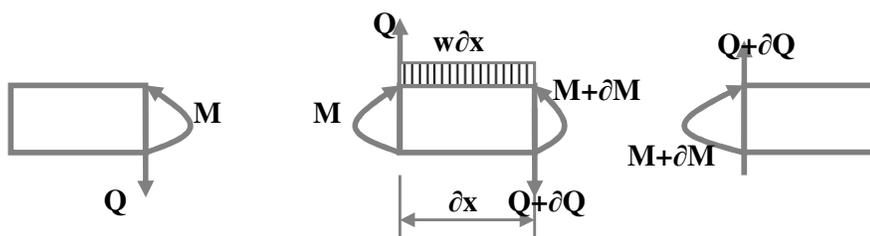
**Figure 2. 11 Element within a beam**
