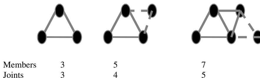
**Figure 2. 5** Statically determinate pin jointed frameworks
