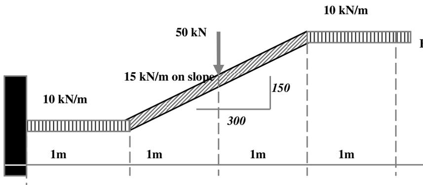
ii) Fixed on one side staircase (cantilevering)
