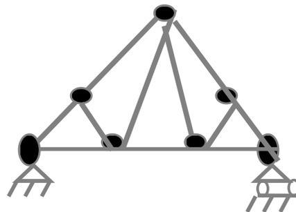
Roller allows movement therefore this support is not rigid
