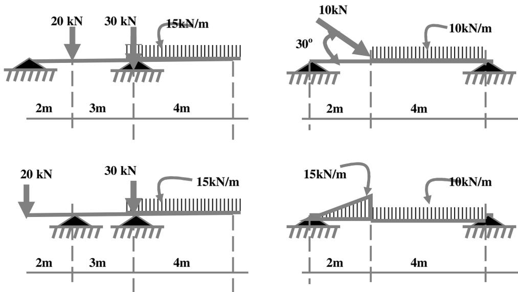
5) Calculate the reaction and its direction for the two staircase sections shown below
