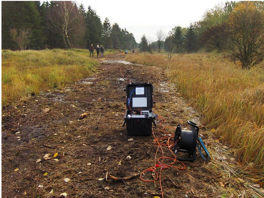
Figure 6.5: Electrical resistivity surveying.
