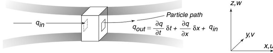
Figure 7.3 Sketch of flow used for deriving the total derivative.
