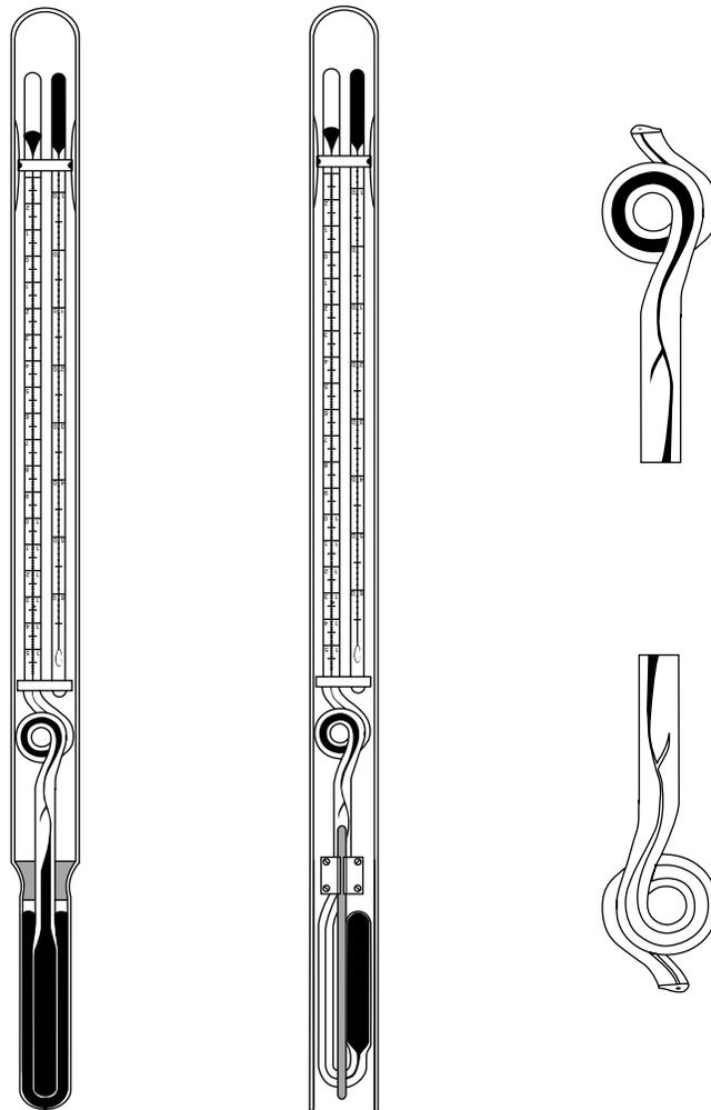
Figure 6.13 **Left:** Protected and unprotected reversing thermometers in set position, before reversal. **Right:** The constricted part of the capillary in set and reversed positions (From von Arx, 1962).
