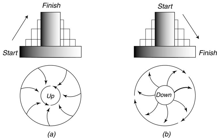
Figure 12.2 Sketch of the production of relative vorticity by the changes in the height of a fluid column. **Left:** vertical stretching reduces the moment of inertia of the column, causing it to spin faster; **Right:** vertical shrinking increases the moment of inertia of the column, causing it to spin slower (from von Arx, 1962).
