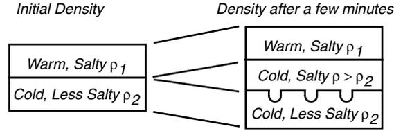
Figure 8.7 **Left:** Initial distribution of density in the vertical. **Right:** After some time, the diffusion of heat leads to a thin unstable layer between the two initially stable layers. The thin unstable layer sinks into the lower layer as salty fingers. The vertical scale in the figures is a few centimeters.
