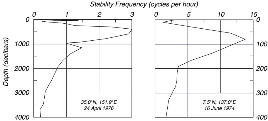
Figure 8.5. Observed stratification frequency in the Pacific. **Left:** Stability of the deep thermocline east of the Kuroshio. **Right:** Stability of a shallow thermocline typical of the tropics. Note the change of scales.
