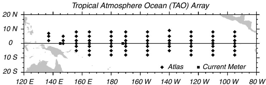
Figure 14.14 Tropical Atmosphere Ocean TAO array of moored buoys operated by the NOAA Pacific Marine Environmental Laboratory with help from Japan, Korea, Taiwan, and France.
