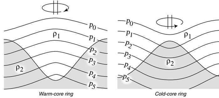
Figure 10.13 Shape of isobaric surfaces  $p_i$  and the interface between two water masses of density  $\rho_1, \rho_2$  if the upper is rotating faster than the lower. **Left:** Anticyclonic motion, warm-core eddy. **Right:** Cyclonic, cold-core eddy. Note that the sea surface  $p_0$  slopes up toward the center of the warm-core ring, and the isopycnal surfaces slope down toward the center (From Defant, 1929).
