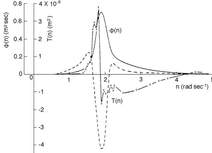
Figure 16.10 The function transferring wave energy from one part of the wave spectrum to another part via nonlinear wave-wave interactions  $T(n)$  where  $n$  is frequency. Dashed curve is for the theoretical spectrum  $\Phi(n)$ ,  $\times - \times$  is for a measured spectrum. The interactions extract energy from high frequency waves and transfer it to low frequency waves, causing the spectrum to change with time and generating waves going faster than the wind, (From Phillips, 1977: 139).
