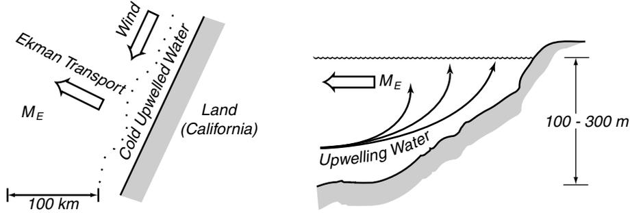
Figure 9.8 Sketch of Ekman transport along a coast leading to upwelling of cold water along the coast. **Left:** Cross section. The water transported offshore must be replaced by water upwelling from below the mixed layer. **Right:** Plan view. North winds along a west coast in the northern hemisphere cause Ekman transports away from the shore.
