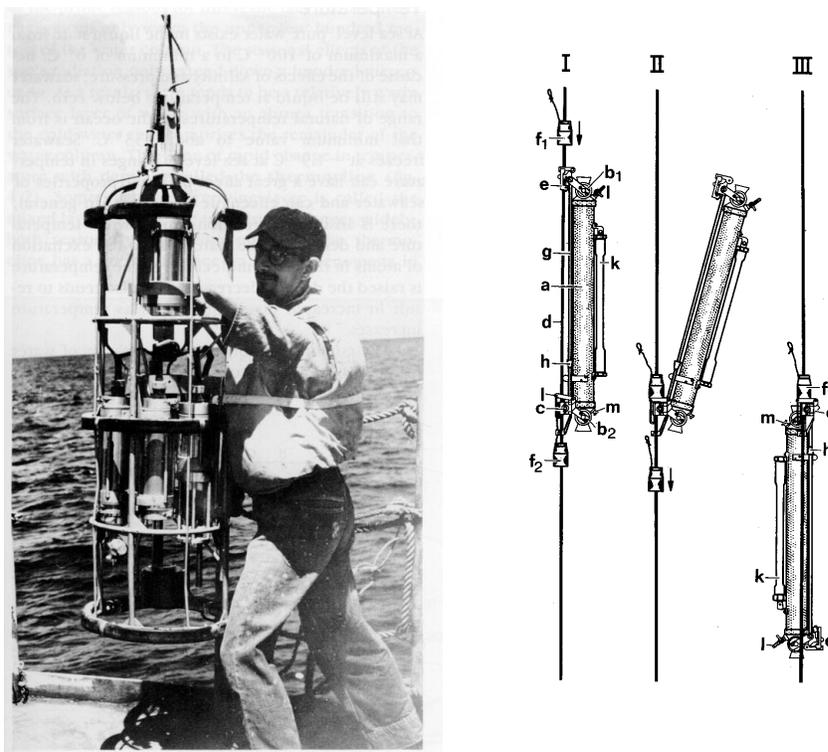
Figure 6.18 **Left** A CTD ready to be lowered over the side of a ship (From Davis, 1987). **Right** Nansen water bottles before (I), during (II), and after (III) reversing. Both instruments are shown at close to the same scale (From Dietrich et al. 1980).
