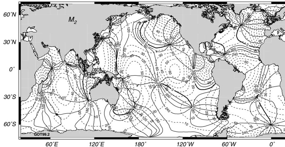
Figure 17.14 Global map of  $M_2$  tide calculated from Topex/Poseidon observations of the height of the sea surface combined with the response method for extracting tidal information. Full lines are contours of constant tidal phase, contour interval is  $30^\circ$ . Dashed lines are lines of constant amplitude, contour interval is 10 cm. (From Richard Ray, NASA Goddard Space Flight Center).
