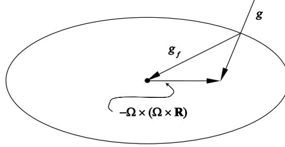
Figure 7.5 Downward acceleration  $g$  of a body at rest on Earth's surface is the sum of gravitational acceleration between the body and Earth's mass  $g_f$  and the centrifugal acceleration due to Earth's rotation  $\boldsymbol{\Omega} \times (\boldsymbol{\Omega} \times \mathbf{R})$ . The surface of an ocean at rest must be perpendicular to  $g$ , and such a surface is close to an ellipsoid of rotation. Earth's ellipticity is greatly exaggerated here.
