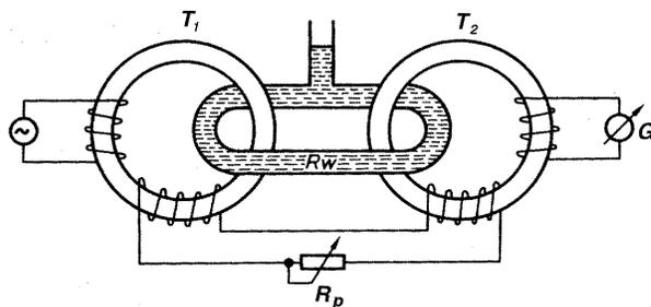
Figure 6.15 The induction method measurement of electrical conductivity uses a sea-water loop which couples two transformer loops  $T_1$  and  $T_2$ . The induced voltage in the second loop is proportional to conductivity  $R_w$  of the water. From Dietrich et al. 1980.
