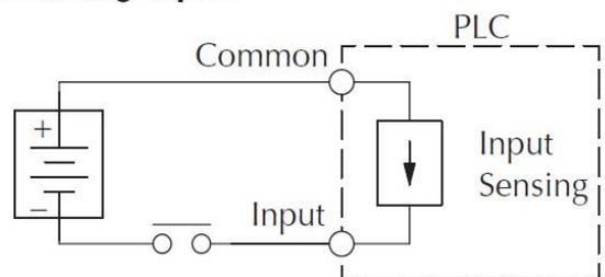
*Typical wiring for sinking and sourcing input devices*
