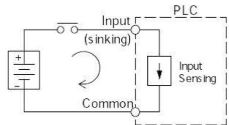
By applying the circuit principles to the four possible combinations of input/output sinking/sourcing types, there are four circuits, as shown below. The common terminal is the terminal that serves as the common return path for all I/O points in the bank.
