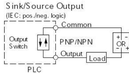
Below are detailed electrical diagrams for sinking and sourcing configurations, showing typical PLC input module and field device circuitry.
