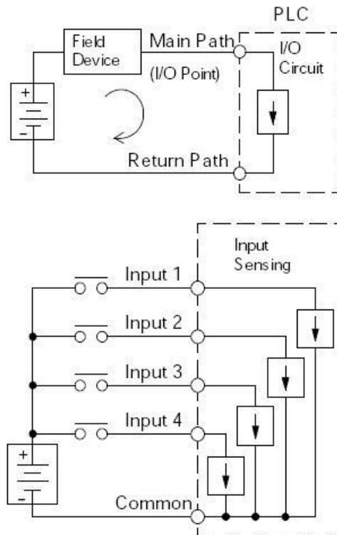
*NOTE: Assuming all input circuits have a similar resistance, the current at the common terminal is four times greater than the current at any one of the inputs. This effect is especially important to note for output circuits, where the current through a common terminal can reach several amperes. You will need to decide whether to fuse each output point individually, or to put a fuse in the common terminal path.*
