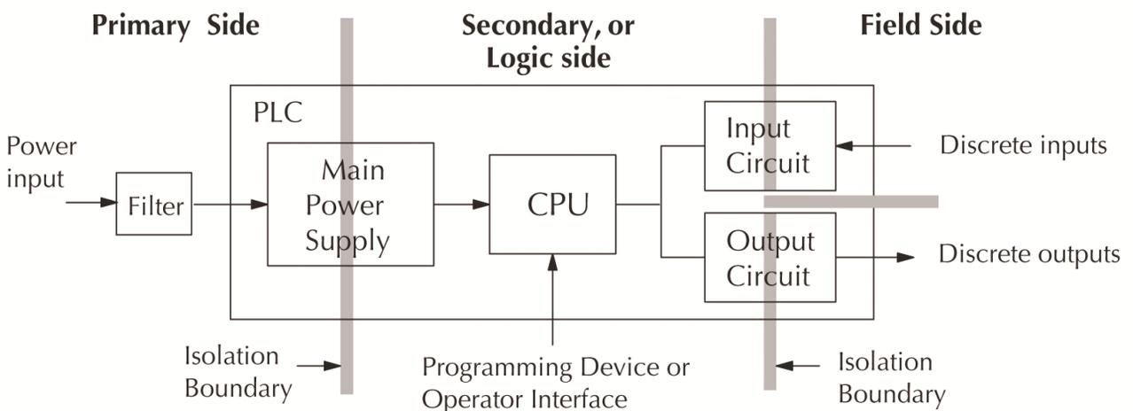
Electrical isolation provides safety, so that a fault in one area does not damage another. Using the figure below as a reference, we see a transformer which provides magnetic isolation between its primary (high voltage) and secondary (control voltage) sides. A powerline filter provides isolation between the control power source and the electronic devices.
