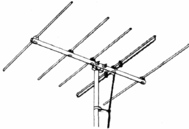
Figure 28.2: In a Yagi-Uda antenna, when a wire antenna is less than half a wavelength, it acts as a waveguide, or a director. Then the wire antenna is slightly more than half a wavelength, it acts as a reflector [129]. Therefore, the antenna radiates predominantly in one direction (courtesy of Wikipedia [130]).
