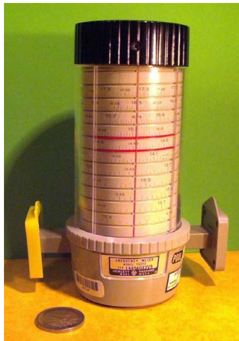
Figure 21.15: An absorption wave meter can be used to measure the frequency of microwave (courtesy of Wiki [119]).
