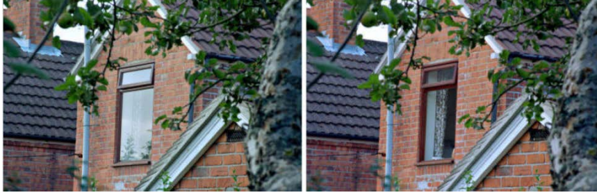
Figure 15.3: Because the TM and TE lights will be reflected differently, polarizer filter can produce remarkable effects on the quality of the photograph [96].
