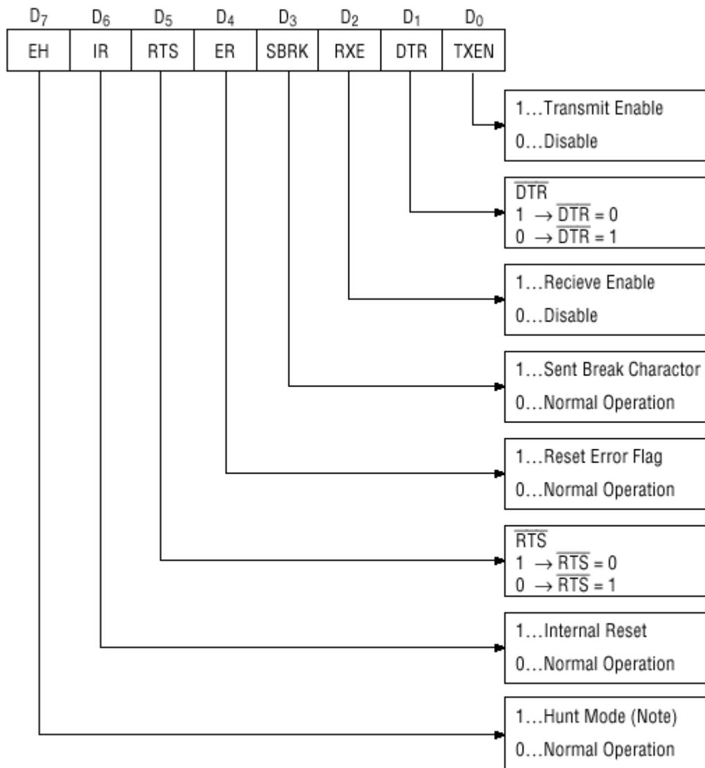
**Note:** Seach mode for synchronous characters in synchronous mode.
