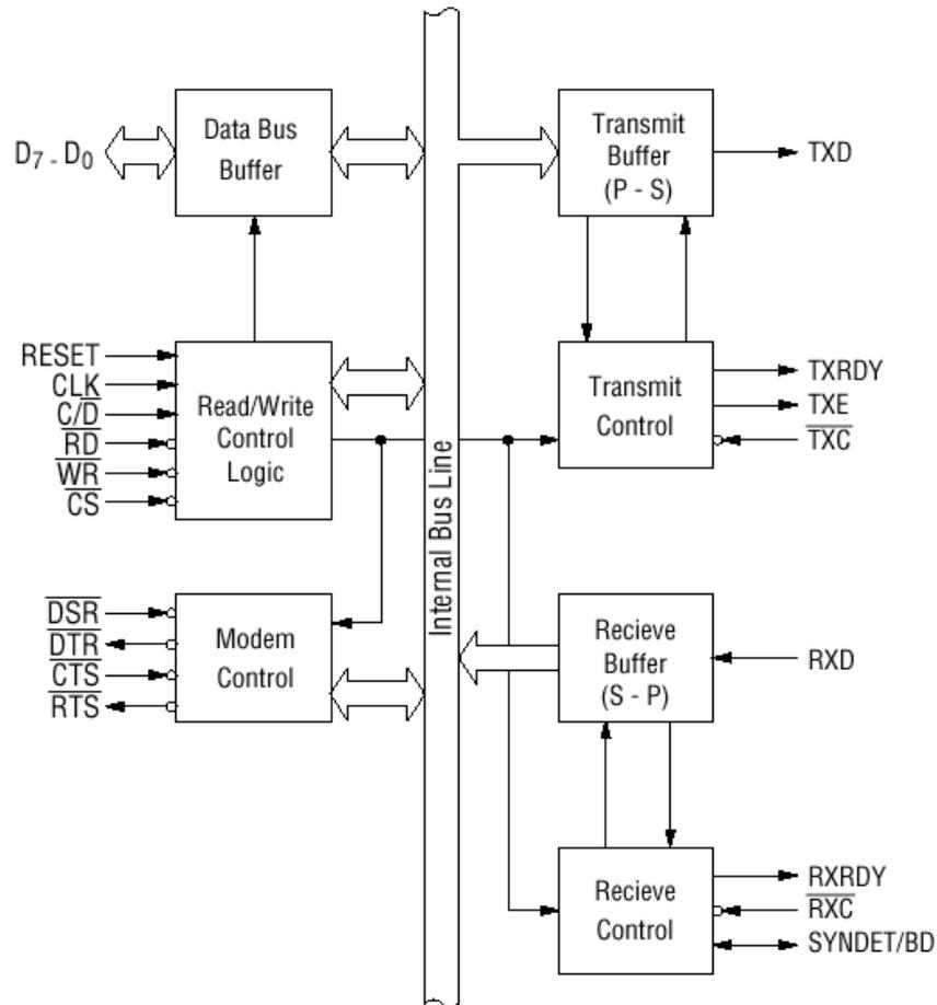
**Block diagram of the 8251 USART (Universal Synchronous Asynchronous Receiver Transmitter)**
