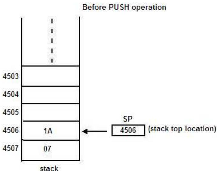
Figure.29 The PUSH operation of the Stack
