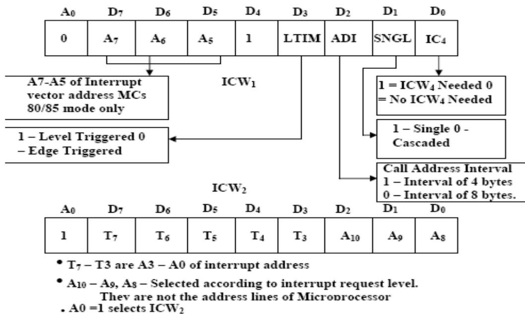
Fig 4 Fig: :tion Command Words ICW<sub>1</sub> and
