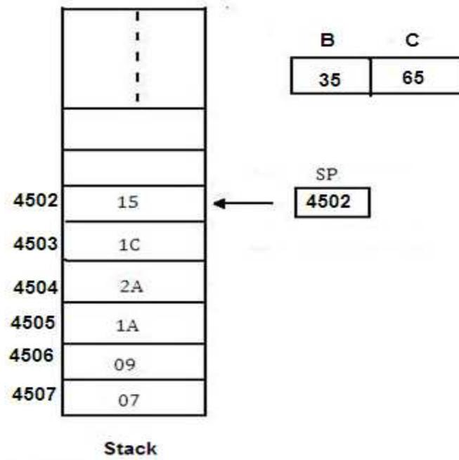
**Figure 31 The POP operation of the Stack**
