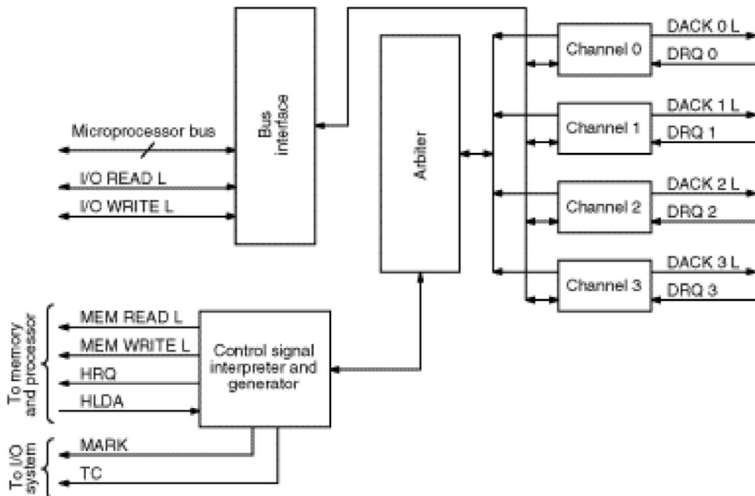
**Figure 5-4:** Structure of the i8527 DMA controller
