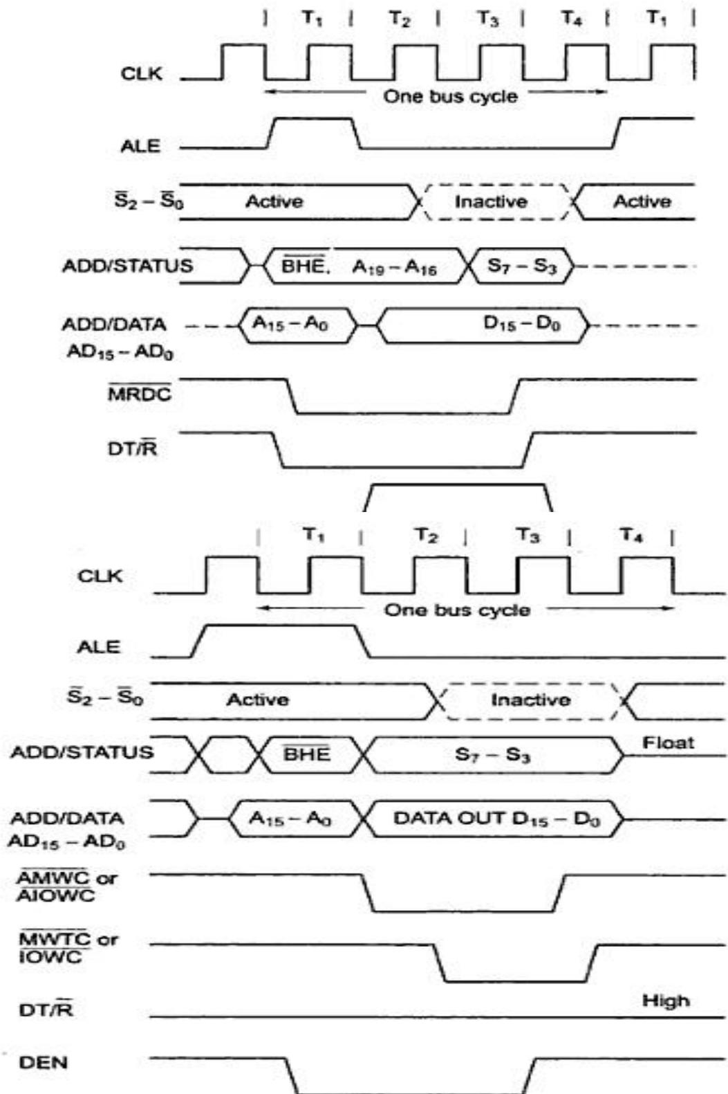
**Fig. 1.16(b)** Memory Write Timing in Maximum Mode
