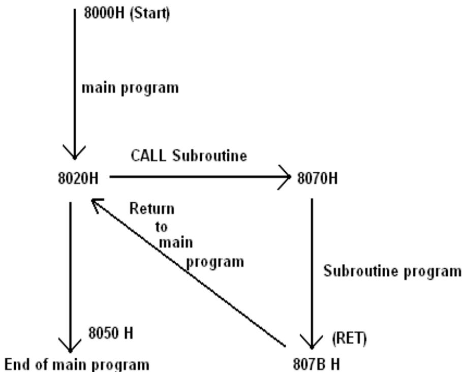
**Fig.33 Diagrammatic representation of subroutine program execution**
