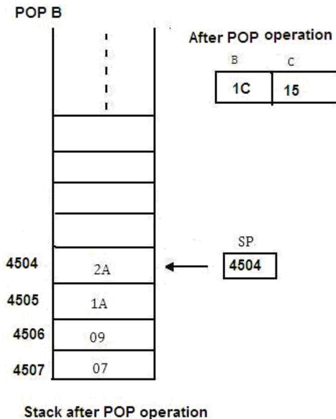
Figure 32 After POP operation the status of the stack
