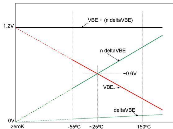
Fig. 7-2: The principle of a bandgap reference.
