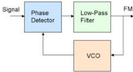
Fig. 12-5: Block diagram of a simple phase-locked loop.
