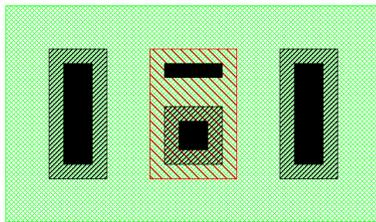
Fig. 17-16: Two collector contacts in an NPN transistors can act as a cross-under.
