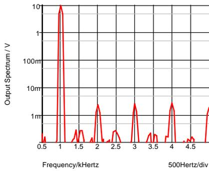
Fig. 14-39: Frequency spectrum in the signal range.
