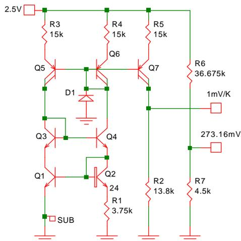
Fig 16-22: A thermometer with a Celsius scale.
