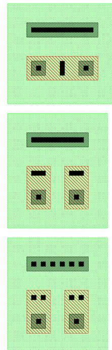
Fig. 17-4: Two-emitter NPN transistors.
