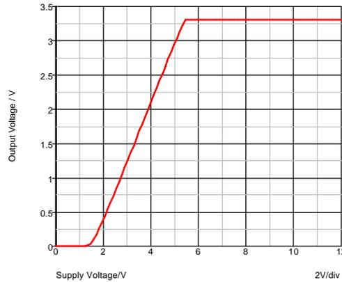
Fig. 14-2: Drop-out voltage of NPN regulator.
