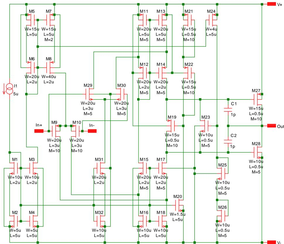
Fig. 8-22: Op-amp with rail-to-rail inputs and output.
