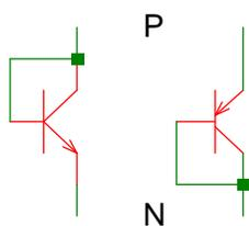
Fig. 1-22: Properly connected diodes in a bipolar process.
