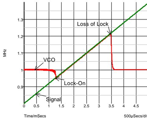
Fig. 12-6: Locking behavior of a phase-locked loop.
