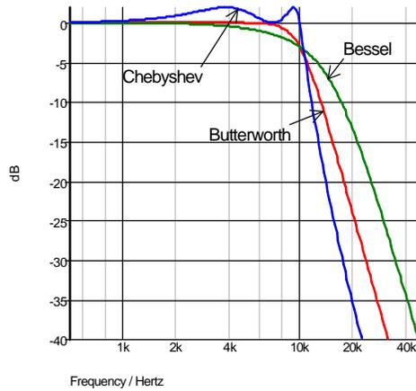
Fig. 13-8: Frequency responses of the three low-pass filters.
