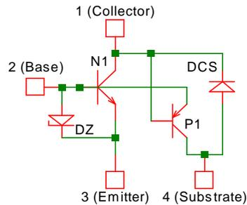
Fig. 2-11: Equivalent circuit for an integrated NPN transistor.
