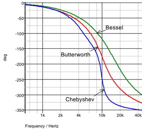
Fig. 13-9: Phase response of the three filters.
