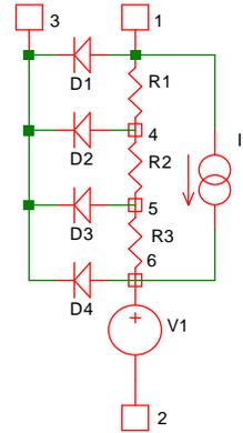
Fig. 2-13: Equivalent circuit for a 3-segment integrated resistor.
