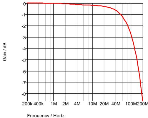
Fig. 2-3: AC analysis: gain (in dB) vs. frequency.
