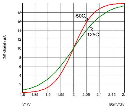
Fig. 4-6: ...and the transconductance also has a temperature coefficient.
