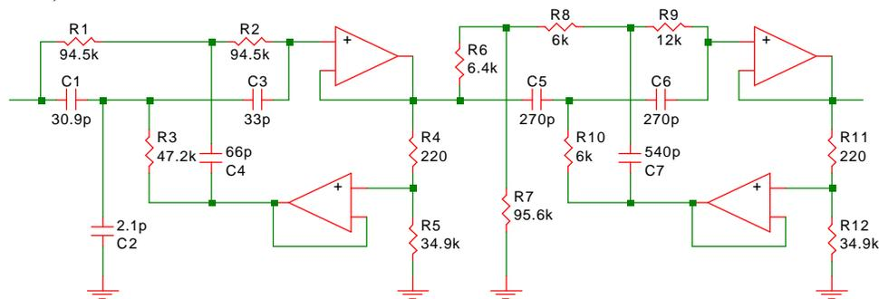
Fig. 13-18: A fourth-order, twin-T elliptic band-pass filter.
