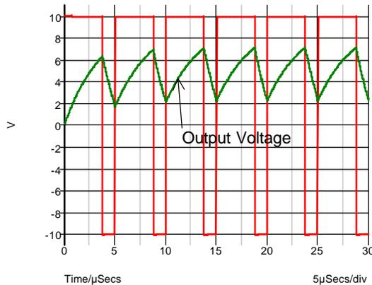
Fig. 14-35: Switching and output waveforms.
