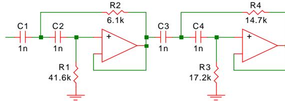
Fig. 13-14: High-pass Sallen & Key filter with Butterworth values.
