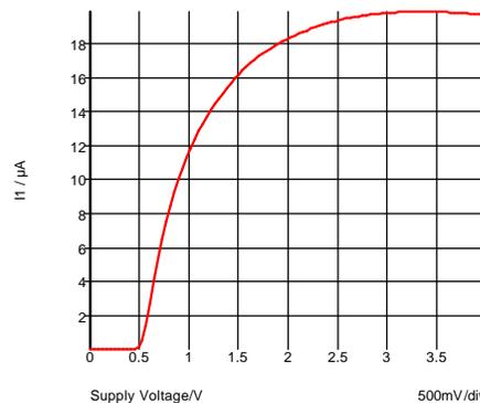
Fig. 5-11:  $I_1$  vs. supply voltage with R3 optimized for the range 3 to 3.6 Volts.
