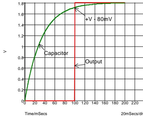
Fig. 11-20: Switching threshold of the 1.8V timer.
