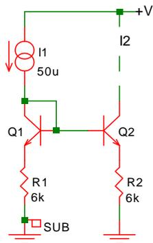
Fig. 3-7: Improved current mirror with emitter resistors.
