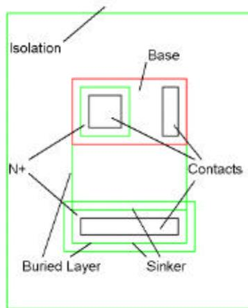
Fig. 17-1: Mask layers for an NPN transistor.
