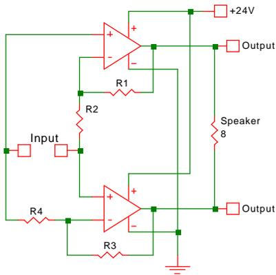
Fig. 14-33: Class AB amplifier with bridge output.
