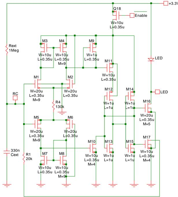
Fig. 11-17: CMOS design for a pulse generator.
