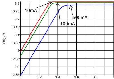
Fig. 14-16: Drop-out voltage.
