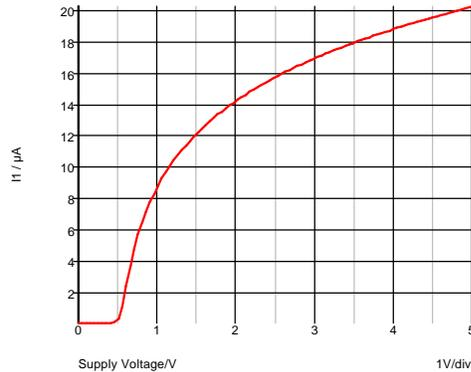
Fig. 5-8:  $I1$  vs. output voltage of figure 5-7.Fig. 5-9:  $I1$  vs. supply voltage of figure 5-7.
