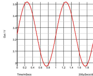
Fig. 4-11: Output signal with a 1mVp sine-wave input.
