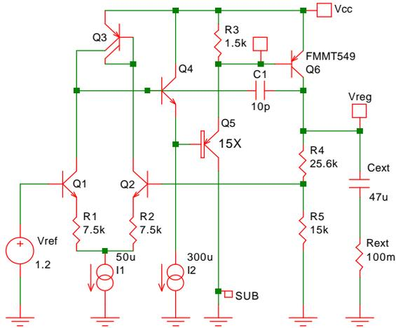
Fig. 14-15: Low drop-out regulator with external PNP transistor.
