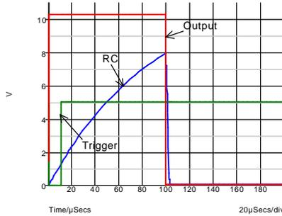
Fig. 11-5: Timer waveforms.
