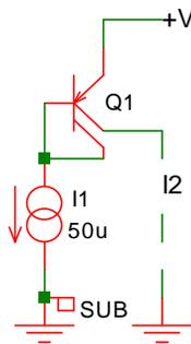
Fig. 3-3: Current mirror with lateral PNP.
