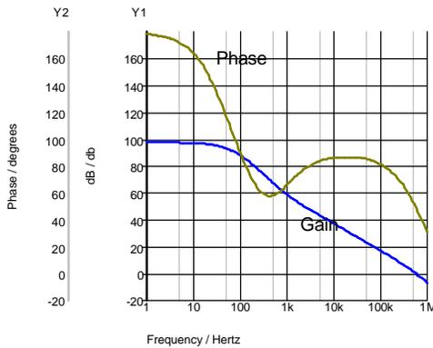
Fig. 14-8: Phase/gain diagram using three compensation capacitors.
