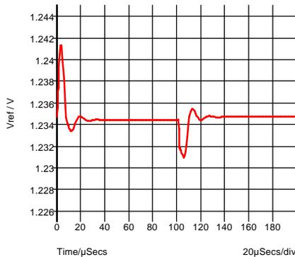
Fig. 7-8: Pulse response, indicating stability.
