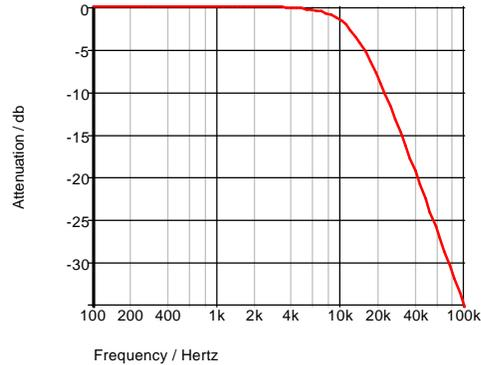
Fig. 13-6: Frequency response of the filter in figure 13-5.
