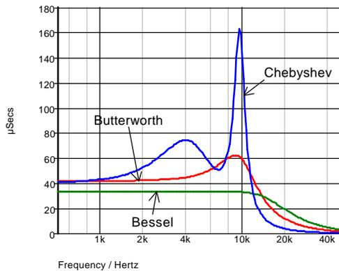
Fig. 13-10: Group delay of the three filters.
