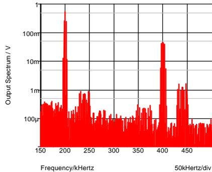
Fig. 14-40: Frequency spectrum in the switching range.
