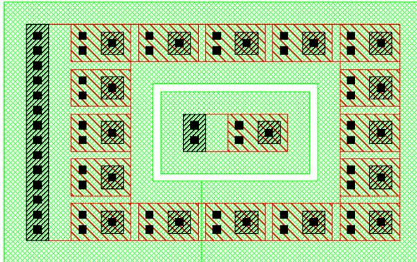
Fig. 17-6: 16:1 emitter ratio with epi-shift mismatch avoided.
