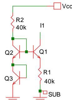
Fig. 5-1: Current source based on VBE (Q3)
