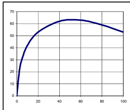
Figure 14-32: Power dissipation vs. power output in a class B amplifier.
