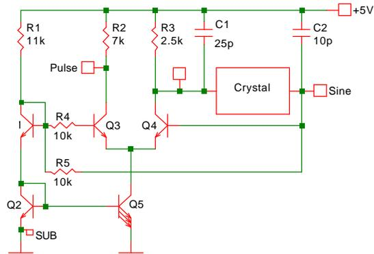
Fig. 11-29: Alternate crystal oscillator with bipolar devices.
