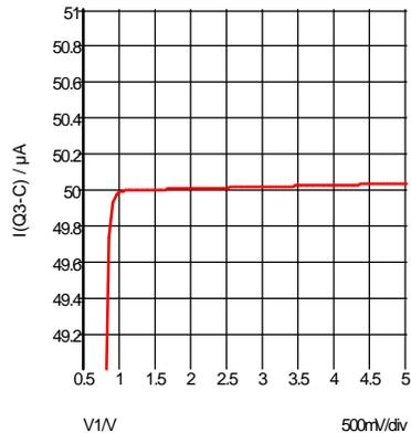
Fig. 3-13: Performance of the four-transistor current mirror.
