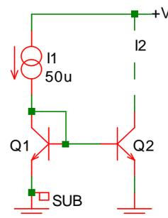
Fig. 3-1: The Widlar current mirror.
