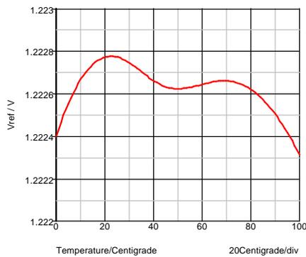
Fig. 7-15: The bow reduced by second-order temperature compensation.
