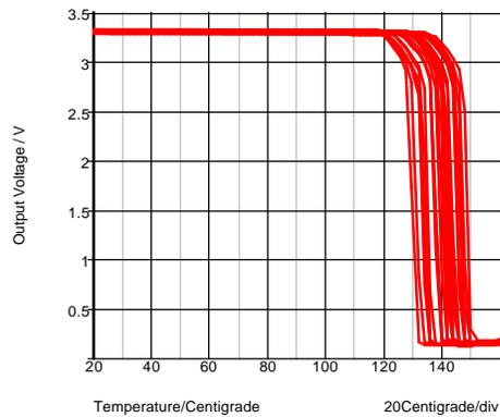
Fig. 14-6: Temperature shut-down.
