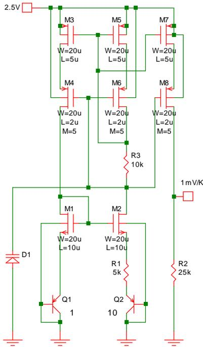
Fig. 16-23: CMOS Thermometer.
