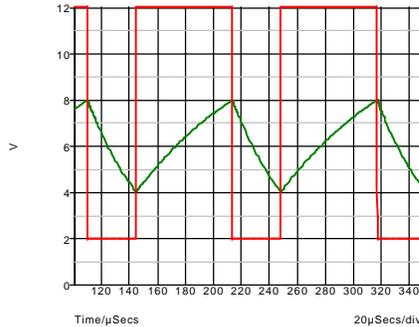
Fig. 11-7: Oscillator waveforms.
