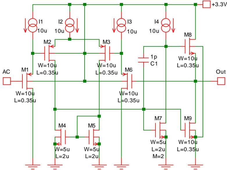
Fig. 16-18: CMOS half-wave rectifier with a single supply.
