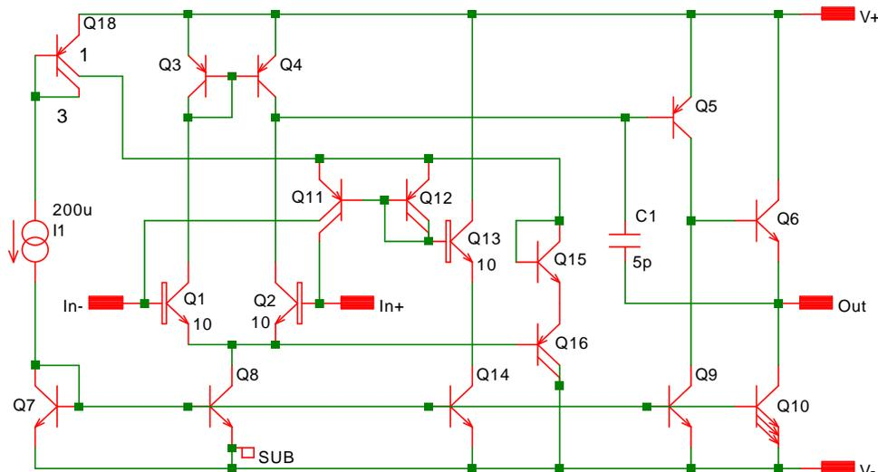
Fig. 8-15: Bipolar op-amp optimized for low noise.
