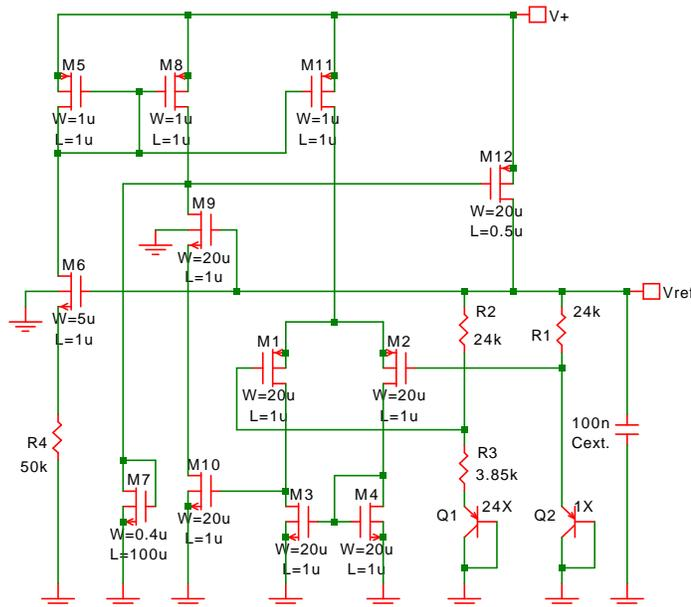
Fig. 7-22: CMOS bandgap reference with substrate diodes.
