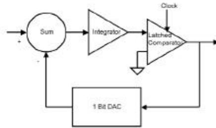
Fig. 15-11: Conventional diagram for a delta-sigma converter.
