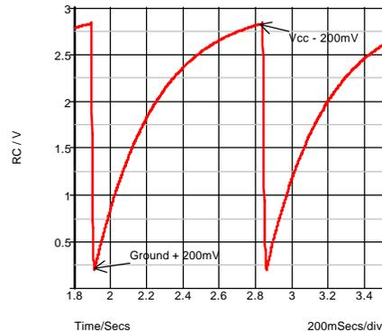
Fig. 11-18: Waveform at RC of figure 11-17.
