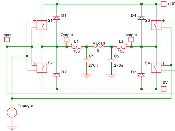
Fig. 14-44: Class D amplifier with bridge output.
