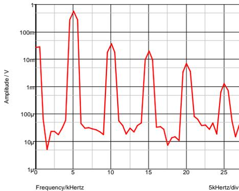
Fig. 6-3: Fast Fourier transform with low resolution.
