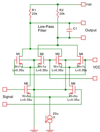
Fig. 12-1: The phase detector.
