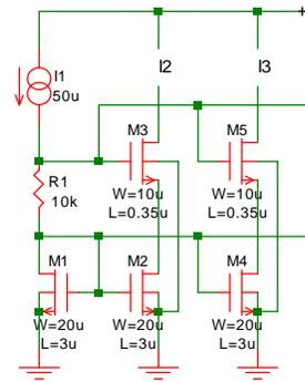
Fig. 3-20: Current mirror with cascode transistors.
