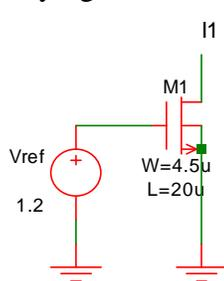
Fig. 5-16: MOS transistor as a current source.
