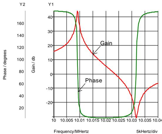
Figure 11-25: Series and parallel resonance of a crystal.
