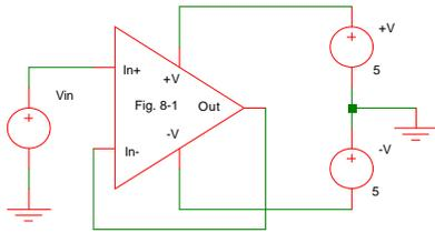
Fig. 8-4: Buffer connection.
