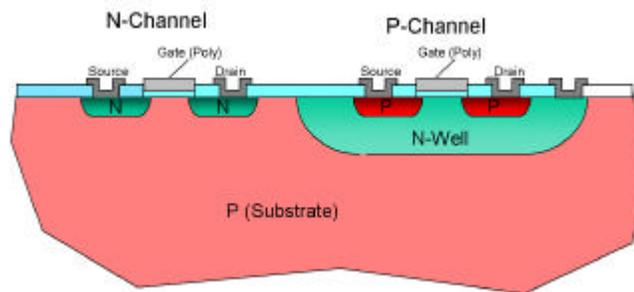
Fig. 1-18: Cross-section of an N-well CMOS process.
