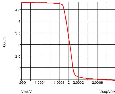
Fig. 4-13: Transfer curve for circuit in figure 4-12.
