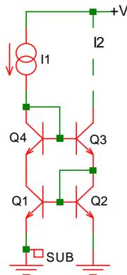
Fig. 3-12: Four-transistor mirror.
