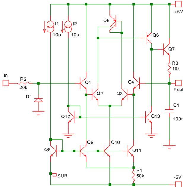
Fig. 16-10: Peak detector with Differential NPN Darlington pair.
