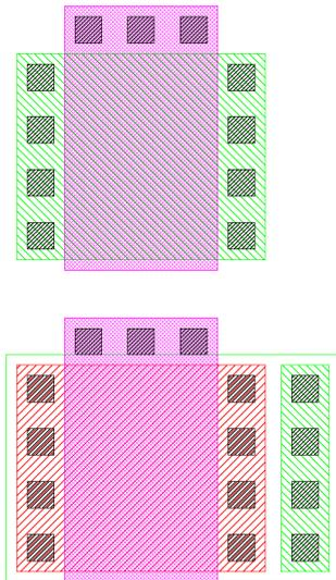
Fig. 17-12: Layout of n-channel (top) and p-channel transistors.
