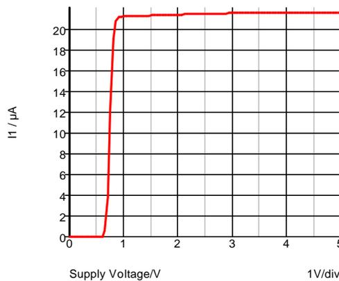
Fig. 5-13:  $I_1$  vs. supply voltage for figure 5-12.
