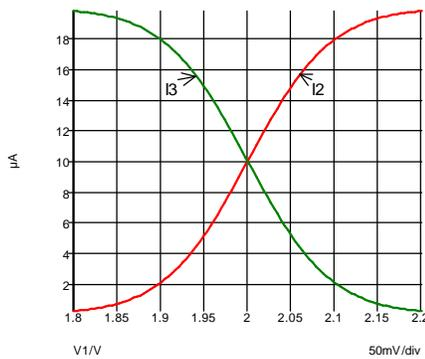
Fig. 4-5: A CMOS differential pair is also non-linear .....
