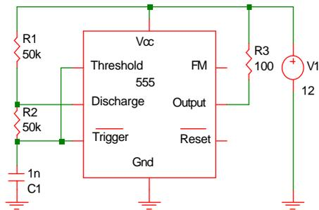
Fig. 11-6: Oscillator connection of the 555.
