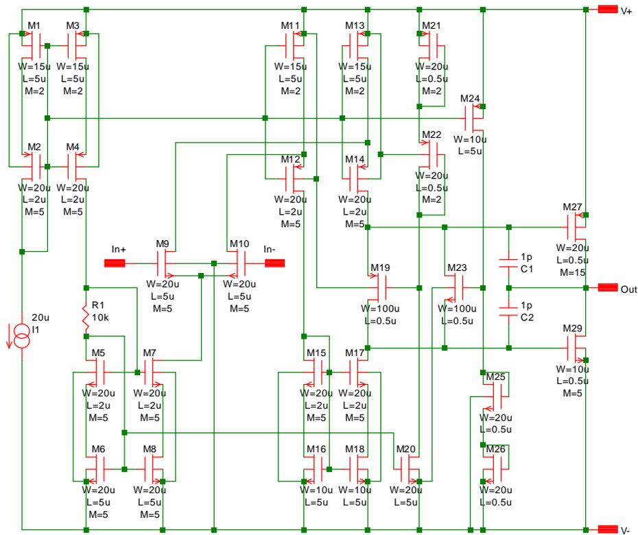
Fig. 8-18: Op-amp with a more capable rail-to-rail output stage.
