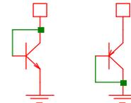
Fig. 16-24: Diode thermometers
