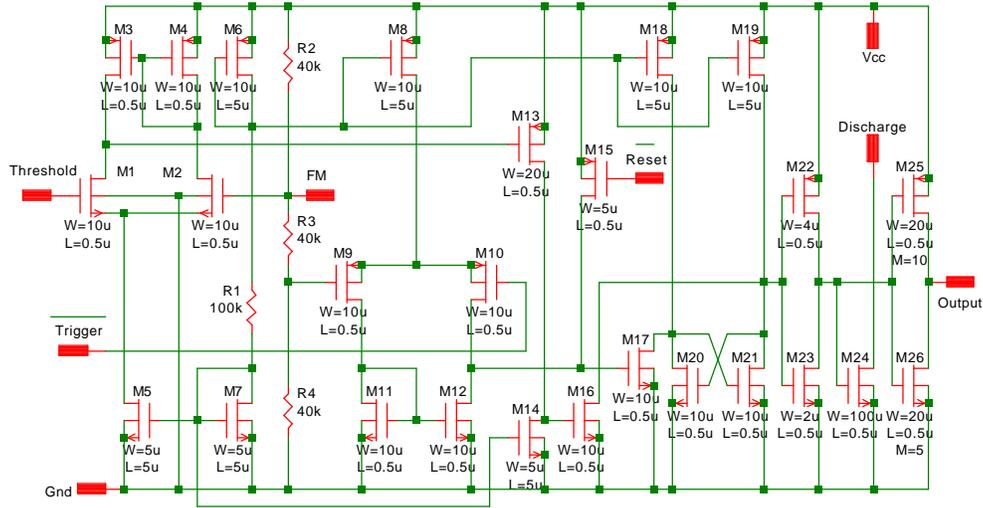
Fig. 11-9: A 5-Volt CMOS version of the 555 timer.
