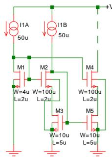
Fig. 3-23: Widely used mirror.
