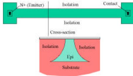
Fig. 10-25: Bulk or Epi-Pinch Resistor.
