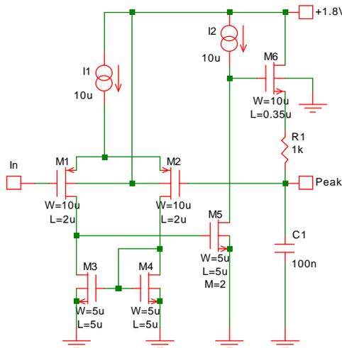
Fig. 16-12: CMOS peak detector.
