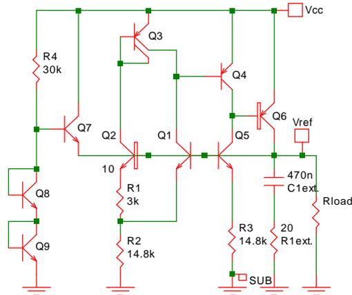
Fig. 7-5: Three terminal Brokaw reference with start-up.
