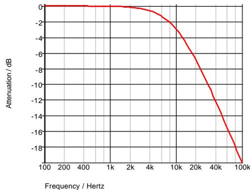
Fig. 13-2: Frequency response of a single-pole filter.
