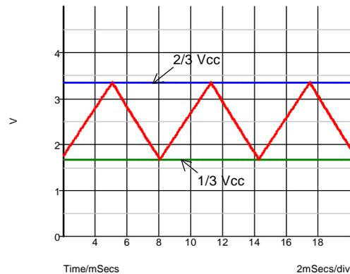
Fig. 11-2: Triangle-wave produced by the 566 oscillator.
