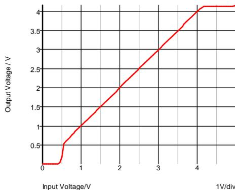
Fig. 2-2: A DC analysis, showing the common-mode range.
