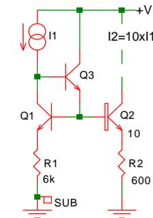
Fig. 3-18: an additional transistor supplies the base current.
