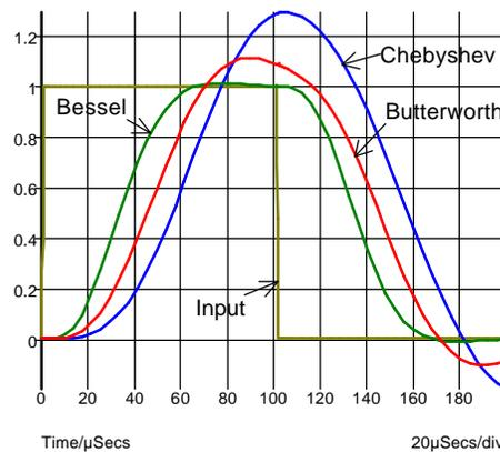
Fig. 13-11: Pulse response of the three filters.
