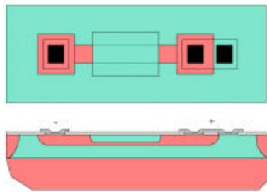
Fig. 1-24: Top view and cross-section of base-pinch resistor.
