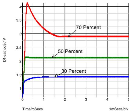
Fig. 14-24: Output voltage for three different duty cycles.
