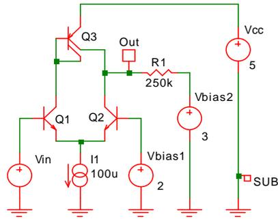
Fig. 4-10: Differential amplifier with an active load.
