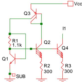
Fig. 5-12: Self-starting current source without large-value resistors.
