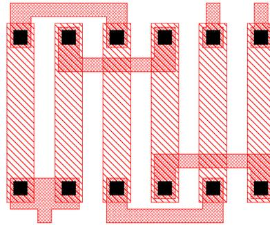
Fig. 17-11: Intermingling and connection of matching resistors.
