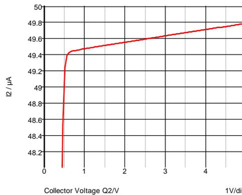
Fig. 3-8: Voltage dependence is now reduced to 0.7%.
