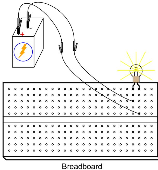
Students often get confused when connecting an ammeter to a breadboard circuit. How can the meter be connected so as to intercept all the circuit's current and not create a short circuit? One easy method that guarantees success is this:
