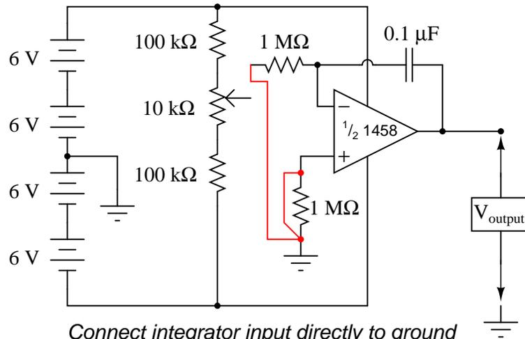
Connect integrator input directly to ground
