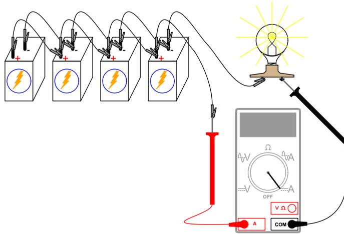
Note the difference in current between the single-battery and total measurements.
