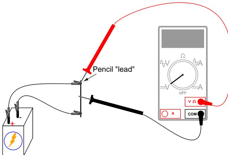
Move the black test probe position along the length of the rod, noting the voltmeter indica-
