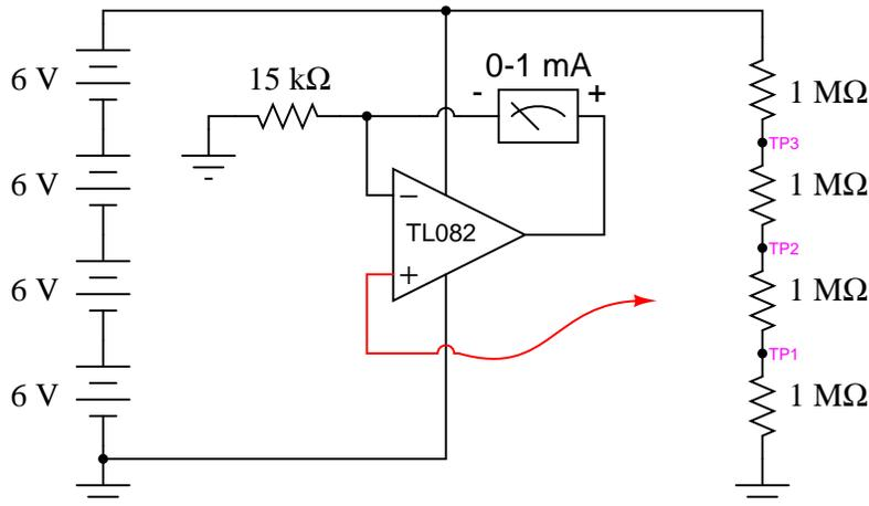
This alteration in the power supply increases the voltages at TP1, TP2, and TP3 to 6, 12, and 18 volts, respectively. With a  $15\text{ k}\Omega$  range resistor and a 1 mA meter movement, measuring 18 volts will gently "peg" the meter, but you should be able to measure the 6 and 12 volt test points just fine.
