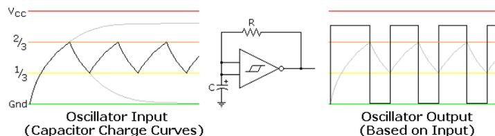
**555 Oscillator Waveforms**
