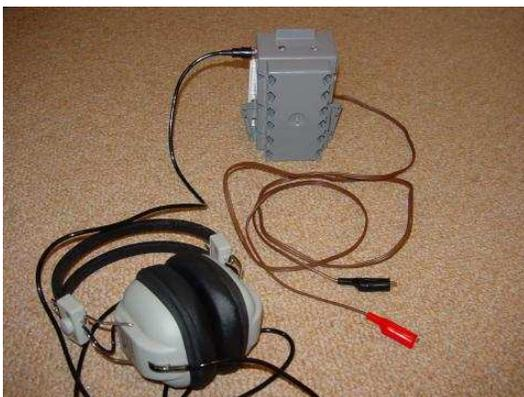
As you can see, I built my detector using scrap parts (household electrical switch/receptacle box for the enclosure, section of brown lamp cord for the test leads). Even some of the internal components were salvaged from scrap (the step-down transformer and headphone jack were
