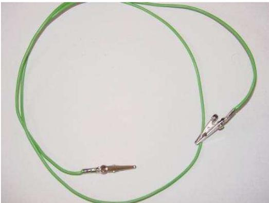
The home-made jumper wires with large, uninsulated (bare metal) alligator clips are okay
