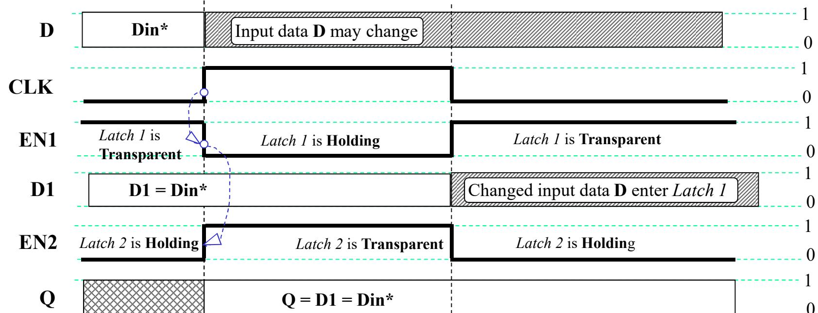
The state of the flip-flop's output  $Q$  copies input  $D$  when the positive edge of the clock  $CLK$  occurs
