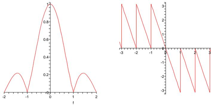
Figure 38: Graph of  $|H(f)|$  (on the left) and  $\Theta(f)$  (on the right) for problem 1b of first set of Chapter 5
