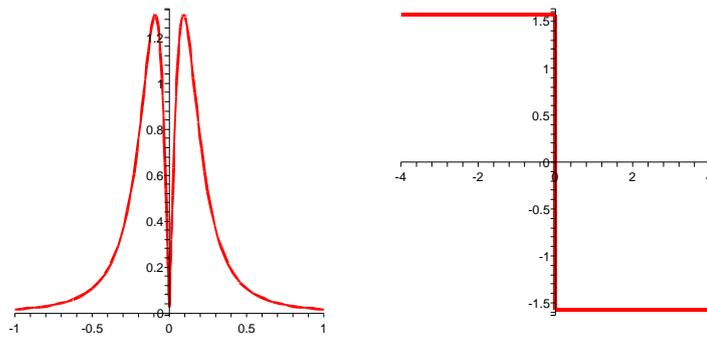
Figure 55: Graph of  $|H(f)|$  (on the left) and  $\Theta(f)$  (on the right) with  $A = \alpha = 1$  for problem 1h of first set of Chapter 5
