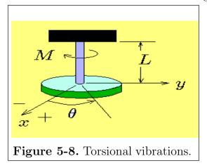
If the disk is rotated through an angle  $\theta$ , there is a restoring moment M produced by the rod. Hooke's law states that the restoring moment is proportional to the angular displacement and
