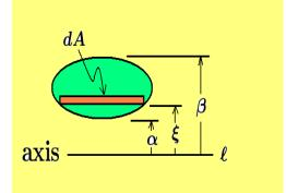
The moment of inertia of a general plane area with respect to an axis can be calculated as follows. Construct elements of area dA all in the shape of a rectangle within the plane area and which are parallel to the axis not passing through the area. By definition, the element of moment of inertia associated with an element of area dA
