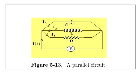
Note that each closed circuit has the same voltage drop. This produces the following equations.
