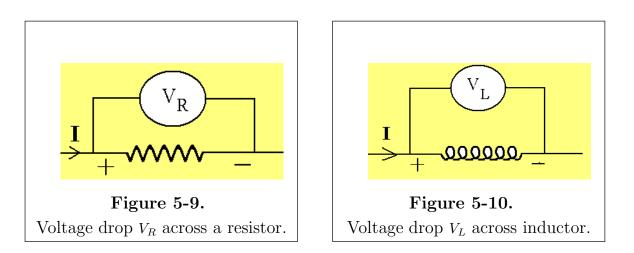
The voltage drop  $V_R$  across a resistance, see figure 5-9, is proportional to the current through the resistance. This is known as **Ohm's law**. The proportionality
