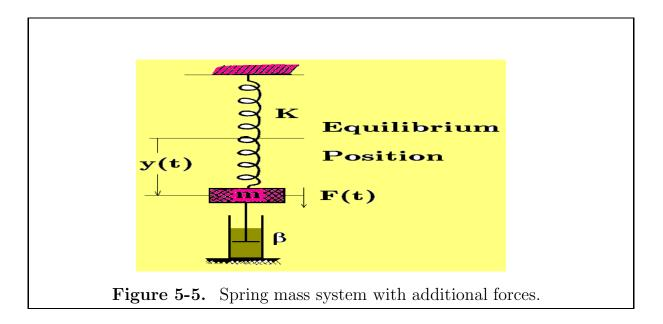
If there is a damping force  $F_D$  which opposes the motion of the mass and the magnitude of the damping force is proportional to the velocity<sup>12</sup>, then this can be represented by
