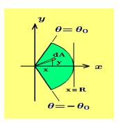
Solution The area inside the circular sector is given by  $A = \theta_0 R^2$ . Move to a general point (x, y) within the sector and construct an element of area  $dA = r dr d\theta$ . The x and y lever arms are given by  $x = r \cos \theta$  and  $y = r \sin \theta$ . The first moment of this area element about the y-axis is given by
