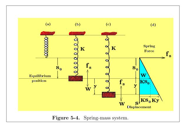
Summation of the forces in equilibrium is represented in figure 5-4(b) which illustrates the spring force equal to the weight acting down or  $f_s = Ks_0 = W$ . This determines the spring constant K as
