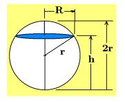
A spherical water tank has a radius of r = 12 feet. Assume h = h(t) is the depth of the water in the spherical tank. The empty space above the water level inside the tank defines a spherical cap whose volume is given by  $V_{cap} = \frac{\pi}{3}(2r - h)^2(r + h)$
