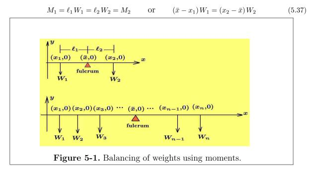
Another way to express the balancing of the see-saw is to examine the distances  $\bar{x} - x_1$  and  $\bar{x} - x_2$ . One distance is positive and the other is negative and the product  $(\bar{x} - x_1)W_1$  gives a positive moment and the product  $(\bar{x} - x_2)W_2$  gives a negative moment. One can then say that the moments produced by the weights balance if  $\bar{x}$  is selected such that the sum of the moments is zero or
