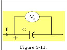
The voltage drop  $V_C$  across a capacitance, see figure 5-11, is proportional to the charge Q of the capacitance. The proportionality constant is denoted 1/C. In symbols this is represented as
