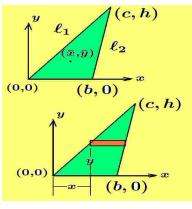
The equation of the line  $\ell_1$  with slope h/c is given by y = (h/c)x. The equation of the line  $\ell_2$ with slope h/(c-b) is given by y = [h/(c-b)](x-b)Construct a horizontal element of area
