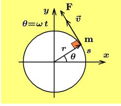
Consider a particle P with constant mass m rotating in a circle of radius r about the origin having a tangential force F producing the motion. Let  $\theta$  denote the angular displacement of the particle,  $\omega = \frac{d\theta}{dt}$  the angular velocity of the particle,  $\frac{d\omega}{dt} = \frac{d^2\theta}{dt^2} = \alpha$ , the angular acceleration of the particle. Newton's second law of motion can then be expressed  $F = m \frac{dv}{dt}$ .
