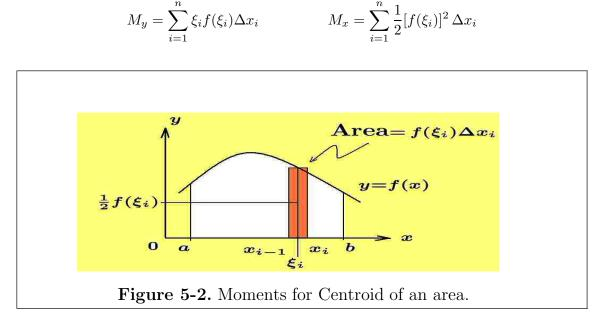
Neglecting infinitesimals of higher order and using the fundamental theorem of integral calculus one finds that in the limit as  $\Delta x_i \rightarrow 0$ , the above sums become the definite integrals
