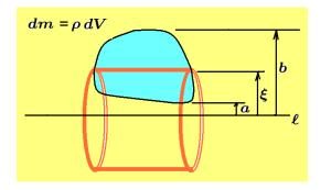
In the study of mechanics one frequently encounters the necessity to calculate the moment of inertia of a solid which is generated by revolving a plane area about an axis. If a rectangular element of area is construct within the plane area and is rotated about an axis  $\ell$  not
