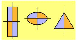
If an object has an **axis of symmetry**, then the **centroid of the object must lie on this line**. For example, if an area has a line of symmetry, then when the area is rotated 180° about this line the area has its same shape. Examine the
