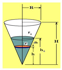
A right circular conical water tank, as illustrated has a top radius R and height H. Assume water is in the tank at a depth  $h_0$ . Let  $\omega = 62.5 \, lbs/ft^3$  denote the density of water.
