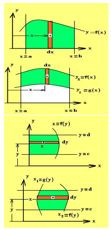
Note that in determining the above lever arm distances the infinitesimals of higher order have been neglected.
