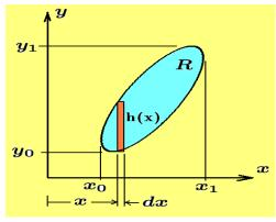
Pappus's<sup>25</sup> theorem states that if a region R is rotated about a line which does not pass through the region, then the volume of the solid of revolution equals the area of the region R multiplied by the distance traveled by the centroid of the region R. Assume the region R illustrated is rotated about the y-axis.
