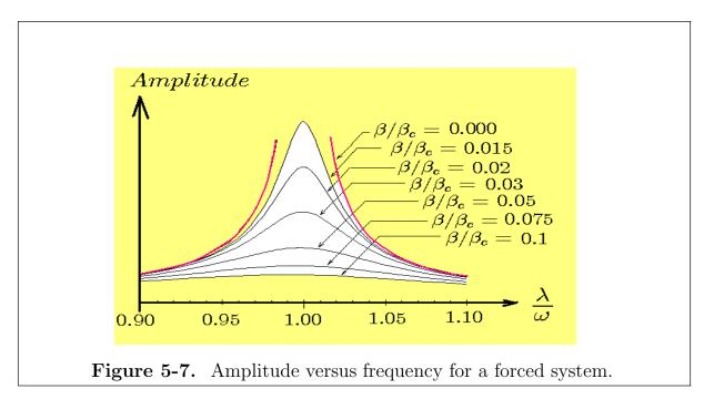
This amplitude, given by equation (5.131), has a maximum value when the denominator is a minimum. Let
