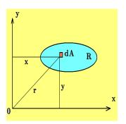
Given a region R one can construct at a general point  $(x, y) \in R$  an element of area dA. This element of area has a second moment of inertia about the y-axis given by
