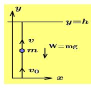
Consider a ball of mass m which is thrown vertically upward with an initial velocity  $v_0$ . Neglect air resistance so that the only force acting on the ball is the force due to gravity and construct a coordinate system with the origin placed at the point where the ball is released. Here the upward direction is taken as positive and by Newton's second law one can write
