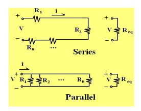
(a) (Resistors in Series) Show that Ohm's law requires the voltage drop in moving around the series circuit requires  $V = iR_1 + iR_2 + \cdots + iR_n$ and so one can replace the sum of the resistors by an equivalent resistance  $R_{eq}$  given by
