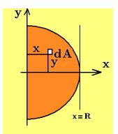
**Solution** The area inside the semi-circle is  $A = \frac{\pi}{2}R^2$ . At a general point (x, y) within the semi-circle construct an element of area dA = dx dy, then the first moment about the y-axis is given by
