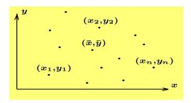
Use the x and y-axes as the lines about which one can take first moments associated with the given point masses. If  $m = \sum_{i=1}^{n} m_i$  is the total sum of all the point masses, then if this mass were placed at the point  $(\bar{x}, \bar{y})$  it would produce first moments about these axes given by
