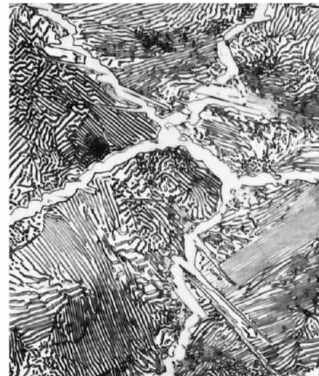
**FIGURE 9.30** Photomicrograph of a 1.4 wt% C steel having a microstructure consisting of a white proeutectoid cementite network surrounding the pearlite colonies. 1000 $\times$ . (Copyright 1971 by United States Steel Corporation.)
