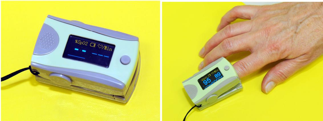
*Fig. 16-6: SpO<sub>2</sub> and pulse measuring with pulse oximeter*
