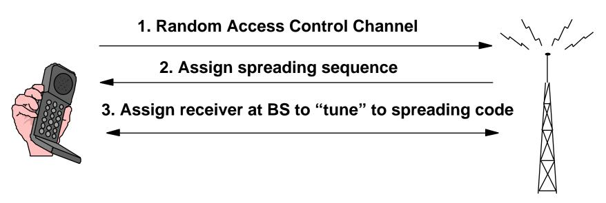
Scheme requires a separate receiver for each active spreading sequence Qualcomm IS-95: 64 assignments are possible Overhead associated with set-up
