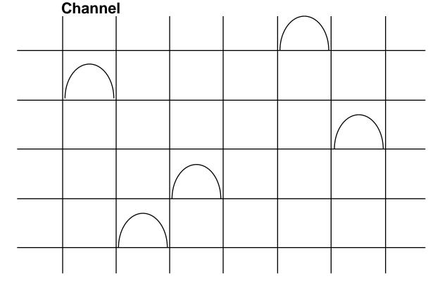
Interference Tolerant: Anti-Jam
