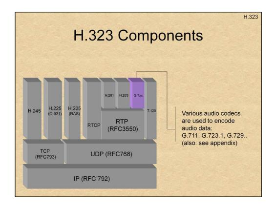
Similarly, G.7xx standards are used for audio data: *(for more on this, see appendix).* Codecs are rated by a Mean Opinion Score – MOS, ranging from 1 (Bad) to 5 (Excellent) – according to the ITU standard P.800.
