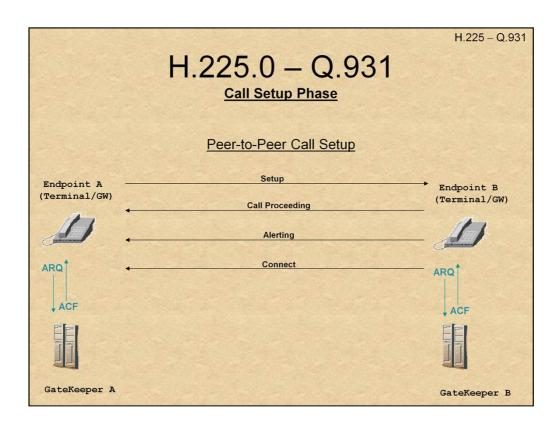
Note that the H.225 messages are not independent of the RAS messages. Both the source and target Gatekeepers (if present) must approve (i.e. send ACFs) the call, otherwise it simply will not happen. For zone-internal calls, the local Gatekeeper is consulted.
