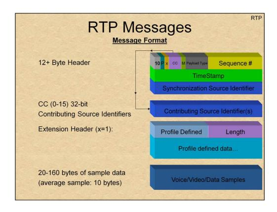
RTP Headers are fixed 12-byte headers, including only the necessary fields for transport management. The fields are listed below:
