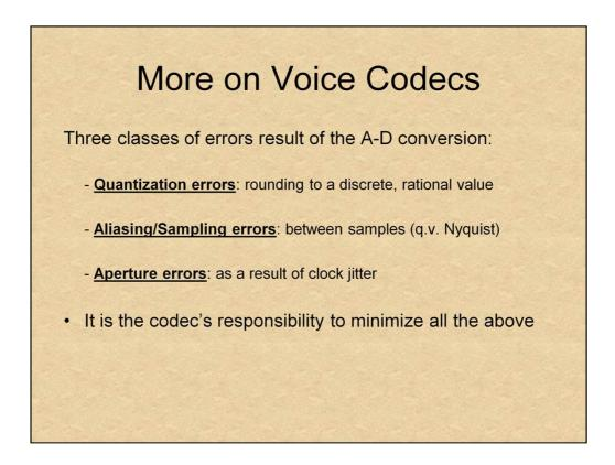
Analog signals are continuous in both time and amplitude. They can be perceived as a function from time to the the signal output units, where both axes are measured in the real numbers. Digital signals, however, are of finite length – and therefore rational. As a result, digital of any resolution will still fall short of the corresponding analog.
