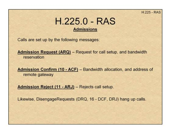
The Admission messages are used to query the gatekeeper, if present, to allow the call to proceed. This can involve validating the call vs. the local administrative policy, reserve proper bandwidth, etc. Similar to the Locate requests, they may be confirmed or rejected.
