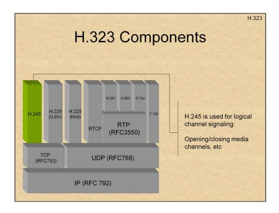
H.245 – "Control protocol for multimedia communication" defines the protocol that is used for logical channel control, or signaling. This involves setting up the transport channels for the various media streams.
