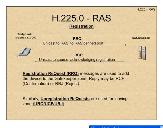
**Advanced Calling Options** ? 🗙 To register, a device supplies one of two: Gatekeeper settings H.323 ID: An email address "account" 🖉 👼 🗌 Use a gate<u>k</u>eeper to place calls E.164 Address: A.K.A a phone number. -Log on using my account name A RCF confirms the device is registered, Log on using my phone number and may be found by entities looking it up (see next page). Gateway settings Use a gateway to call telephones and videoconferencing systems. ΟK Cancel
