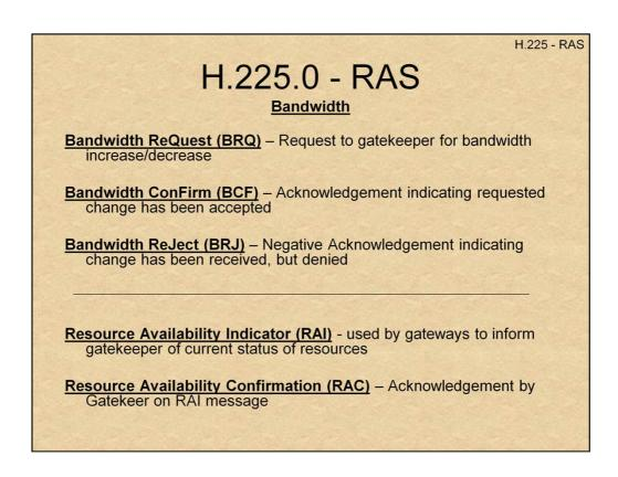
The Bandwidth increase/decrease requests are passed between endpoint and gatekeeper, and offer no guarantee as to bandwidth allocated by the rest of the network (i.e. from Gatekeeper and onwards).
