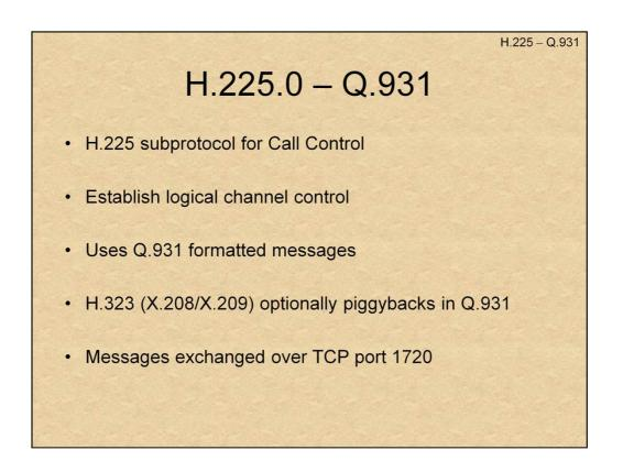
H.225.0/Q.931 is a TOTALLY different protocol, and has little to do with the other component, RAS. Q.931 has been ported from ISDN signaling.
