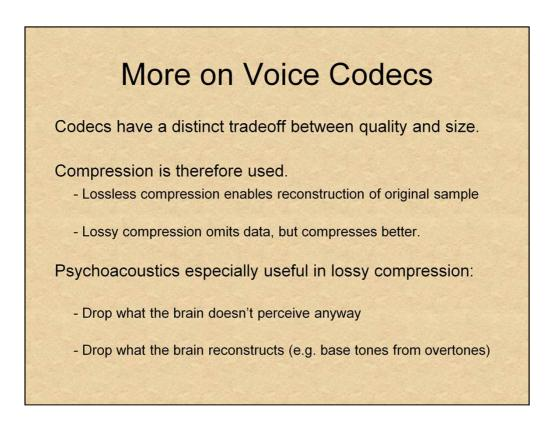
As can be seen in the table showing various sample rates, more samples of greater sample size = better quality. But that also means greater bandwidth. Most codecs therefore use some form of compression.
