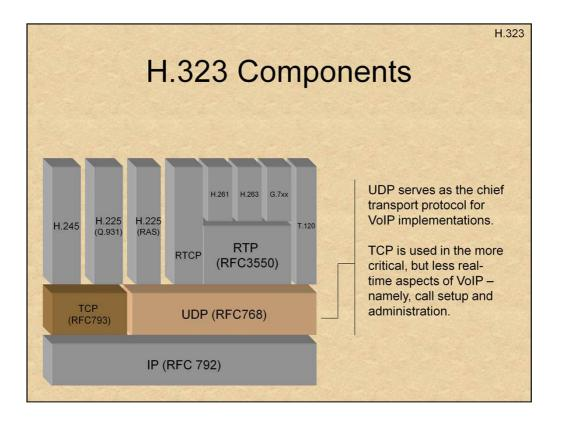
Contrary to many other protocols, VoIP primarily used UDP, and not TCP. While TCP is, by far, the more reliable of the two, it is incompatible with the Real-Time requirements of VoIP. This is due to TCP's slow nature, resulting from its acknowledgements:
