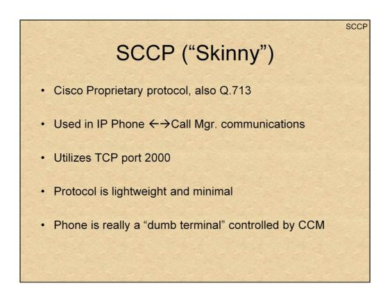
The Cisco "Skinny" protocol was originally developed by the Selsius Corporation. With their acquisition by Cisco, this became a Cisco propietary protocol, that is used in the communication between the Cisco IP Phones (mostly 79xx) and the Cisco Call Manager.
