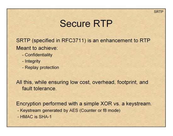
In order to provide security for RTP and RTCP, a proposed extension, known as <u>Secure RTP</u> (SRTP) specified in <u>RFC3711</u>, has been proposed.
