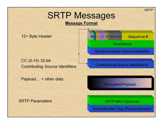
SRTP encrypts the RTP payload, and authenticates the entire packet. It piggybacks over normal RTP by appending two fields to an RTP message:
