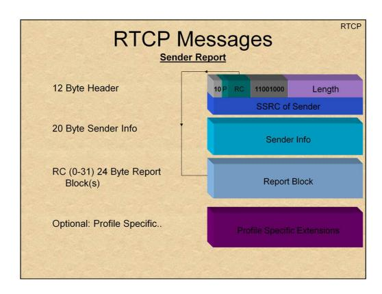
RTCP's "Sender Report" is comprised of a fixed 20-byte "Sender Info" block, and an optional 0-31 (5-bit value - RC) "Report Blocks". Each report block is 24 bytes.
