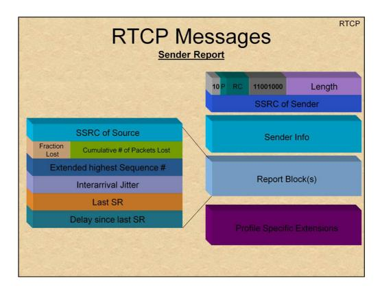
The "Report Blocks" provide more details as to the source, and allow the determination of network lag and round-trip time. Each is 24 bits, as follows:
