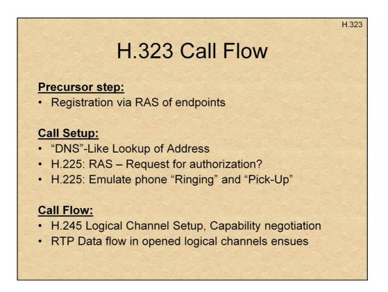
H.323 defines a lengthy process to setup a multimedia call. The process consists of the following stages as shown above. We will now focus on each of these stages.
