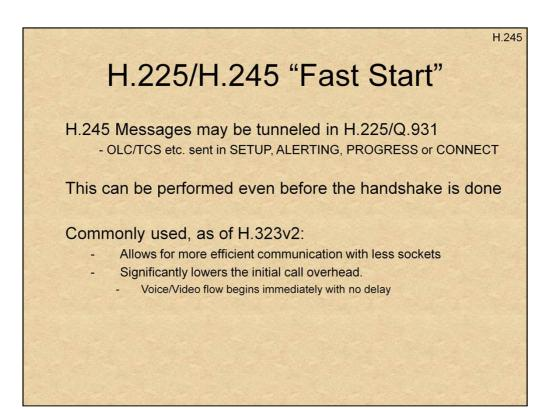
H.323v2 and above support a special form of H.245 tunneling called "Fast Connect" or "Fast Start". This is the sending of optional H.245 "OpenLogicalChannel" messages, that open the RTP media stream, in the SETUP and ALERTING messages. This is meant to prevent the H.245 setup overhead - which often results in voice clipping or silence. The messages are sent in the "fastStart" Information Element of the Q.931 messages.
