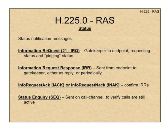
Status notification Information Requests (IRQ) are sent in the opposite direction – from GateKeeper to endpoint. These requests solicit the response from the Endpoint. The endpoint then responds with an IRR. The GateKeeper may then acknowledge (IACK) or negative-acknowledge (INAK) the IRR.
