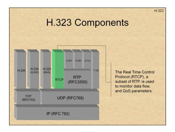
RFC3550, the RTP specification, also introduces the Real Time Control Protocol – RTCP. This is essentially a subset of RTP, used to provide real-time statistics on data flow, so Quality of Service can be measured in real time. RTCP will also be discussed in more detail, shortly.
