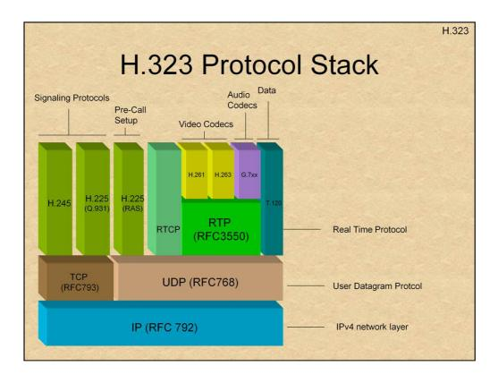
The above slide shows the H.323 "Protocol Stack" – and is an important illustration as to how all the various building blocks of H.323 "fit together".
