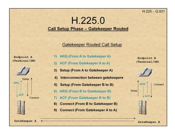
Gatekeeper routed configurations, as the name suggests, enable all calls to be routed through the gatekeepers themselves. Connection is not Point to Point, but Point-GateKeeper-GateKeeper-Point. This is is useful to prevent cases wherein a rogue terminal can attempt connections without GateKeeper approval. In these configurations, the GateKeepers establish the call, and may configure FireWalls to enable specific connections, giving better control over VoIP calls.
