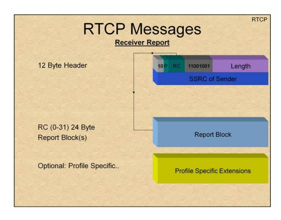
The Receiver Report (PT = 201) is identical to the Sender Report packet, with the exception that the Sender Info Block is omitted.
