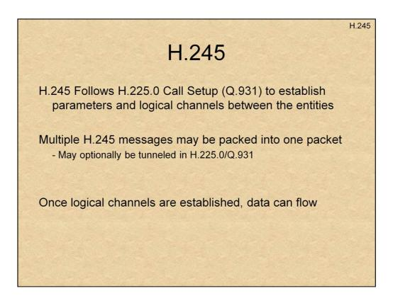
Once H225.0 sets up a logical call "object", another protocol comes into play – this time, H.245. This protocol is used in call control, to set call parameters and establish logical channels between the peers.
