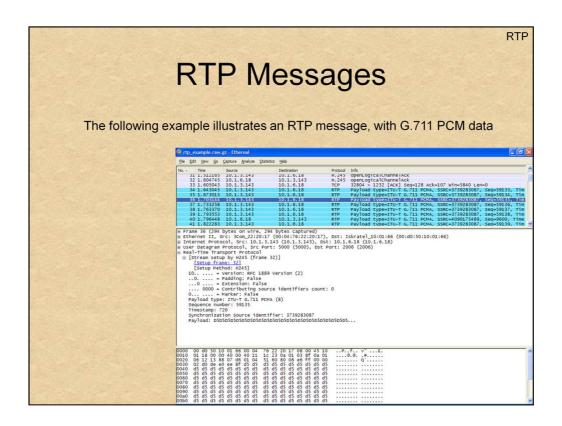
To decode the G.711, any analyzer such as Ethereal can save the payload in the .au format (Sun Audio) which is readily readable by WinAmp or Windows Media Player.
