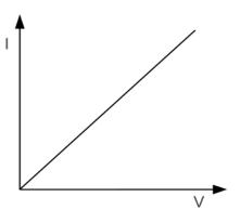
Figure 166: Schematic illustration of the IV characteristic of a tunnel barrier device, i.e. two metals separated by a thin insulator.
