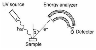
Figure 121: The principle of XPS and UPS
