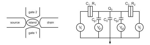
Figure 89: Single electron transistor with two gates and its circuit.
