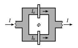
Figure 168: Schematic illustration of a SQUID.
