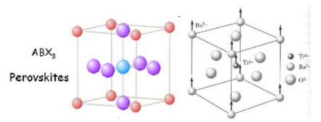
Figure 133: The structure of a perovskit with the example  $BaTiO_3$
