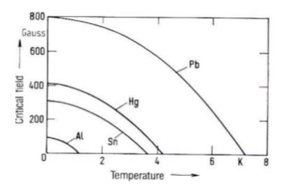
Figure 158: The critical magnetic field  $H_c(T)$  as a function of temperature T. For  $T = T_c$  we have  $H_c(T_c) = 0$ .  $H_c(T)$  separates the normal (above the curve) from the superconducting (below the curve) state.
