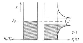
Figure 162: Schematic illustration of the energy gap in a superconductor.
