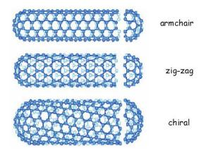
Figure 40: Different types of carbon nanotubes.
