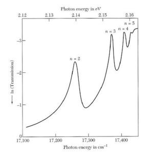
Figure 115: Absorption experiment to show the excitation levels of excitons
