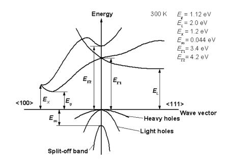
Figure 53: Band structure of Silicon, example for indirect bandgaps
