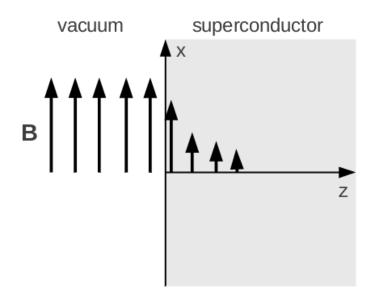
Figure 163: Illustration of the above example of a semi-infinite superconductor in a homogeneous magnetic field in vacuum.
