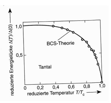
Figure 164: The superconducting band gap versus temperature. Comparison between theoretical (BCS) and experimental data for Ta.
