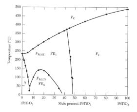
Figure 138: Phase diagram of PZT
