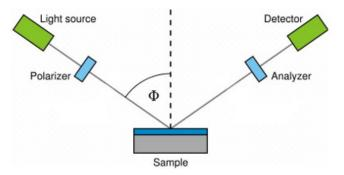
Figure 119: Principle of optical measurement
