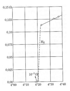
Figure 157: Resistance as a function of temperature for a mercury sample as investigated by K. ONNES.
