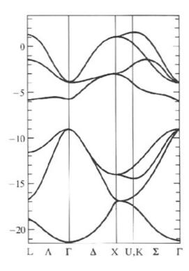
Figure 153: Electron dispersion relation of silicon
