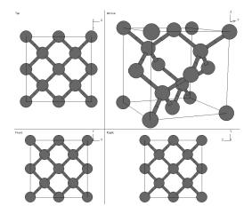
Figure 147: Crystal structure of silicon
