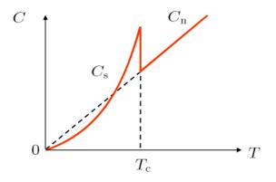
Figure 161: Schematic illustration of the dependence of the heat capacity on temperature in a superconductor.
