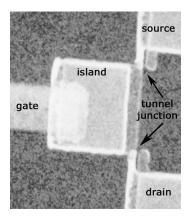
Figure 87: Single electron transistor.
