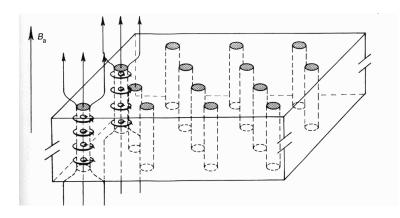
Figure 165: Schematic illustration of the flux penetration in the SHUBNIKOV phase.
