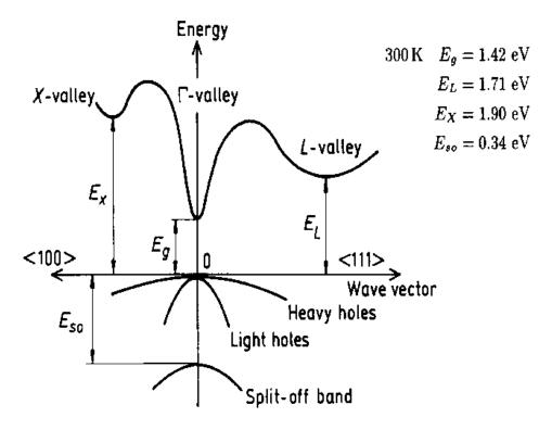
Figure 54: Band structure of Gallium Arsenide, example for direct bandgaps
