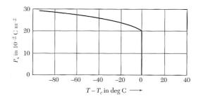
Figure 146: The polarization of  $BaTiO_3$  as a function of temperature
