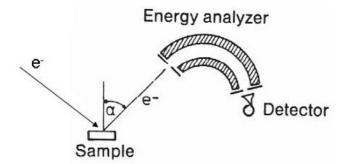
Figure 120: Principle of reflection electron energy loss spectroscopy
