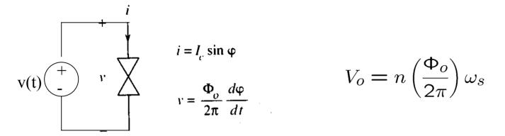
An ac voltage of 1 GHz applied across the junction will give a dc current, at  $V_0 = 0$  and at dc voltages of integral multiples of  $2\mu V$ .
