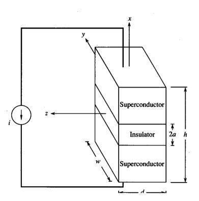
The current must be continuous, so it must flux through the insulating barrier; a process which is not allowed classically. But quantum mechanically the superelectrons can tunnel through the insulating barrier as a supecurrent with zero voltage. This is the Josephson current.
