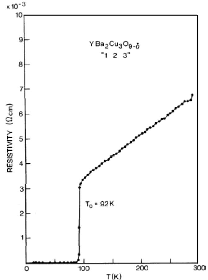
Figure 1.14. Resistivity of a single-phase  $\text{YBa}_2\text{Cu}_3\text{O}_9$  sample as a function of temperature.
