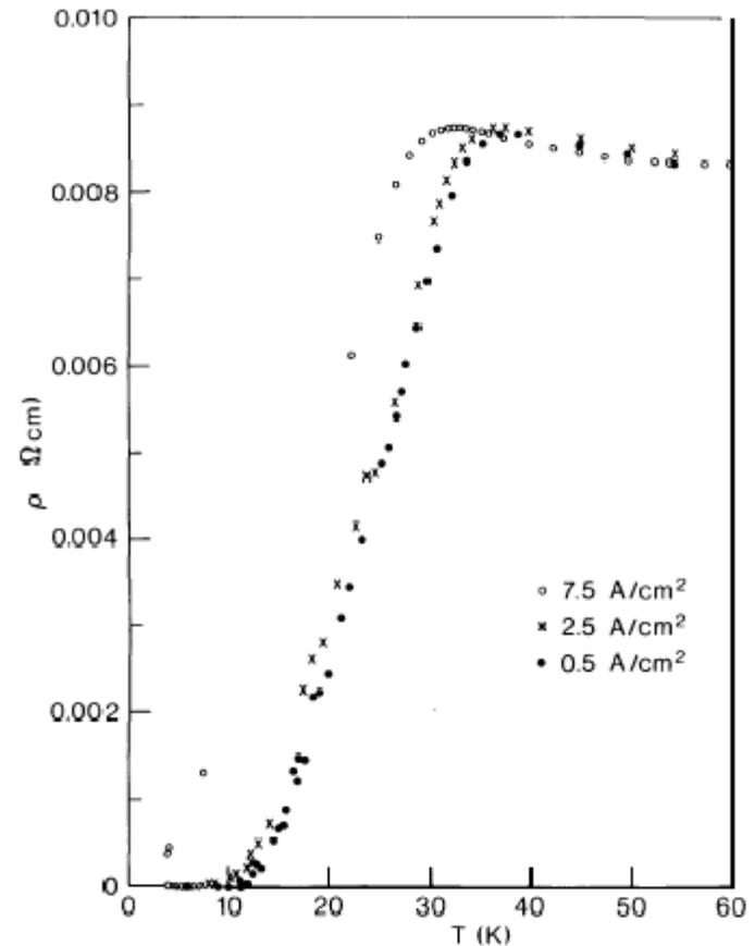
Figure 1.5. Low-temperature resistivity of a sample with  $x(\text{Ba}) = 0.75$ , recorded for different current densities. From [1.19], © Springer-Verlag 1986.
