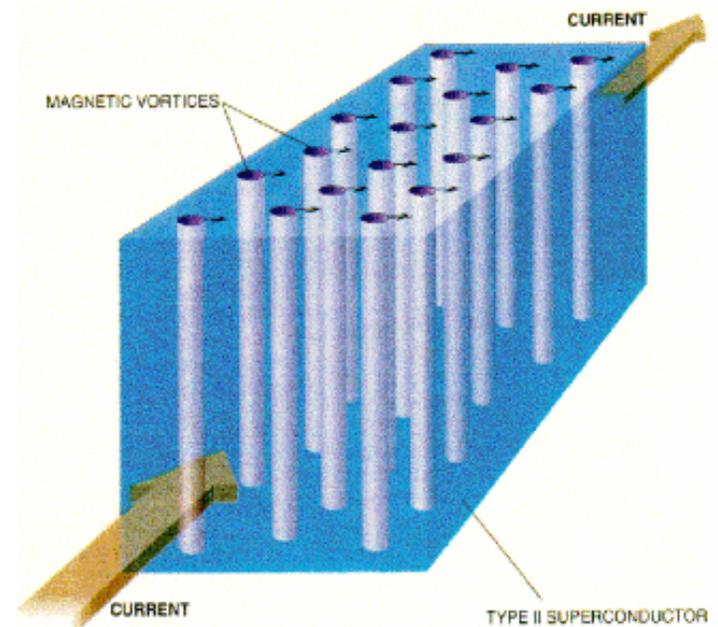
**A current-carrying type II superconductor in the mixed state**
