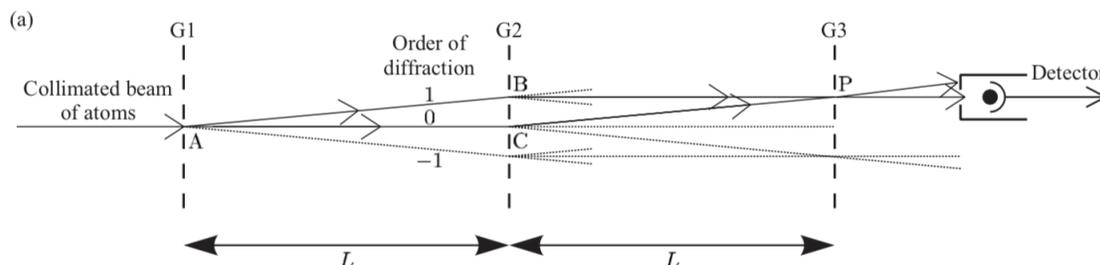
The diffraction gratings here are identical, and spaced so that the slits of one fall at the maxima of the previous one. As a result, atoms can propagate from A to P via either B or C. This is precisely the form of a Mach–Zehnder interferometer.
