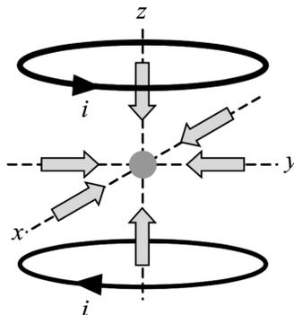
The two current loops create a magnetic quadrupole field near the origin, where the magnetic field vanishes.
