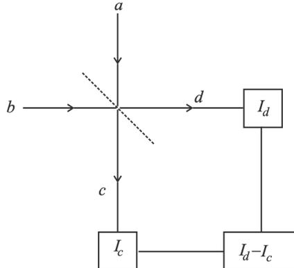
Here, mode  $a$  contains a state to be measured, while mode  $b$  contains a strong coherent classical field of amplitude  $\beta$ . The setup is known as homodyne detection because these two fields are produced by the same source and thus have the same frequency.
