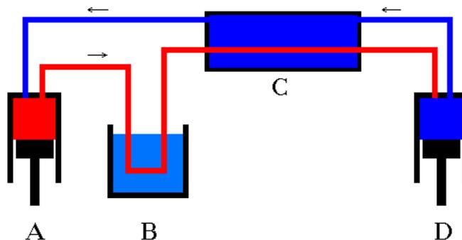
First, a gas is compressed by a piston and thereby heated (A). Most of the heat is removed by a cooler (B), and then further cooled by a countercurrent heat exchanger (C). Finally, the gas is again cooled by expansion against a piston at (D). The net effect is that the gas ends up cooler than it started.
