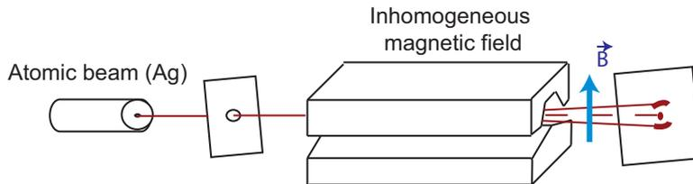
**Abbildung 10.1.** Stern Gerlach experiment. An atomic beam splits in two parts in an inhomogeneous magnetic field along the  $z$ -axis which is parallel to the average magnetic field direction.
