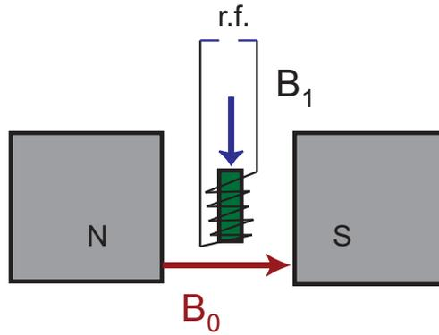
**Abbildung 10.11.** NMR setup; The sample (green) is positioned in a homogeneous and constant magnetic field  $B_0$ ; perpendicular to  $B_0$  an additional magnetic field  $B_1$  is generated with a high frequency generator (r.f.); absorption of the r.f. field result in nuclear spin flips and in reducing the power of the induction coil, which is the measured quantity.
