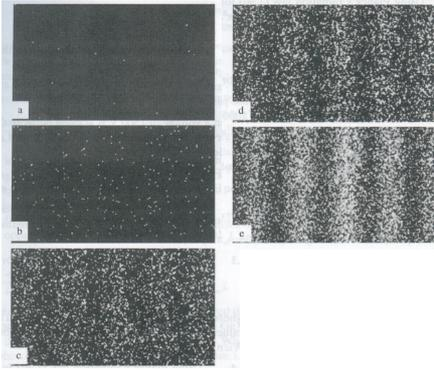
**Abbildung 2.2.** Build up of an interference pattern by accumulating single electrons in a two-slit experiment of Tonomura et al. (Tonomura, J. et al. *American Journal of Physics* **57**, 117, 1989). Number of electrons: (a) 10; (b) 100; (c) 3000; (d) 20000; (e) 70000.
