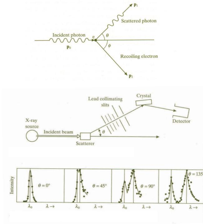
**Abbildung 2.1.** Set up and scattering pattern of photons as a function of wavelength. The data were taken for graphite crystals.
