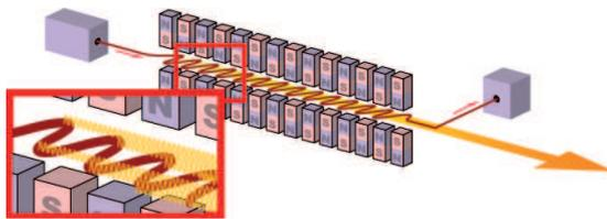
**Abbildung 1.1.** Light generation in a free electron laser. Note, that the lasing process is due to stimulated emission in the direction of the moving electrons.
