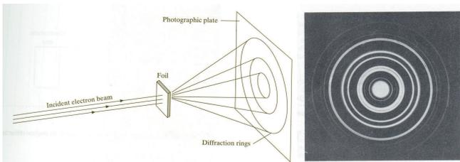
**Abbildung 2.3.** Set up and diffraction pattern of an electron diffraction experiment on crystal powder (from L. Germer).
