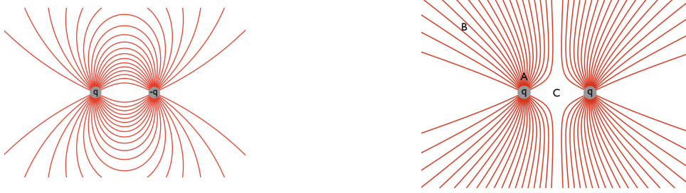
Fig. 2.5 left Field lines for two equal and opposite charges, an “electric dipole.” The number of lines leaving the positive charge equals the number terminating at the negative charge right Field lines for two positive charges of equal magnitude. Can you rank the relative field strengths at points A, B, and C? 13
