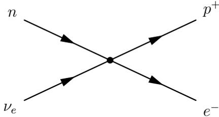
The “Feynman diagram” of the 4-point interaction “neutrino scattering on a neutron” has the following matrix element:
