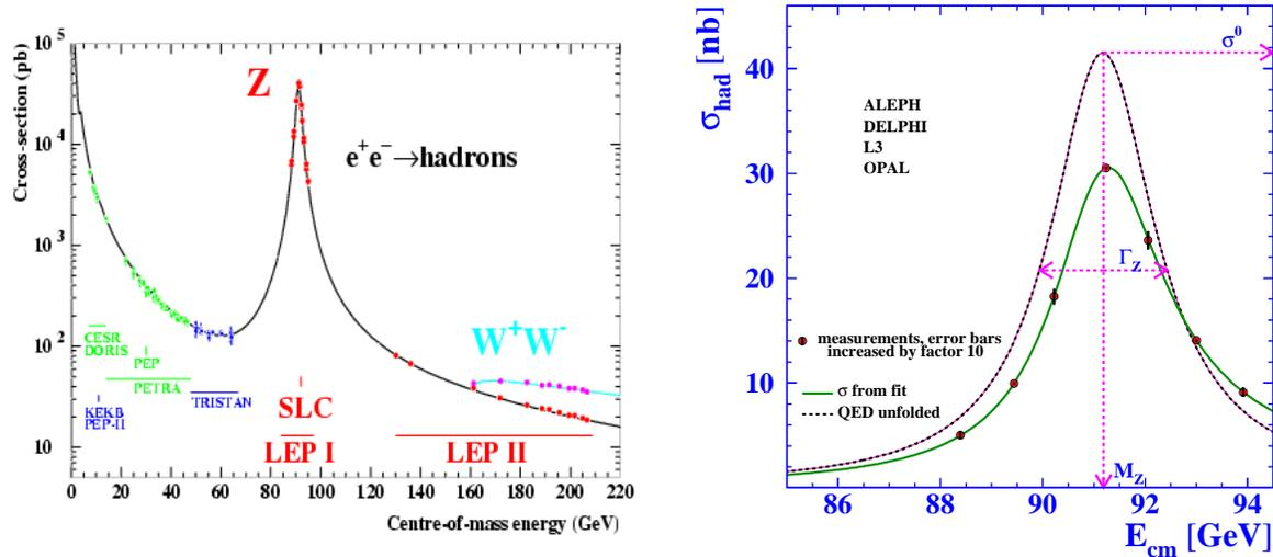
Figure 12.4: *left*: The  $Z$ -lineshape as a function of  $\sqrt{s}$ . *right*: The Lineshape parameters for the lowest order calculations and including higher order corrections.
