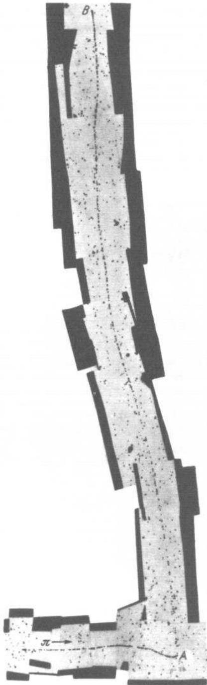
**Figure 1.4** One of Powell's earliest pictures showing the track of a pion in a photographic emulsion exposed to cosmic rays at high altitude. The pion (entering from the left) decays into a muon and a neutrino (the latter is electrically neutral, and leaves no track). Reprinted by permission from C. F. Powell, P. H. Fowler, and D. H. Perkins, *The Study of Elementary Particles by the Photographic Method* (New York: Pergamon, 1959). First published in *Nature* **159**, 694 (1947).
