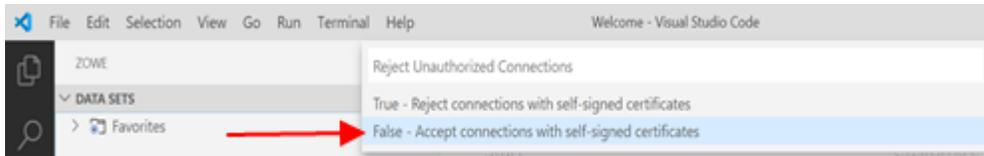
Figure 13. Accept connections with self-signed certifications
