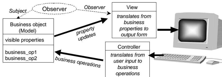
**Figure 41** MODEL-VIEW-CONTROLLER instantiates OBSERVER.
