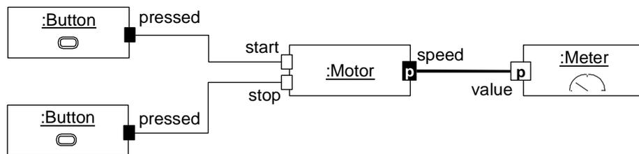
**Figure 43** Component ports and event and property connectors.
