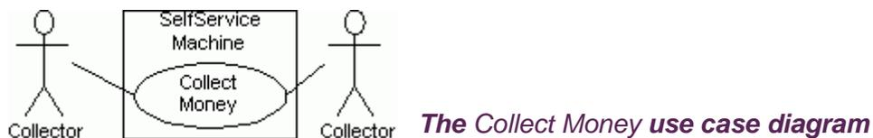
The steps of un-securing the machine, front opening, closing and securing the machine are the same that supplier and collector must do. This is a good place to include a use case. Let's combine the "un-secure" and "pull open" steps into use case called "Expose the inside" and the "close machine" and "secure" with use case "Un-expose the inside". By including a use case Restock and Collect use cases may look as this:
