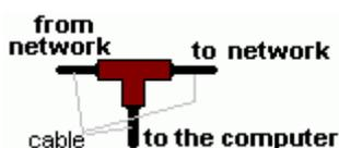
Computers connect to a network cable via connection devices called T-connectors, or sometimes vampire-taps are used. T-connector has three connecting points. Its form is similar with T-letter and that's why their name came from. Network cable goes from one end-point to the other end-point of the connector, and the third end-point has a cable going to the
