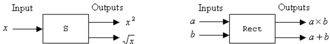
**Figure 10.2:** The box notations of one-input and two-output subroutine `s`, and two-input and two-output subroutine `Rect`.
