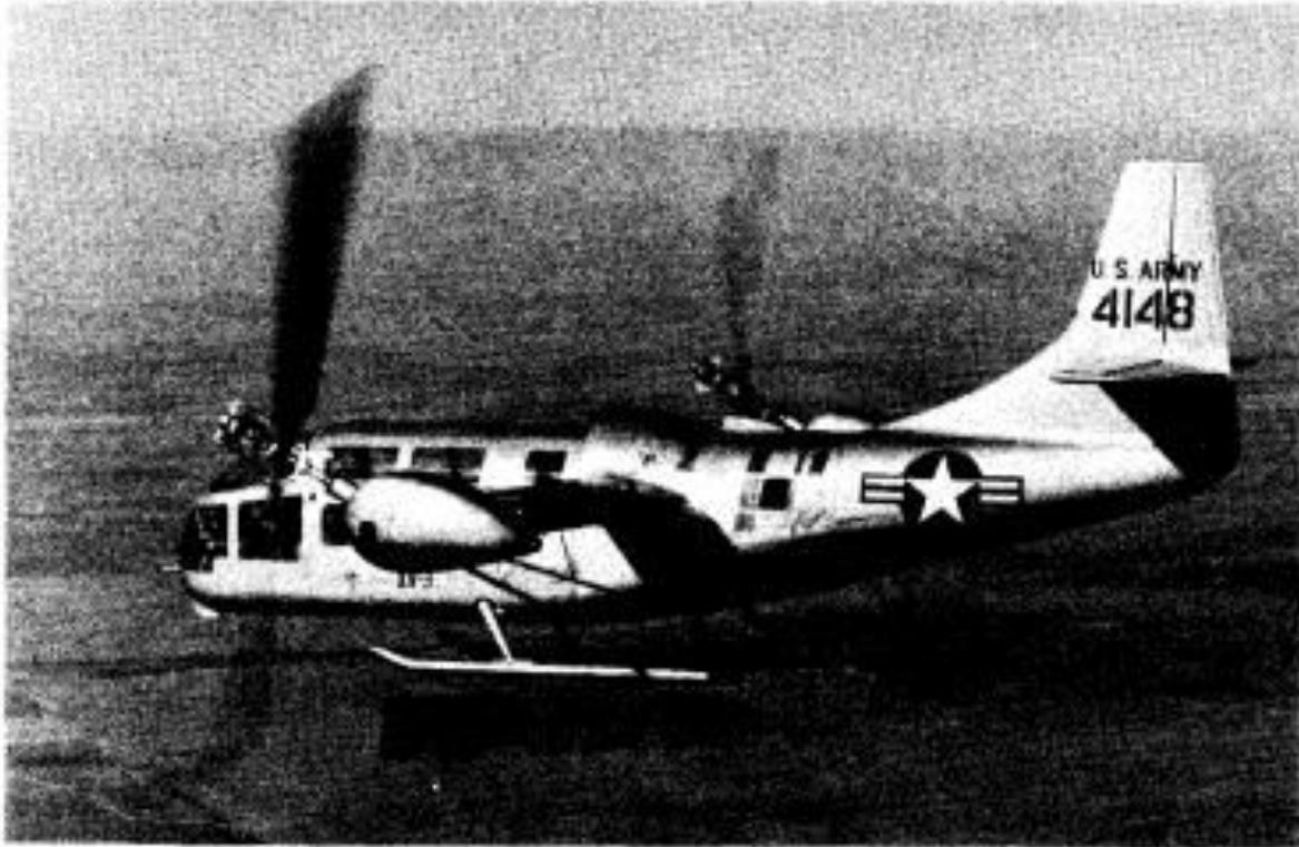
Figure 41. The Bell XV-3, a tilting-rotor VTOL aircraft. (Textron's Bell Helicopter Co.)
