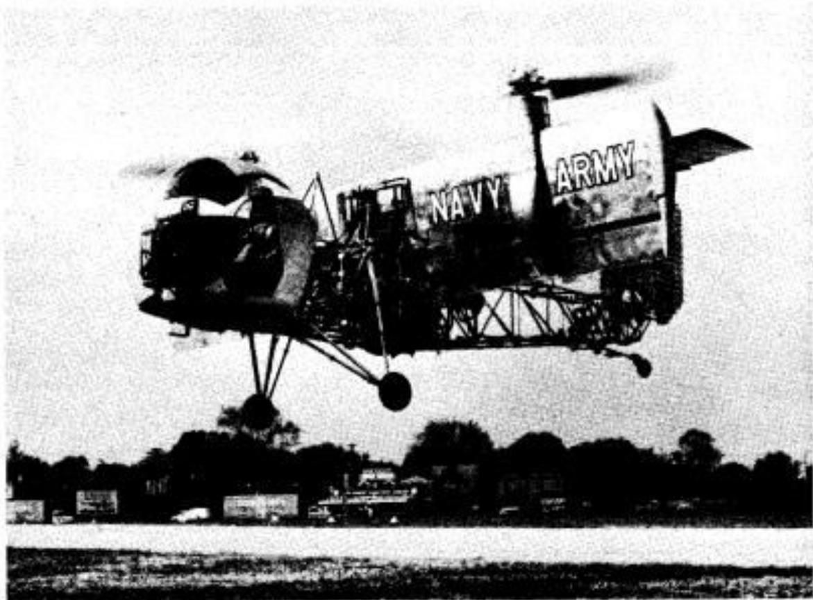
Figure 40. The first successful tilt- wing aircraft, the Vertol 76. (Vertol Div., The Boeing Co)
