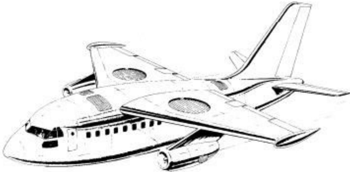
Figure 43. A fan-in-wing aircraft
