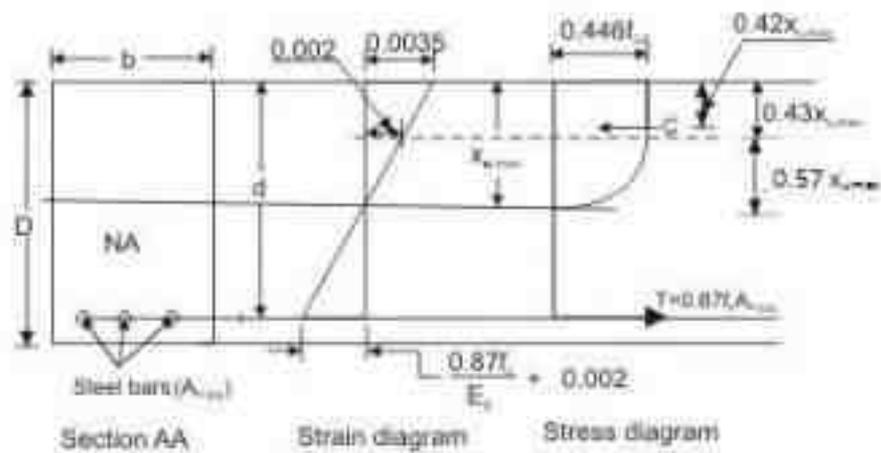
Rectangular beam under flexure when  $x_c = x_{c,max}$
