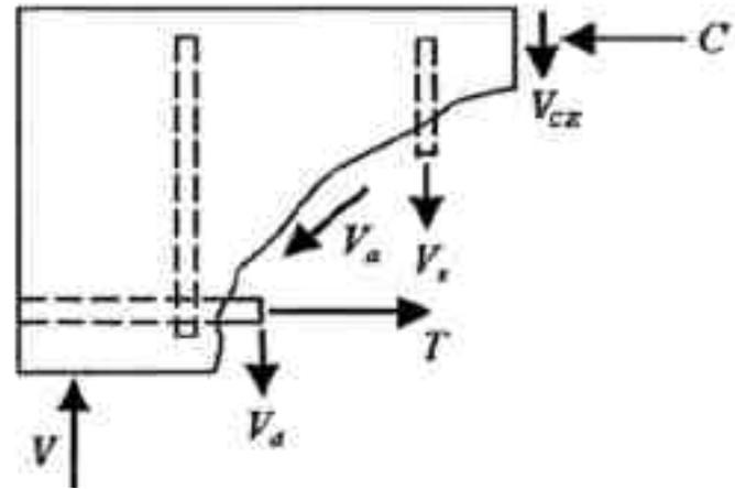
**Mechanism of Shear Transfer in Cracked concrete Beam**
