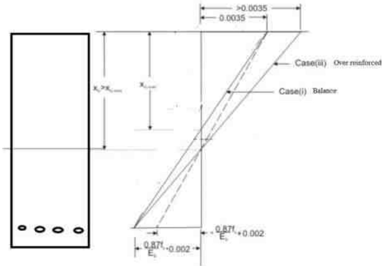
*Strain in concrete reaches its ultimate value first i. e. 0.0035*
