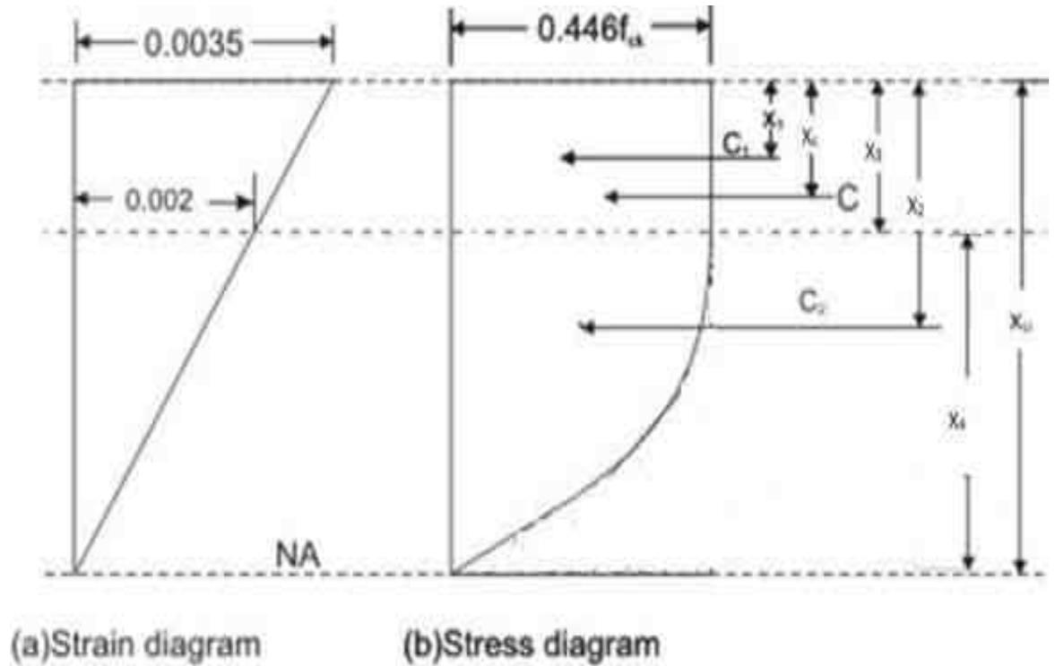
Stress Strain Diagram above the Neutral Axis
