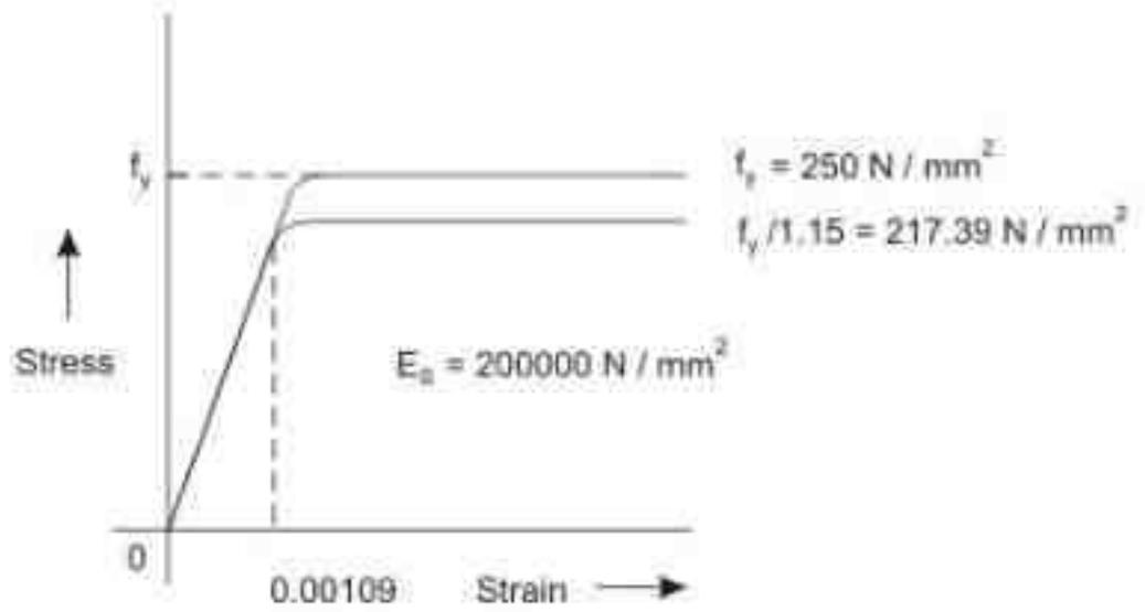
Stress - Strain curve for mild steel (idealised)
