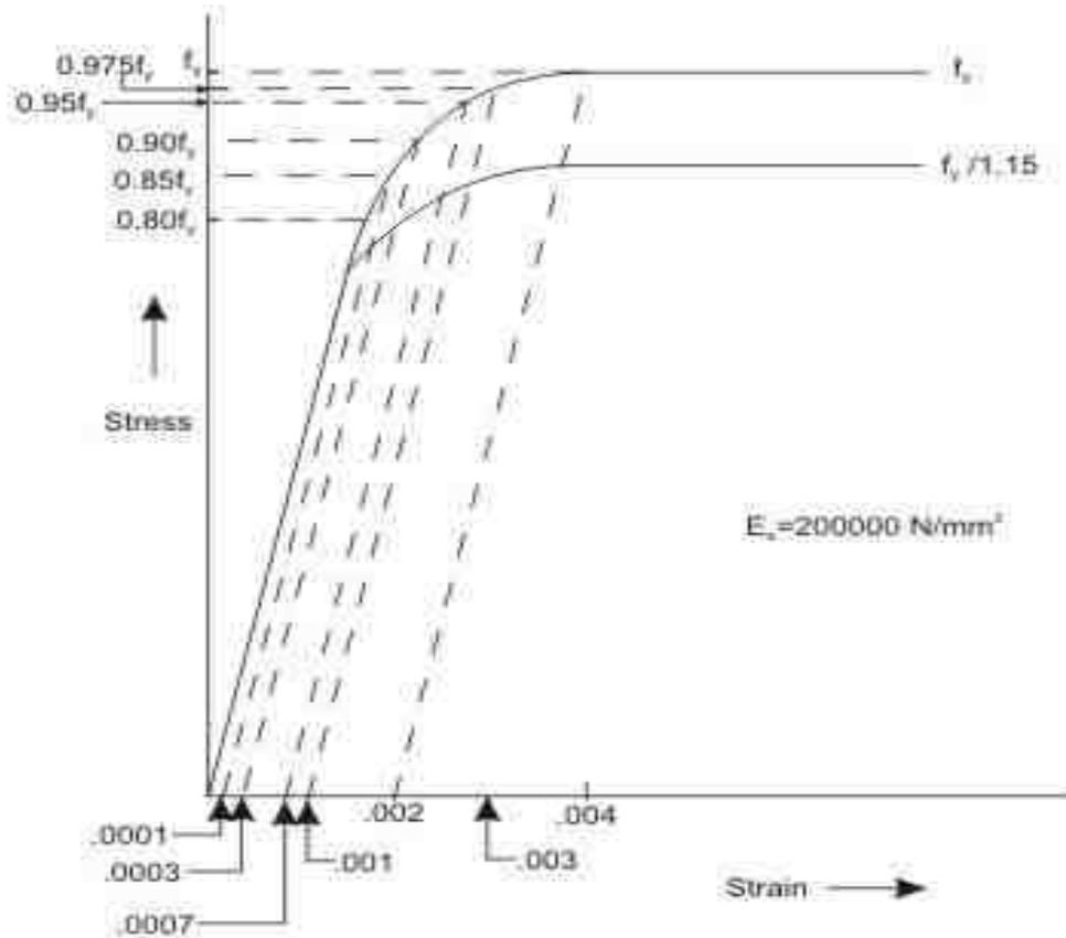
**Stress-Strain Curve for cold worked deformed bar**
