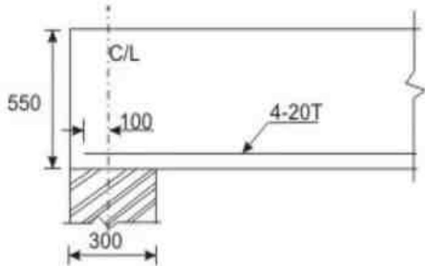
Determine the anchorage length of 4-20T reinforcing bars going into the support of the simply supported beam shown in Fig. The factored shear force  $V_u = 280 \text{ kN}$ , width of the column support = 300 mm. Use M 20 concrete and Fe 415 steel.
