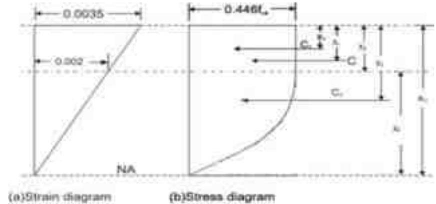
Stress Strain Diagram above the Neutral Axis
