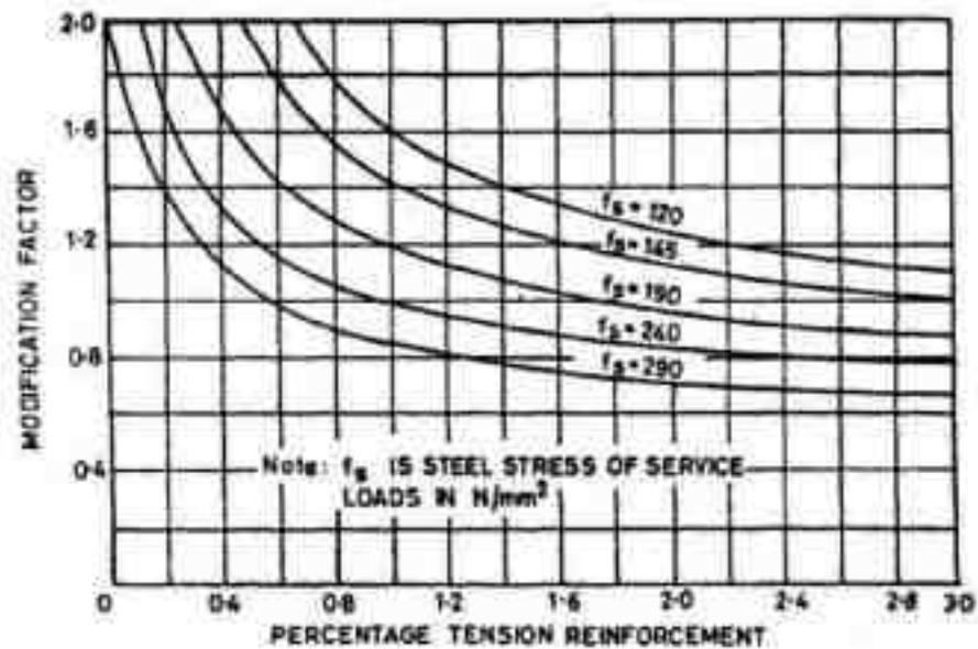
$$f_s = 0.58 f_t \frac{\text{Area of cross-section of steel required}}{\text{Area of cross-section of steel provided}}$$
