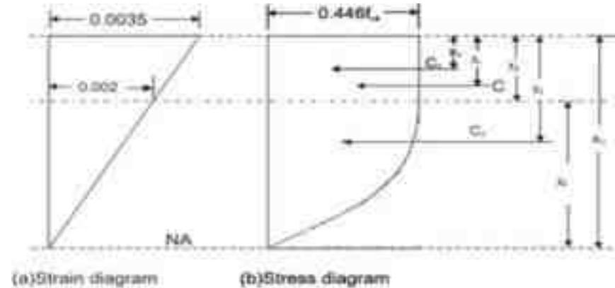
Stress Strain Diagram above the Neutral Axis
