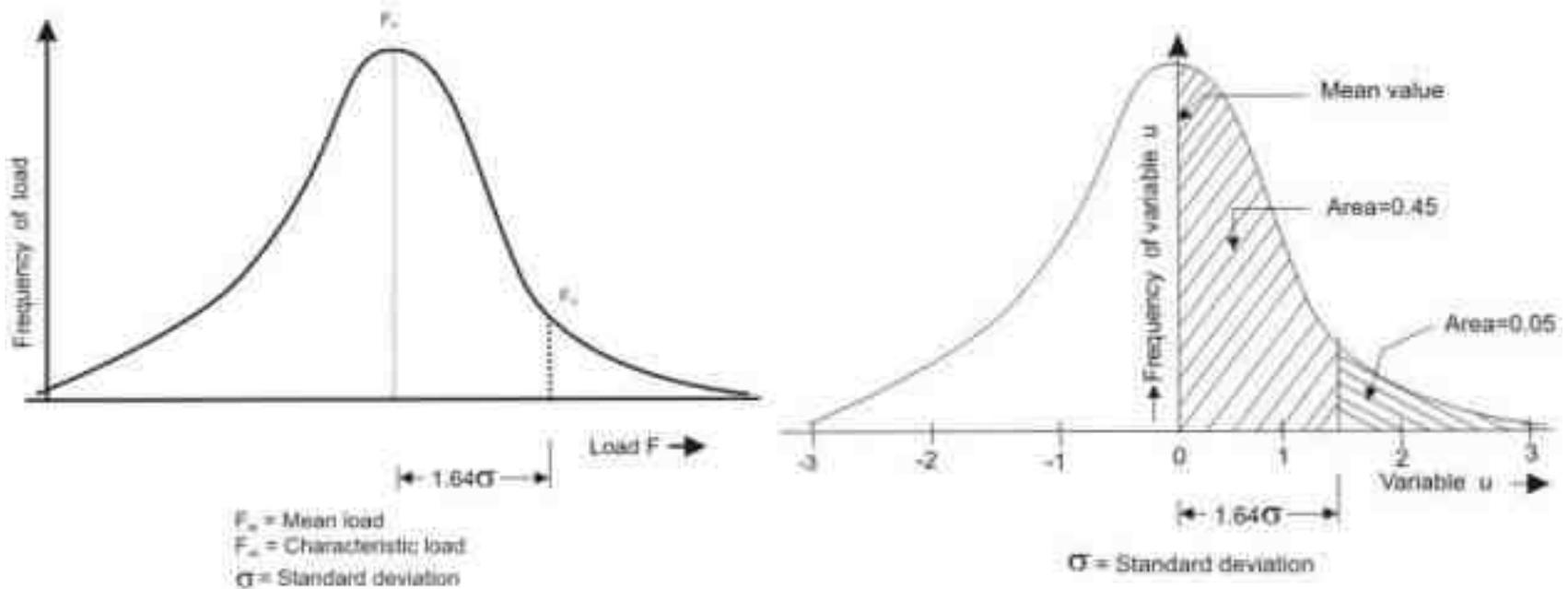
Characteristic load = Average/mean load +  $K$  ( $\sigma$ =standard deviation for load)
