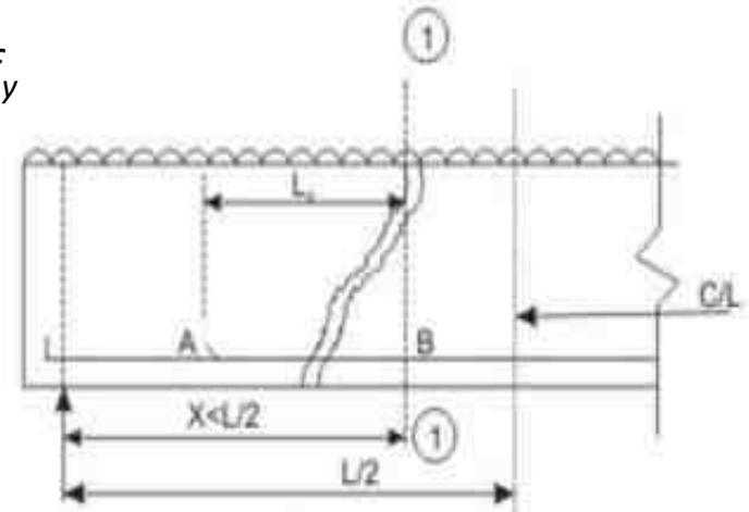
(a): Beam showing  $L_d$  of a bar
