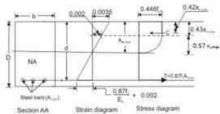
Rectangular beam under flexure when  $x_u = x_{u,limit}$
