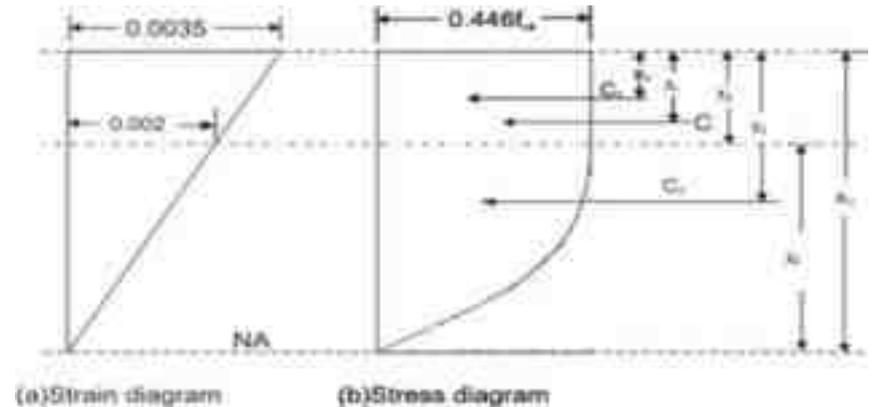
Stress Strain Diagram above the Neutral Axis
