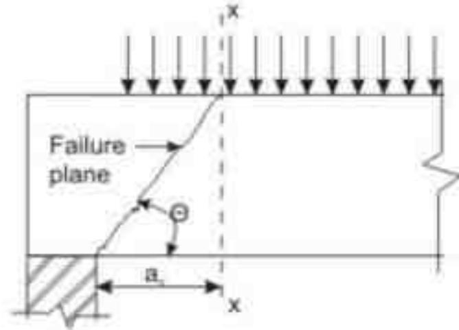
Account may be taken of the enhancement in any situation where the section considered is closer to the face of a support or concentrated load than twice the effective depth,  $d$ . To be effective, tension reinforcement should extend on each side of the point where it is intersected by a possible failure plane for a distance at least equal to the effective depth, or be provided with an equivalent anchorage.
