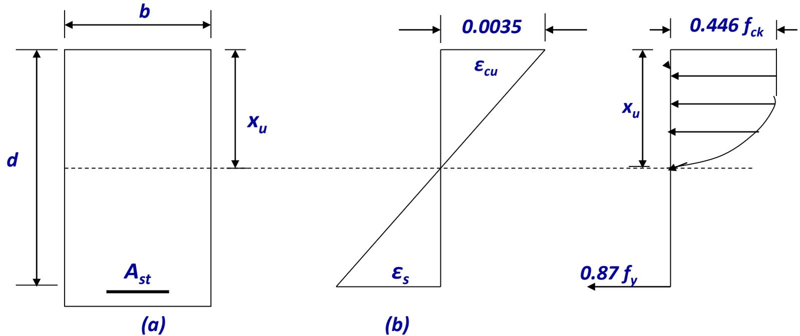
**Strain diagram and Stress blocks:**
