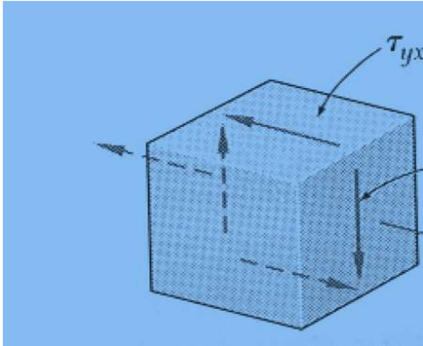
Shear stresses develop on horizontal planes
