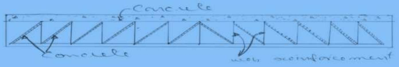
(c) Truss Action in a Reinforced concrete Beam
