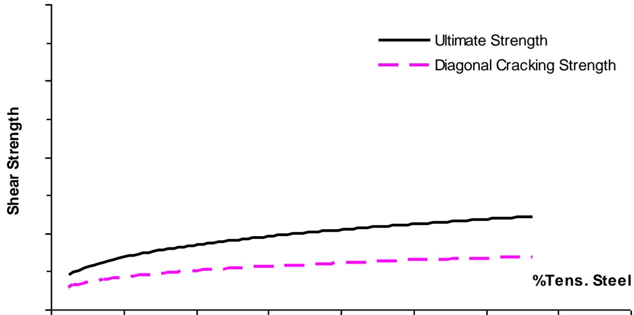
Qualitative variation of ultimate and Diagonal cracking strength with % Tension Steel
