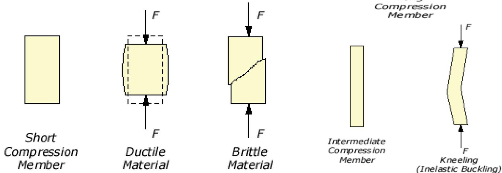
Long members are referred to as columns. Columns, normally fail in buckling.
