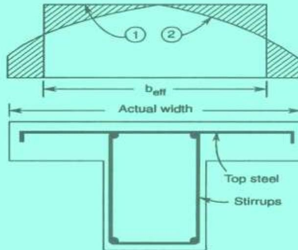
Fig. 8.3 Effective width of T beams: 1. Actual stress distribution in compression flange; 2. Assumed stress distribution in compression flange.
