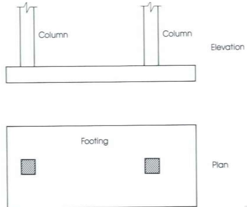
Cantilever or strap footings consist of two single footings connected with a beam or a strap and support two single columns. This type replaces a combined footing and is more economical.
