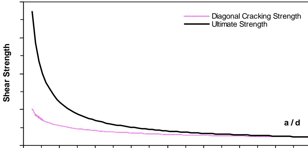
Qualitative variation of ultimate and Diagonal cracking strength with  $a/d$  ratio
