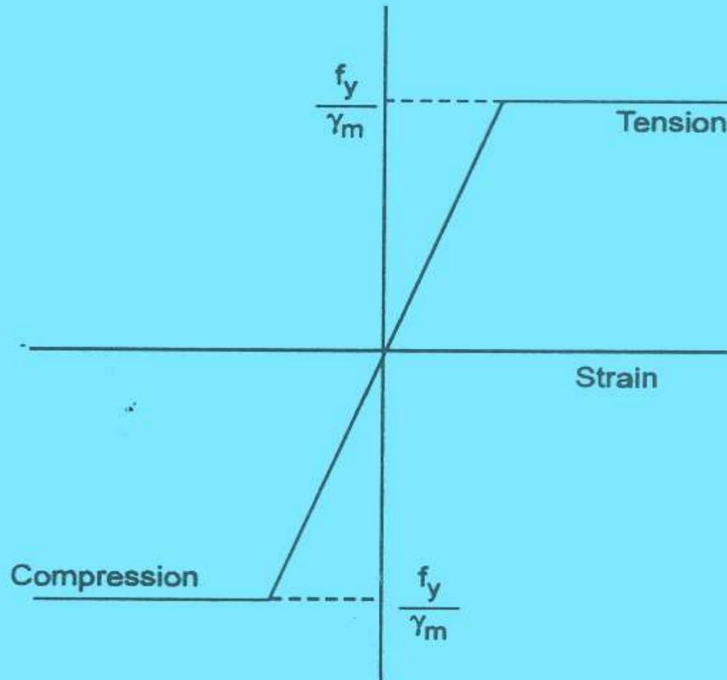
**Fig. 2.5 Stress-strain curve for steel (BS 8110).**
