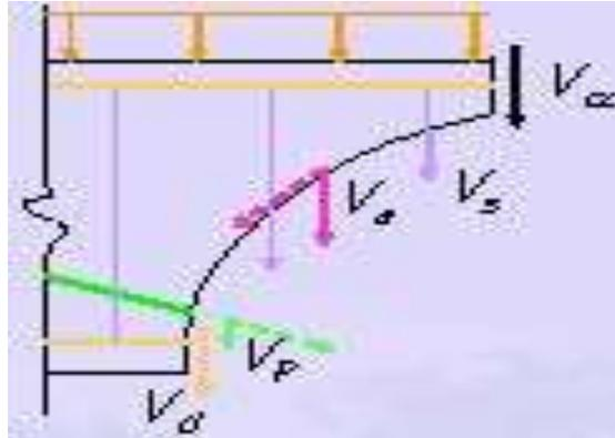
Fig. 8 Internal forces at a flexure shear crack
