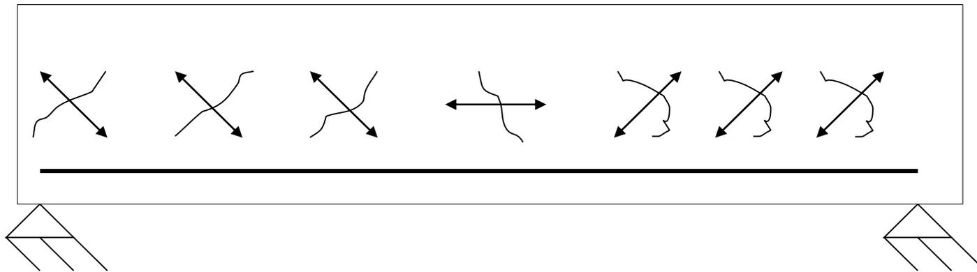
**Direction of potential cracks in a simple beam.**
