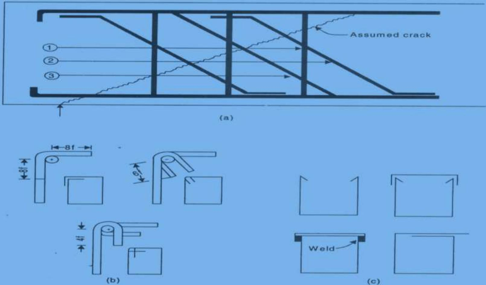
**Fig. 7.4** Types of shear reinforcements in beams: (a) Shear reinforcements—(1) system of vertical stirrups; (2) system of inclined stirrups; (3) bent-up tension bar; (b) Detailing of ends of conventional types of stirrups; (c) Some special shapes of stirrups.
