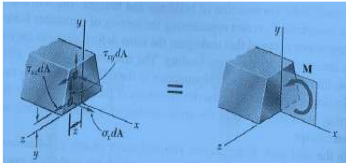
**Stresses developed in beam under pure bending moment**
