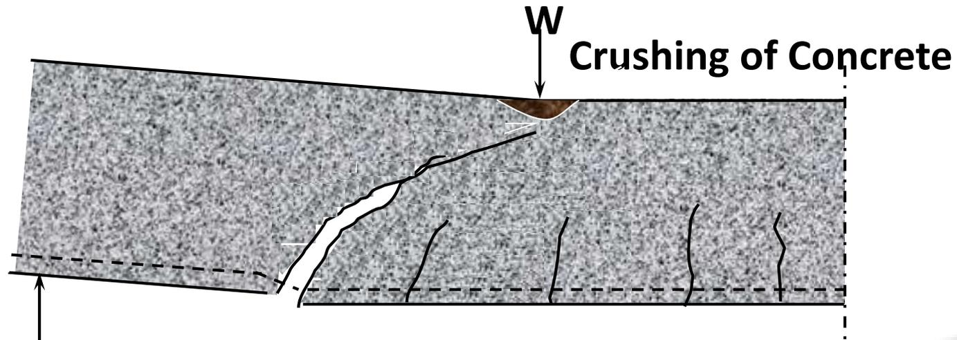
**Crushing of Concrete**
