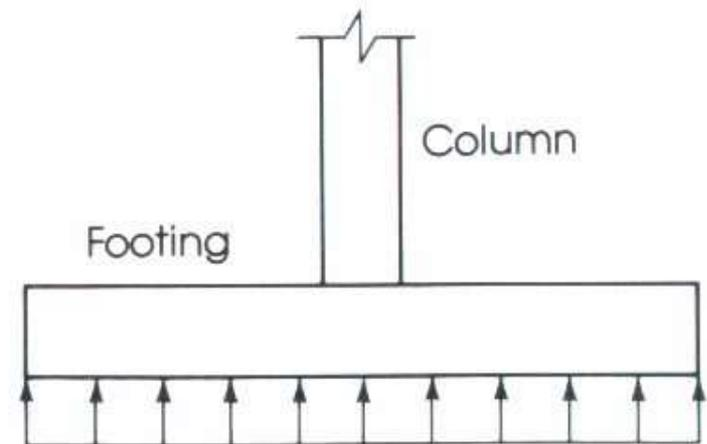
However the actual distribution of the soil is not uniform, but depends on many factors especially the composition of the soil and degree of flexibility of the footing.
