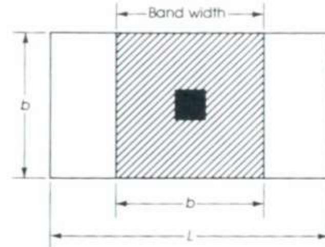
$$\frac{\text{Reinforcement in band width}}{\text{Total reinforcement in short direction}} = \frac{2}{\beta + 1}$$
