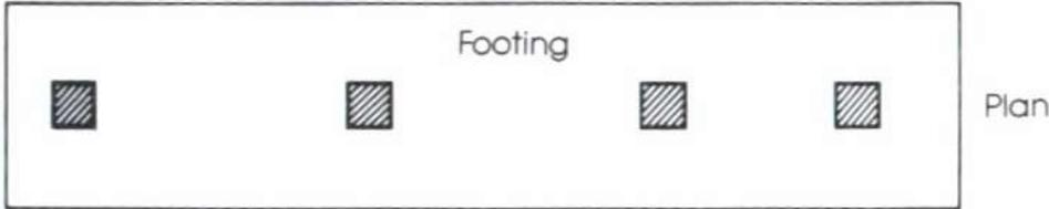
Rafted or mat foundation consists of one footing usually placed under the entire building area. They are used, when soil bearing capacity is low, column loads are heavy single footings cannot be used, piles are not used and differential settlement must be reduced.
