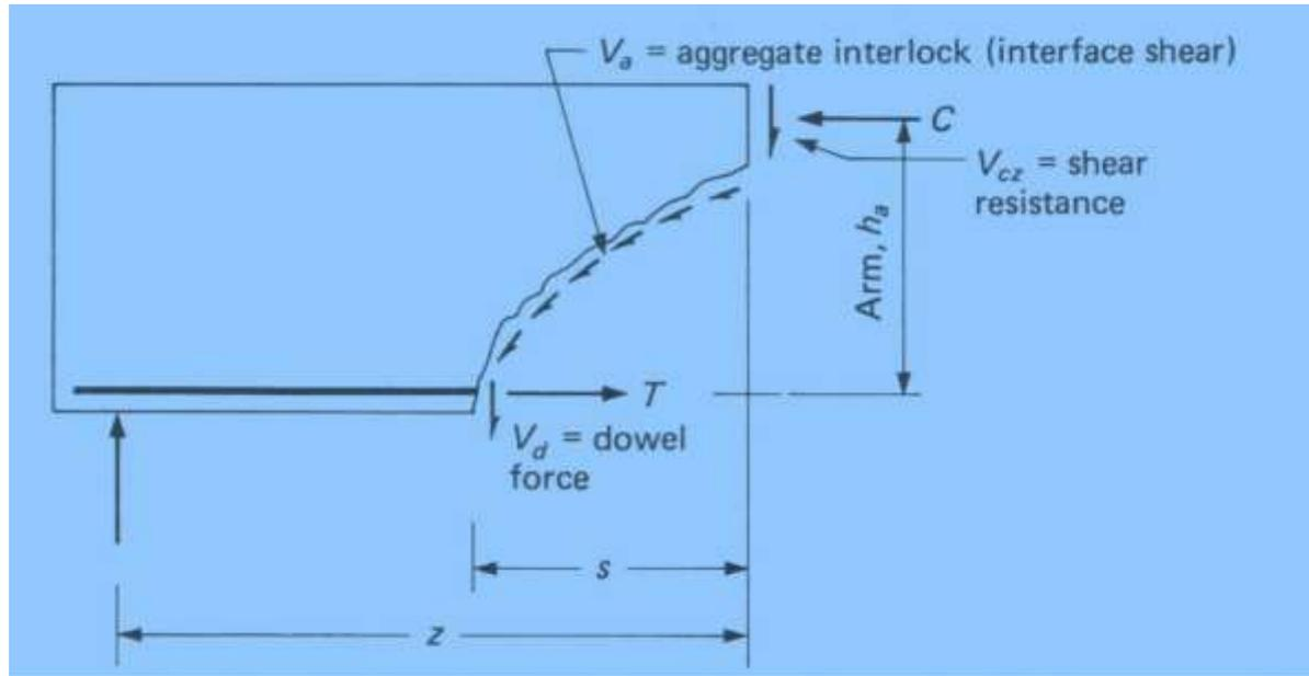
$v_{cz}$  = Shear in compression zone (20-40%)
