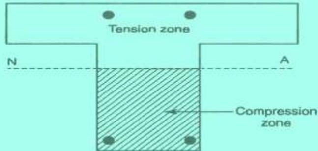
Fig. 8.2 Flanged beams over supports with negative moments.
