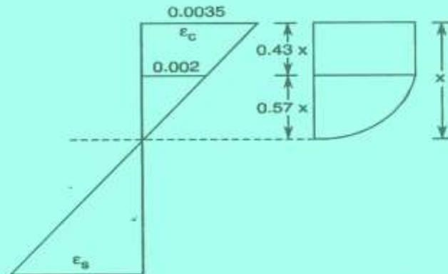
Fig. 8.5 Compression stress block in T beams.
