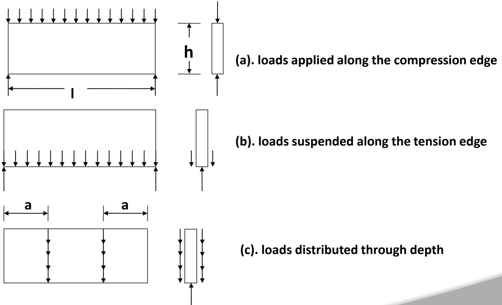
**Fig. Placements of loads on deep beams.**
