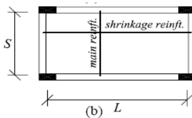
**One way slab; (a) classification; (b) reinforcement**
