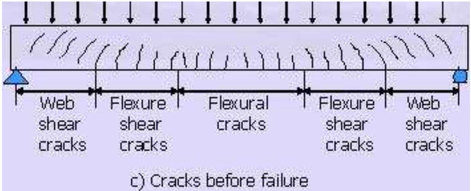
c) Cracks before failure
