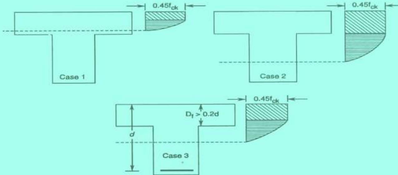
Fig. 8.4 Three possible positions of neutral axis in T beams.
