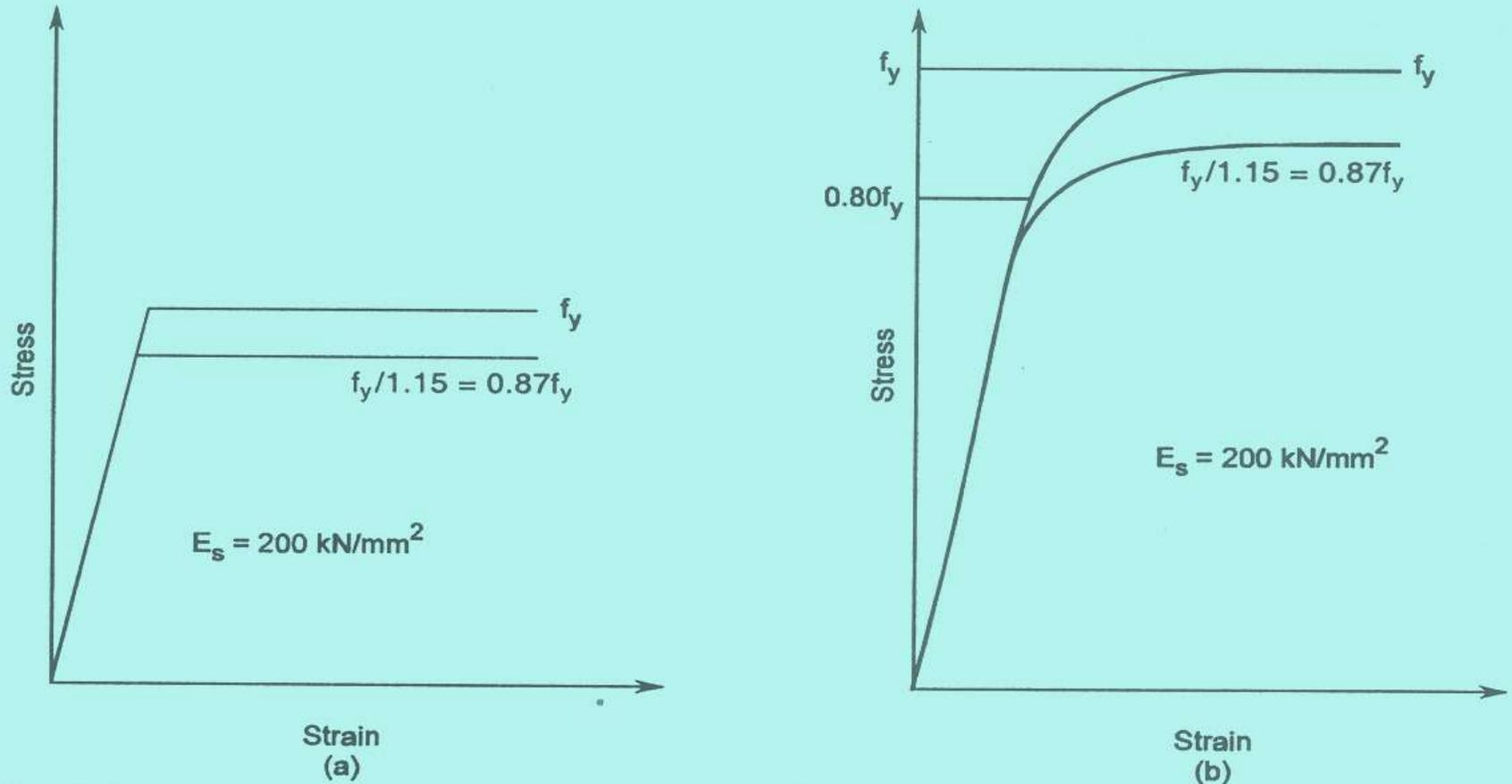
**Fig. 2.4 Stress-strain curves for steel reinforcements: (a) Mild steel; and (b) Cold worked bars. (Fig. 23 of IS 456–2000)**
