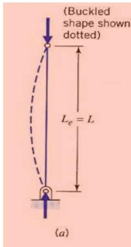
Pinned-Pinned, or rounded-rounded
