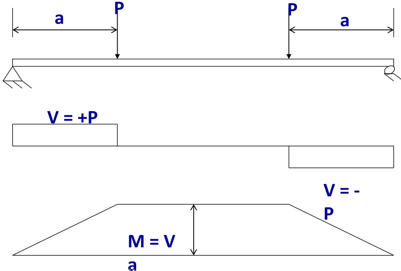
**Basic Definition of Shear span,  $a$**
