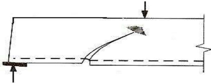
Fig. 10 Shear compression failure
