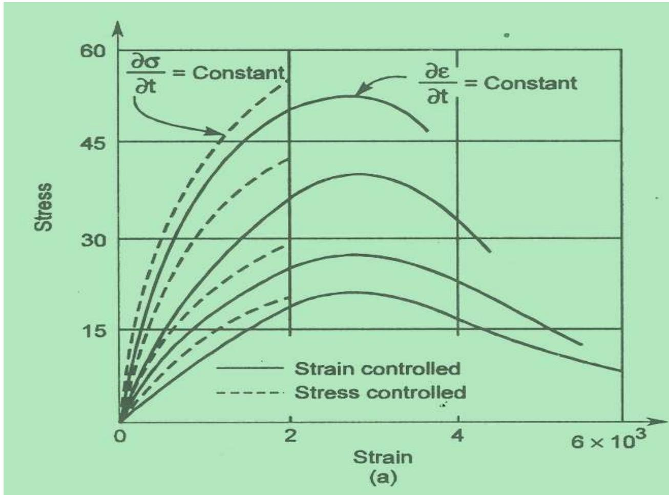
**Design stress-strain curves for concrete in compression**
