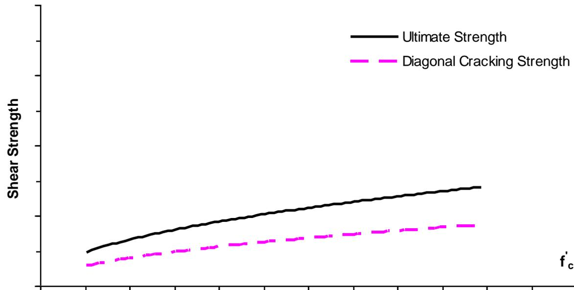
Qualitative variation of ultimate and Diagonal cracking strength with Compressive Strength of Concrete
