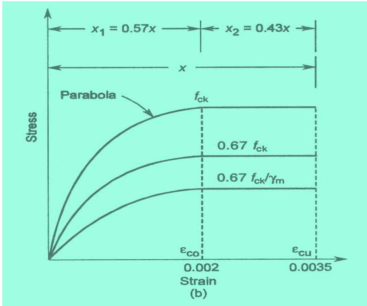
**Design stress-strain curves for concrete in compression**
