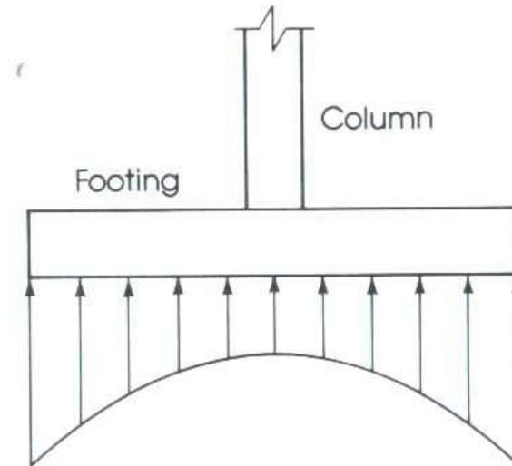
Footings must be designed to carry the column loads and transmit them to the soil safely while satisfying code limitations.
