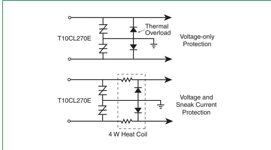
Figure 6.65 SIDACtor Cell Primary Protection
