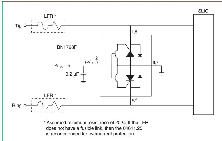
Figure 6.53 SLIC Protection with Series R and 8-pin *Battrax*
