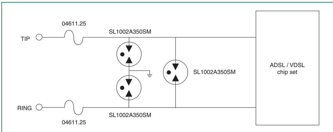
Figure 6.11 Single Port Delta Solution Providing Metallic and Longitudinal Protection
