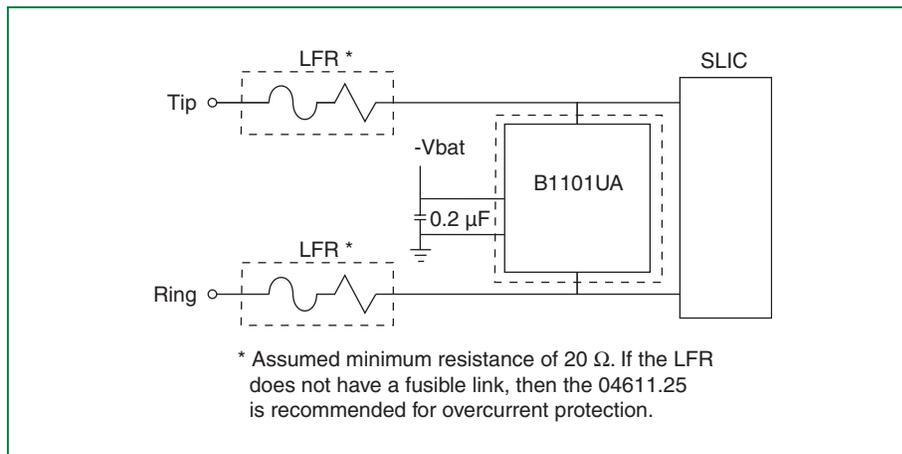
Figure 6.52 SLIC Protection with Series R and *Batrax*
