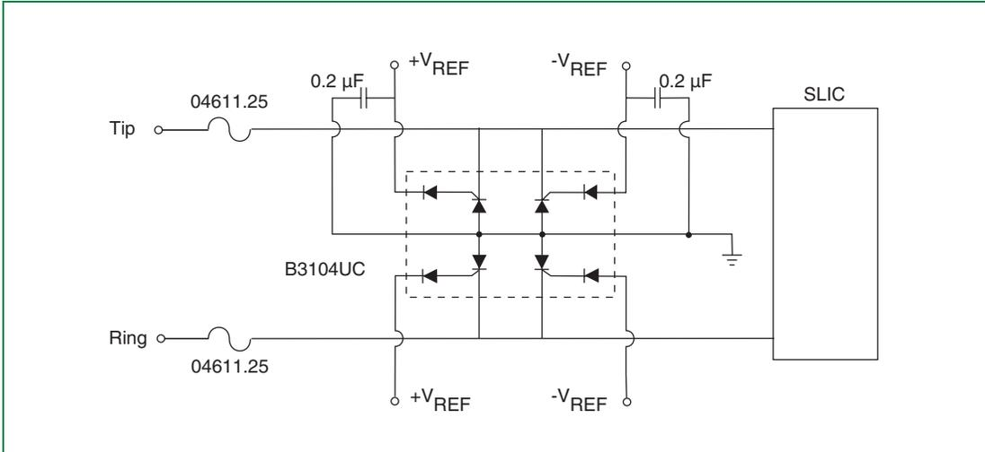
Figure 6.49 SLIC Protection with a *Battrax* Dual Positive/Negative Device
