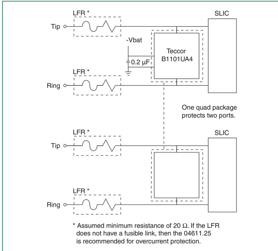
Figure 6.54 SLIC Protection with Series R and Quad *Batrax*
