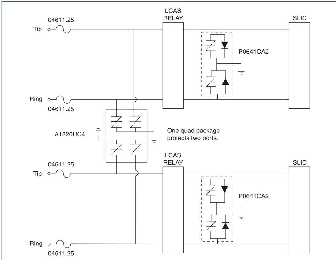
Figure 6.41 SLIC Protection with *TeleLink* Multiport
