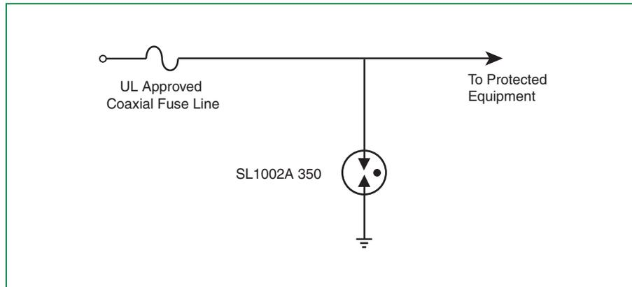
Figure 6.62 Gas Plasma Arrester CATV Station Protection
