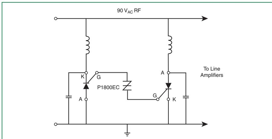
Figure 6.60 CATV Amplifier Protection
