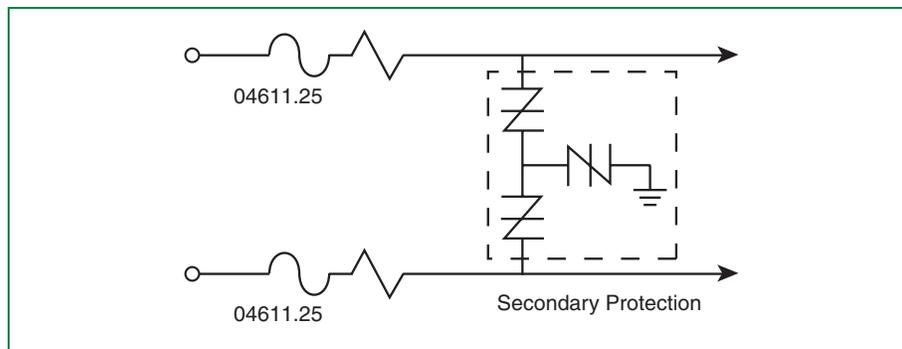
Figure 6.29 Coordination Solution with Resistor
