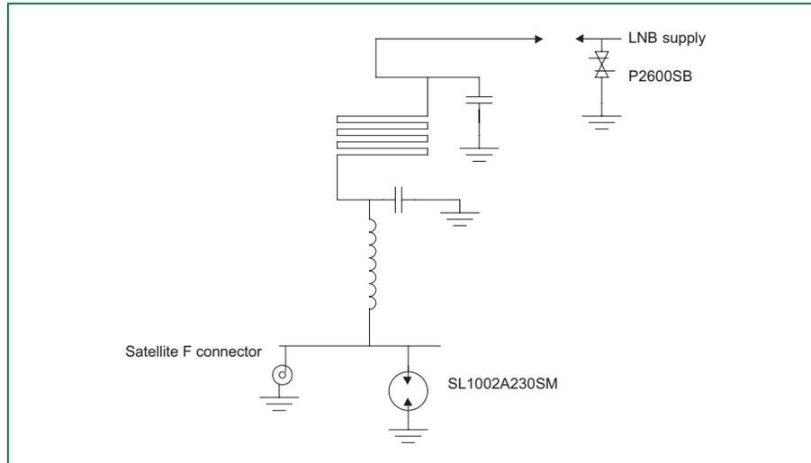
Figure 6.8 Satellite Receiver Protection
