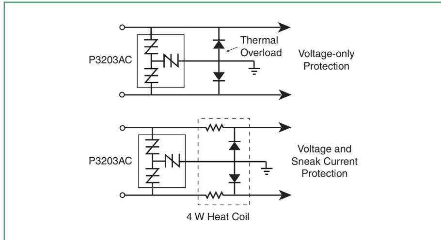
Figure 6.66 Balanced SIDACtor Primary Protection
