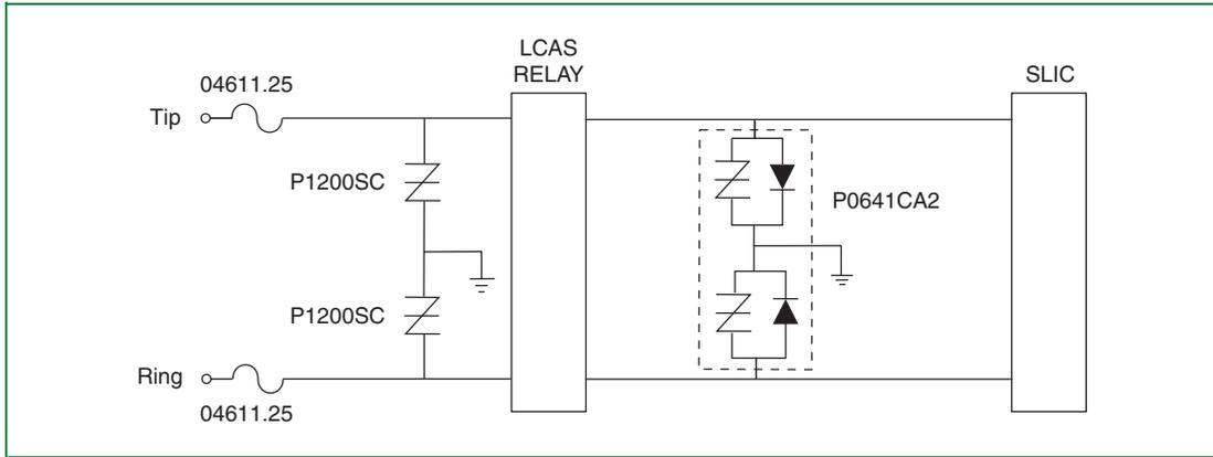
Figure 6.43 SLIC Protection with Single Port Discrete
