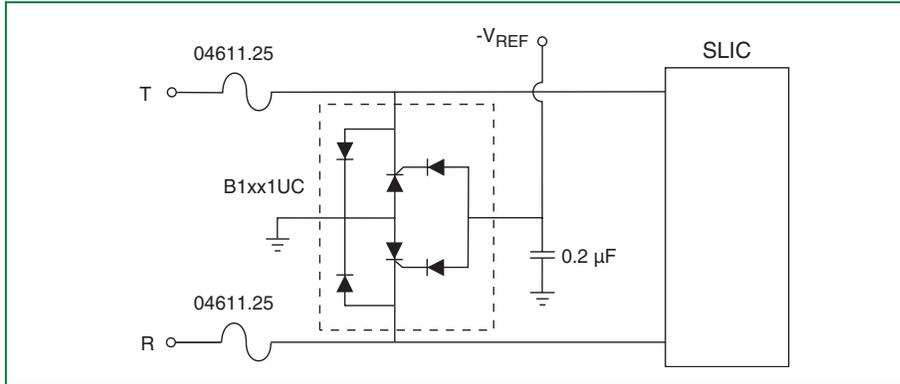
Figure 6.47 SLIC Protection with a Dual *Battrax* Device
