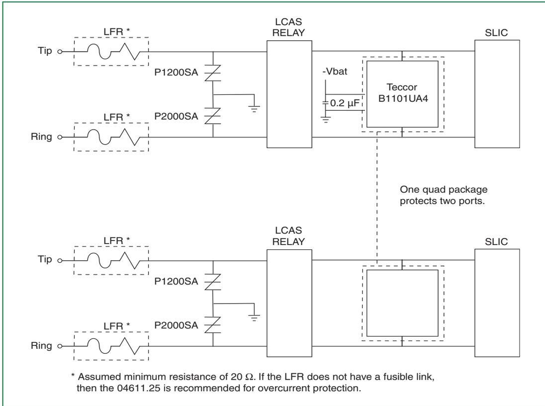
Figure 6.34 SLIC Protection with Quad *Batrax*
