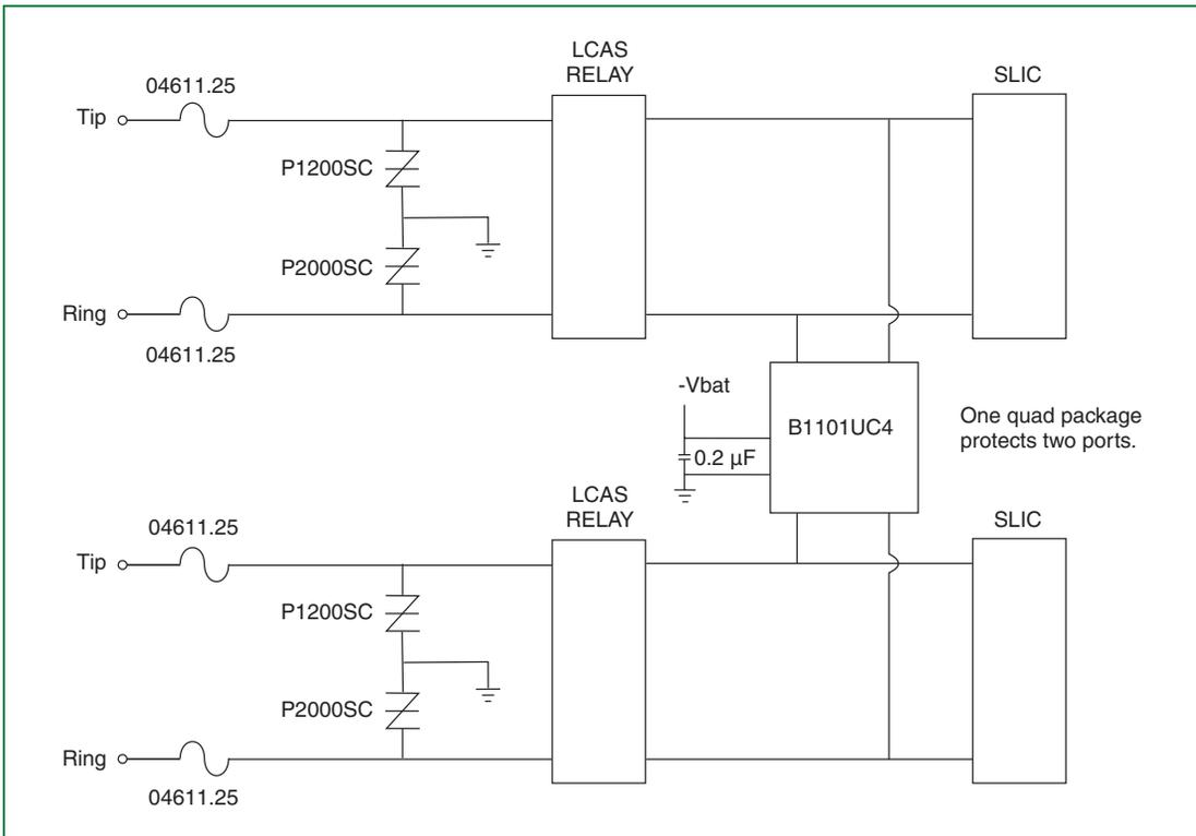
Figure 6.38 SLIC Protection with Quad *Battrax* with Asymmetrical Relay Protection
