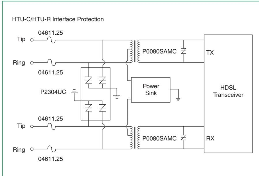
Figure 6.15 HDSL Quad Protection
