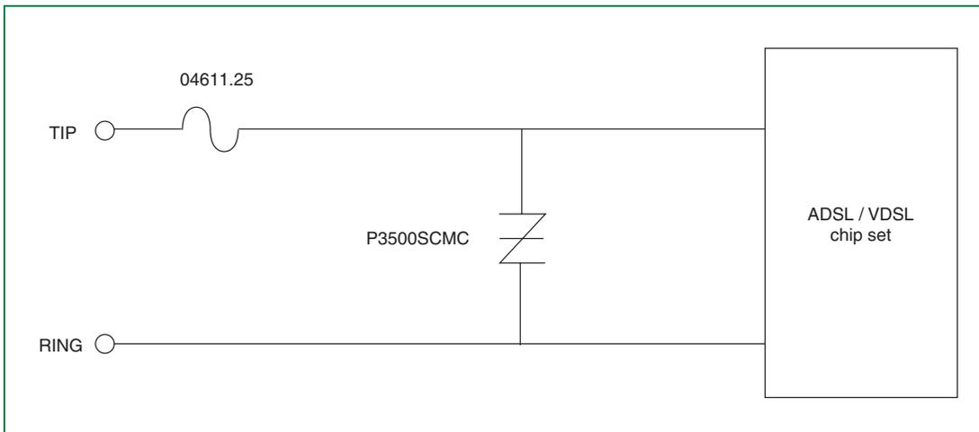
Figure 6.12 *SIDACtor* ADSL / VDSL Protection
