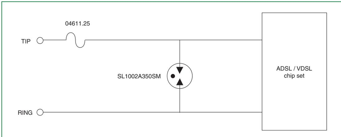
Figure 6.10 Gas Plasma Arrester ADSL Protection
