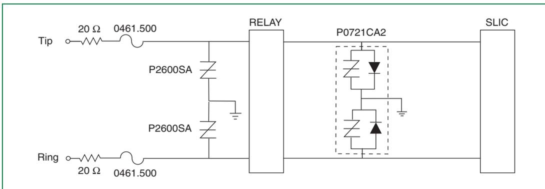
Figure 6.40 SLIC Protection with Fixed Voltage *SIDACTor* Devices
