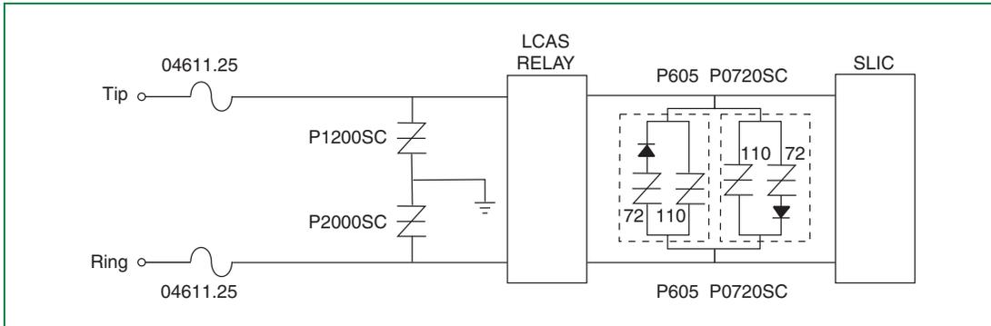
Figure 6.36 SLIC Protection with Asymmetrical Devices
