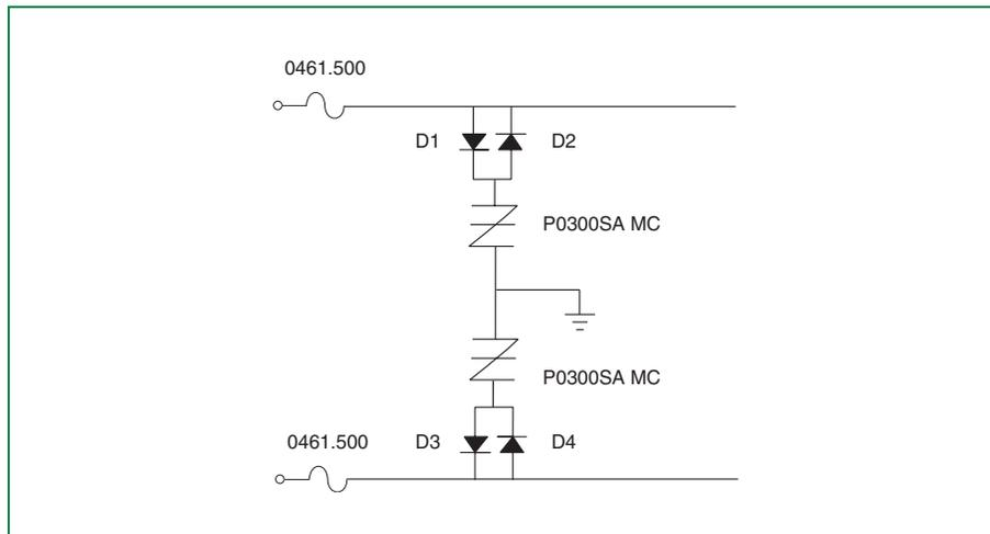
Figure 6.73 10Base-T Metallic and Longitudinal Protection
