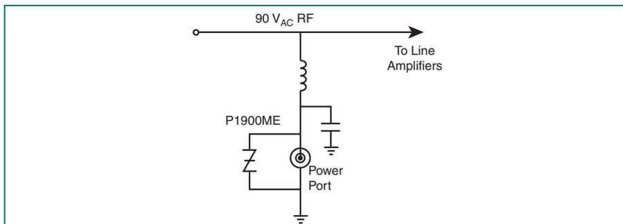
Figure 6.59 SIDACTor CATV Amplifier Protection (incorporated into a power inserter module)
