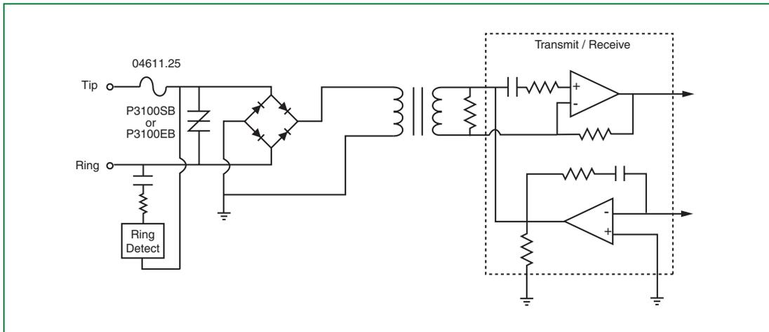
Figure 6.2 Transformer Coupled Tip and Ring Interface
