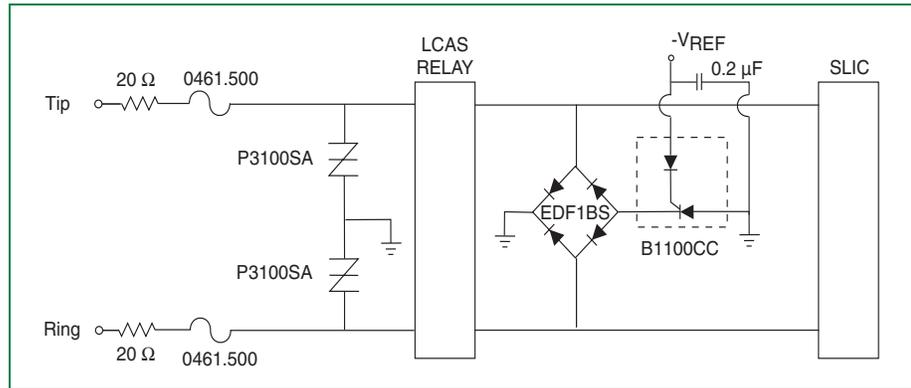
Figure 6.44 SLIC Protection with a Single *Battrax* Device
