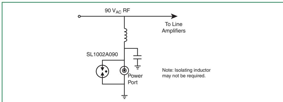
Figure 6.58 Gas Plasma Arrester CATV Amplifier Protection (incorporated into a power inserter module)
