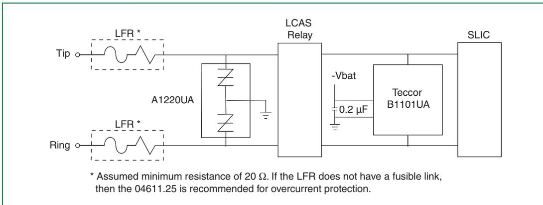
Figure 6.32 SLIC Protection with Limiting Resistance
