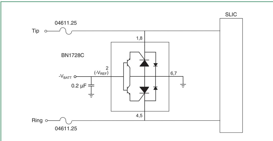
Figure 6.50 SLIC Protection with an 8-pin *Battrax* Dual Positive/Negative Device
