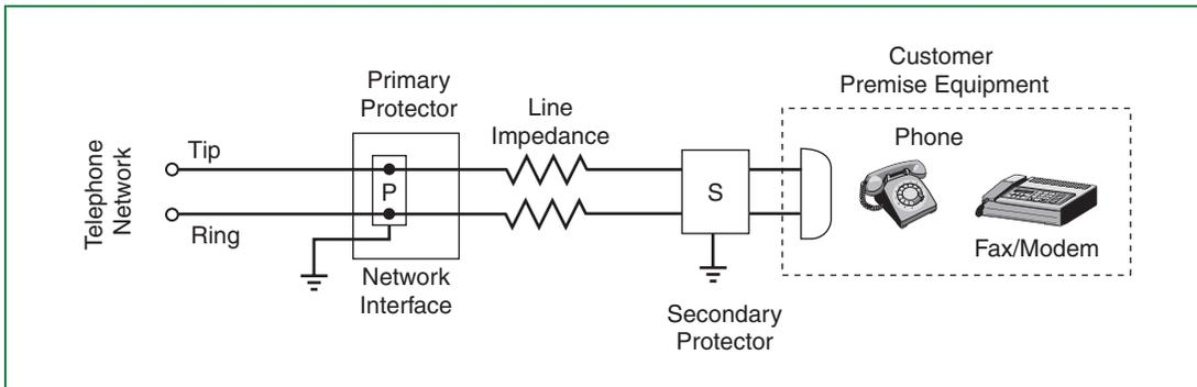
Figure 6.67 CPE Secondary Protection
