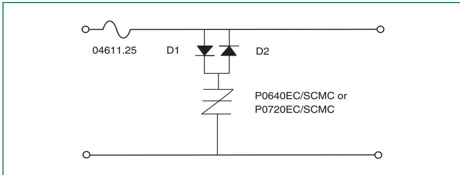
Figure 6.27 T3 Protection—SIDACtor Device and Diodes
