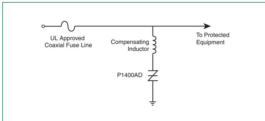
Figure 6.61 *SIDACtor* CATV Station Protection
