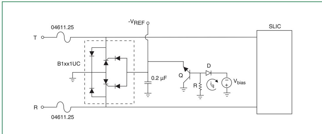
Figure 6.55 *Batrax* Protection Gate Buffer Circuit
