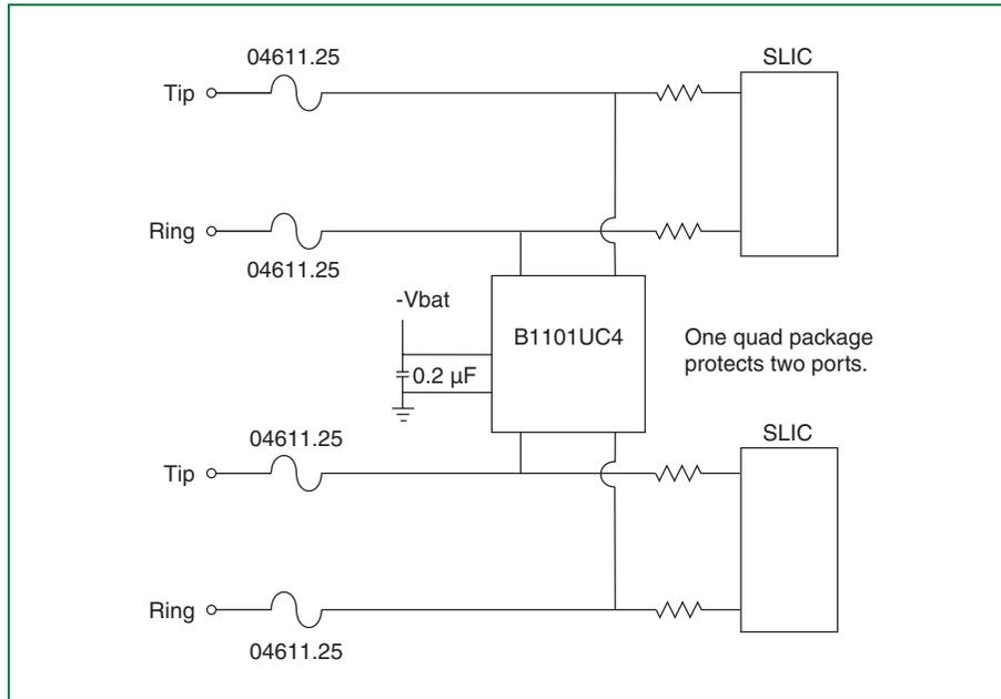
Figure 6.51 SLIC Protection with Quad *Batrax*
