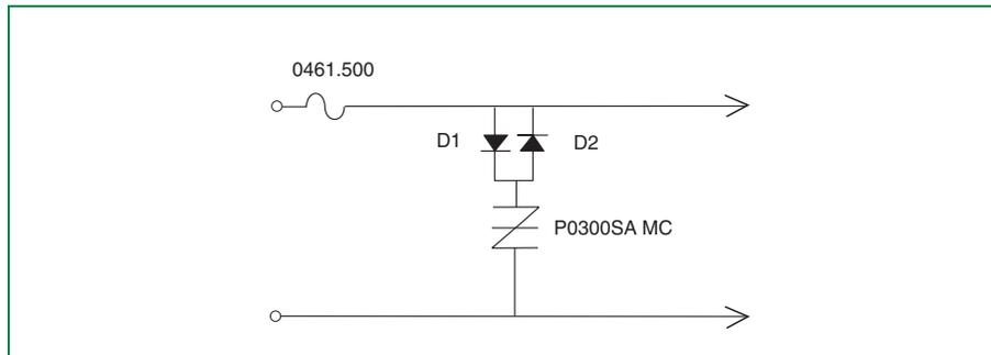
Figure 6.72 10Base-T Metallic-only Protection
