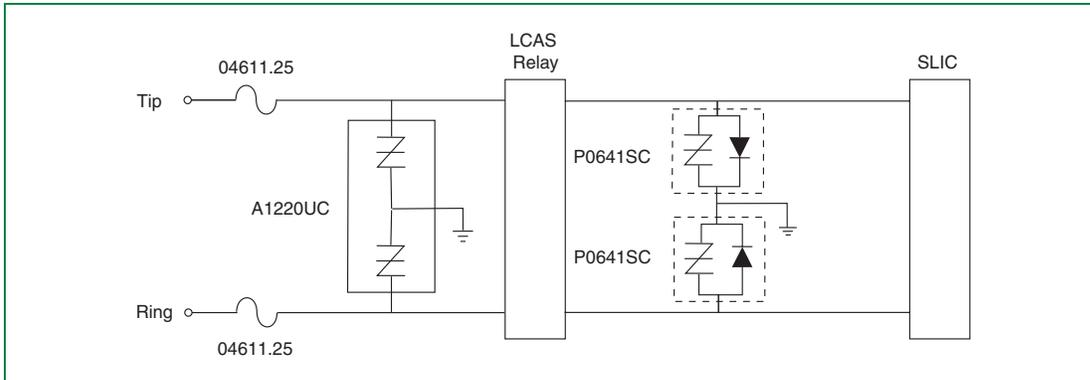
Figure 6.31 SLIC Protection for LCAS
