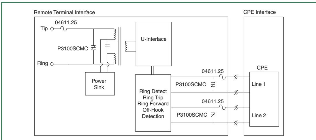
Figure 6.20 Pair Gain RT Protection
