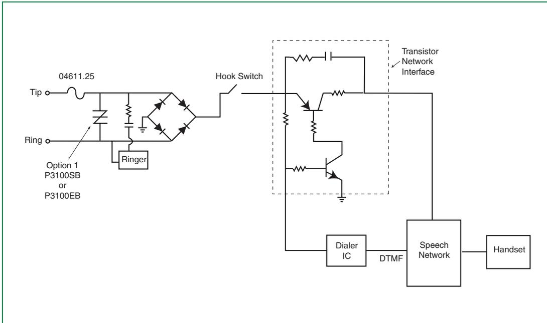
Figure 6.4 CPE Transistor Network Interface—Option 1
