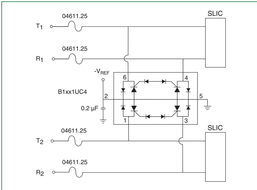
Figure 6.48 SLIC Protection with a Single *Battrax* Quad Negative Device
