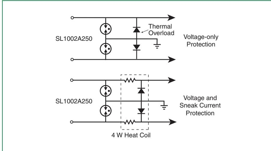
Figure 6.63 Gas Plasma Arrester Primary Protection
