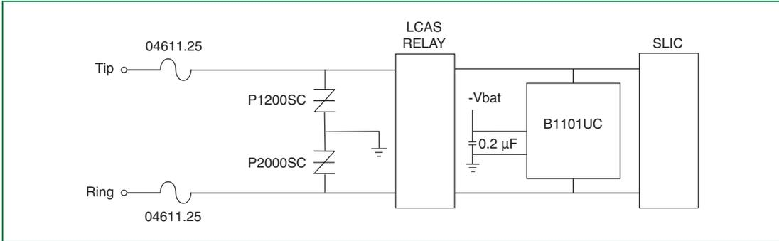
Figure 6.37 SLIC Protection with *Battrax*
