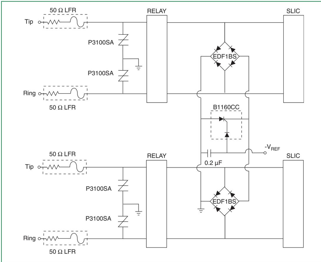
Figure 6.45 SLIC Protection with a Single *Battrax* Device
