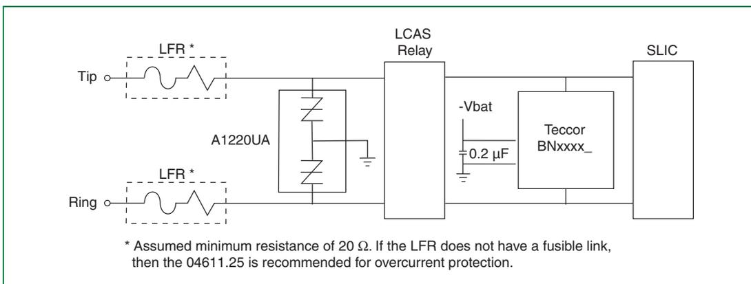
Figure 6.33 SLIC Protection with Limiting Resistance—Buffered *Bat*rax
