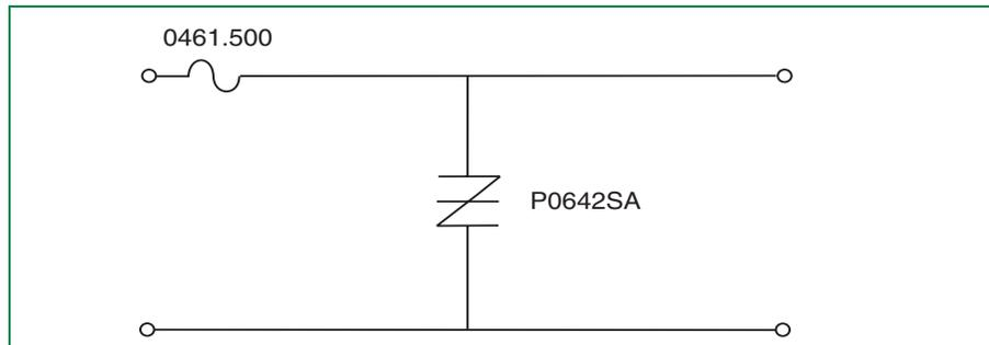
Figure 6.28 T3 Protection—SIDACTor Device
