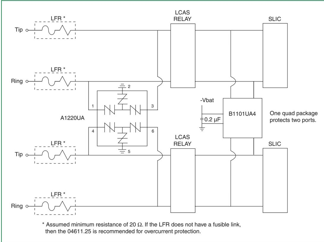
Figure 6.35 SLIC Protection with Quad *Batrax* and Balanced Relay Protector
