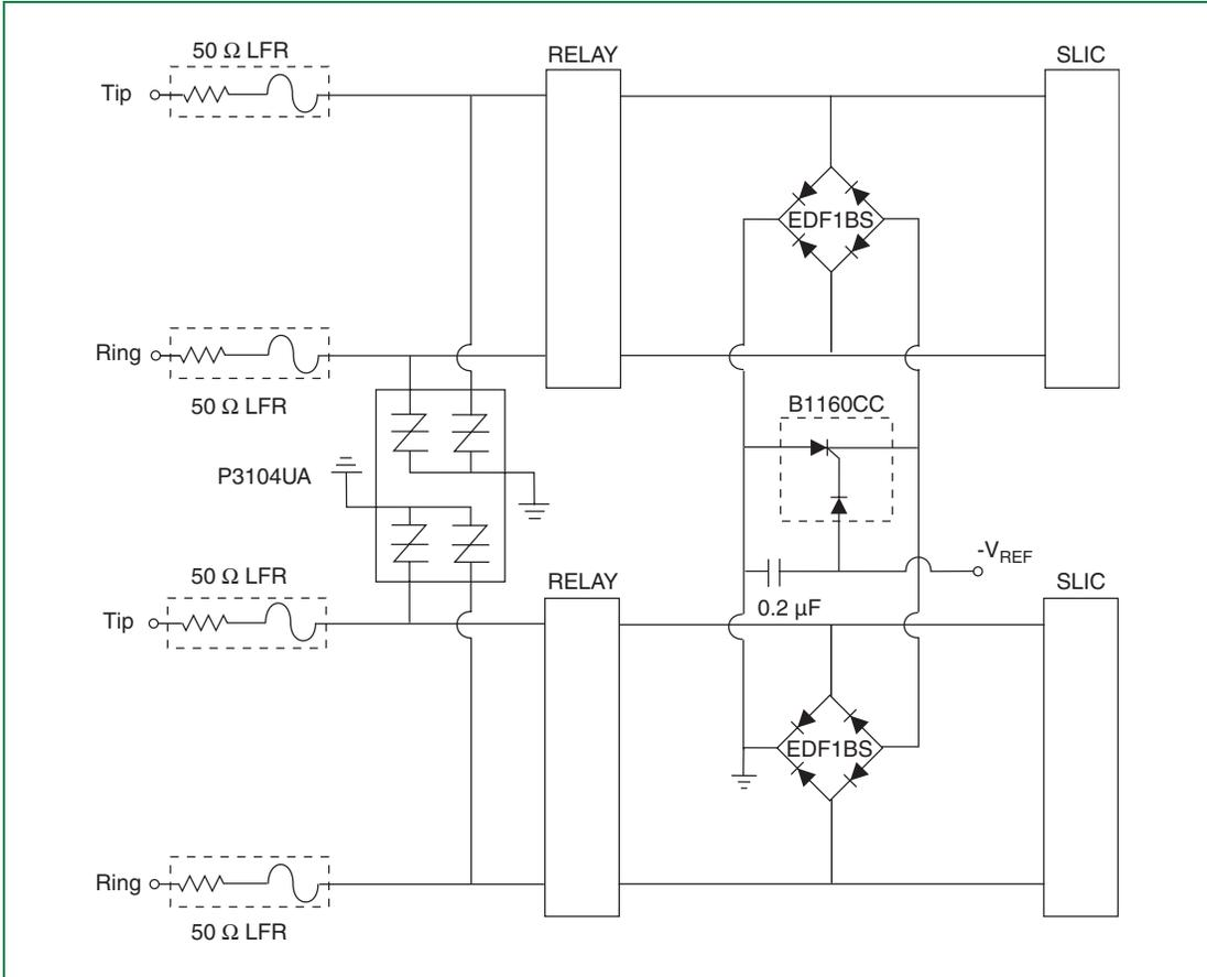
Figure 6.46 SLIC Protection with Diode Bridge
