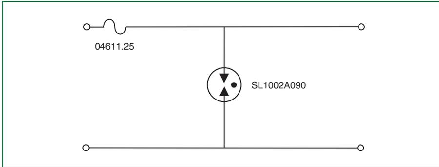
Figure 6.26 T3 Protection—Gas Plasma Arrester
