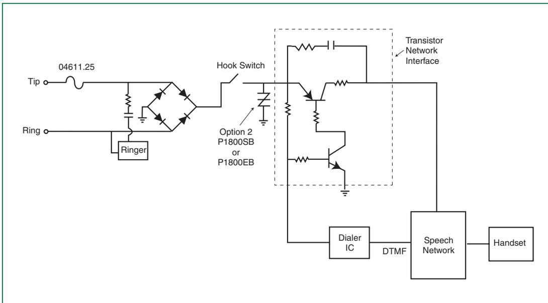
Figure 6.5 CPE Transistor Network Interface—Option 2
