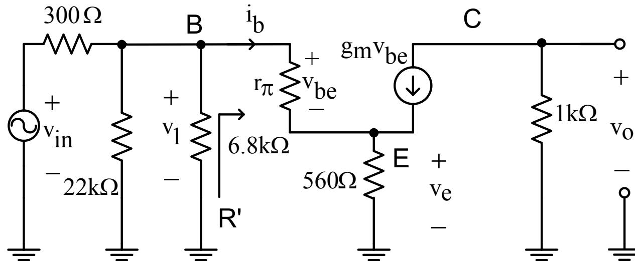
$$v_1 = \frac{(22k//6.8k//R')v_{in}}{22k//6.8k//R'+300}$$
