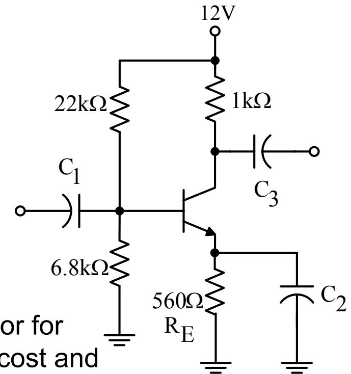
This is the minimum value for the bypass capacitor for this circuit. A larger value can be used, although cost and physical size usually impose limitations.
