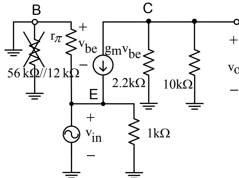
The  $56 k\Omega//12 k\Omega$  is shorted to ground and can be neglected in the small signal model. The analysis becomes difficult because the current source is between the output and the input node. Hence, use the T-model.
