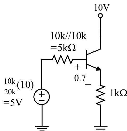
Using KVL at the input loop :
