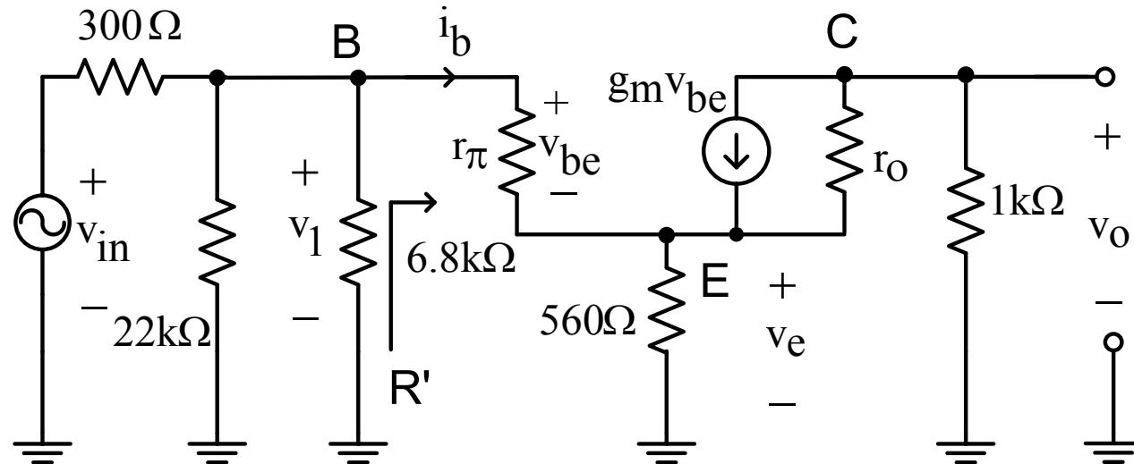
If the effect of  $r_o$  is neglected, the open circuit voltage gain :
