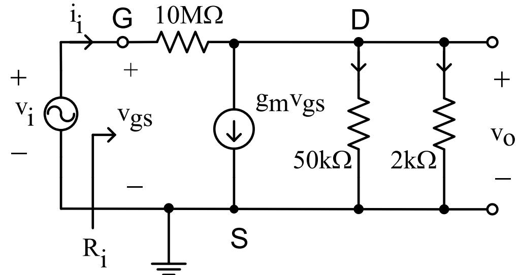
$$i_i \left( 1 + \frac{10M}{50k//2k} \right) = v_i \left( g_m + \frac{1}{50k//2k} \right)$$
