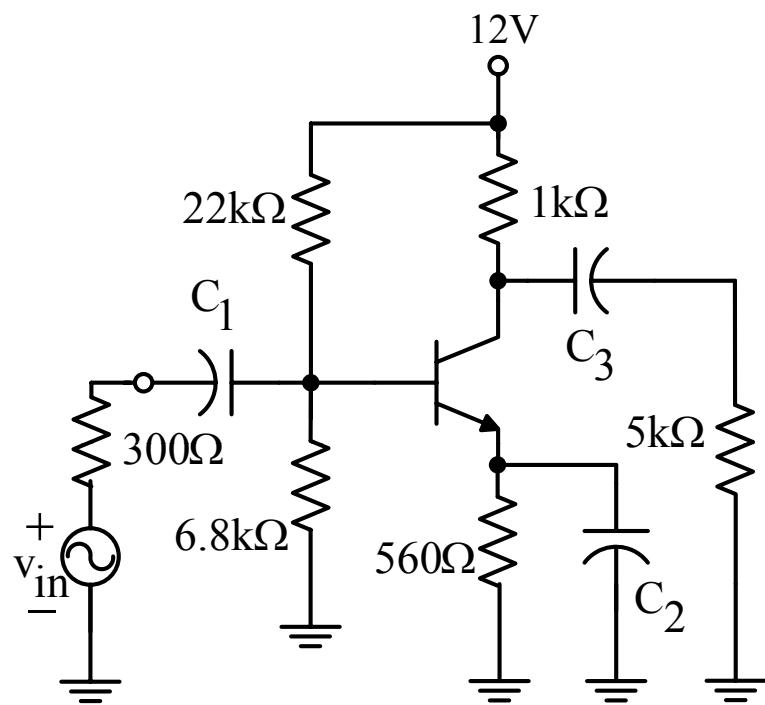
$$a_v = \frac{v_o}{v_{in}} = \frac{-g_m v_{be} (1\text{k} \parallel 5\text{k})}{v_{in}}$$
