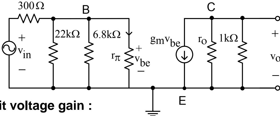
**Open circuit voltage gain :**
