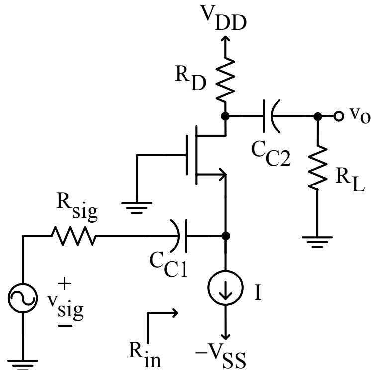
$$I_D = \frac{\mu_n C_{ox}}{2} \frac{W}{L} (V_{GS} - V_t)^2$$
