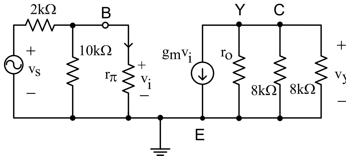
2. Determine the signal voltage at the B. The signal source gives a voltage of 10mV rms and has a resistance of  $300\Omega$ .
