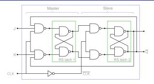
\* When CLK goes high, only the first latch is affected; the second latch retains its previous value (because  $\overline{\text{CLK}} = 0 \rightarrow R_2 = S_2 = 1$ ).
