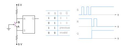
\* Because of the chatter, the S and R inputs may have multiple transitions when the switch is thrown from A to B.
