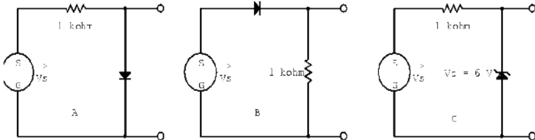
**Figure 14:** Circuits with a single ideal diode.
