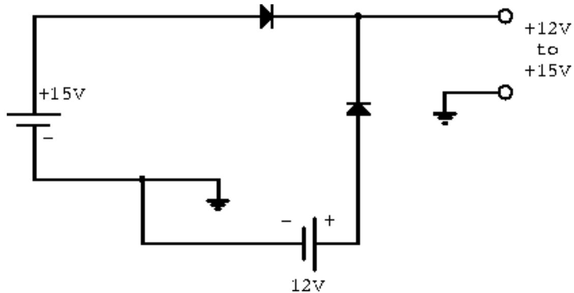
**Figure 13:** Diode OR gate.
