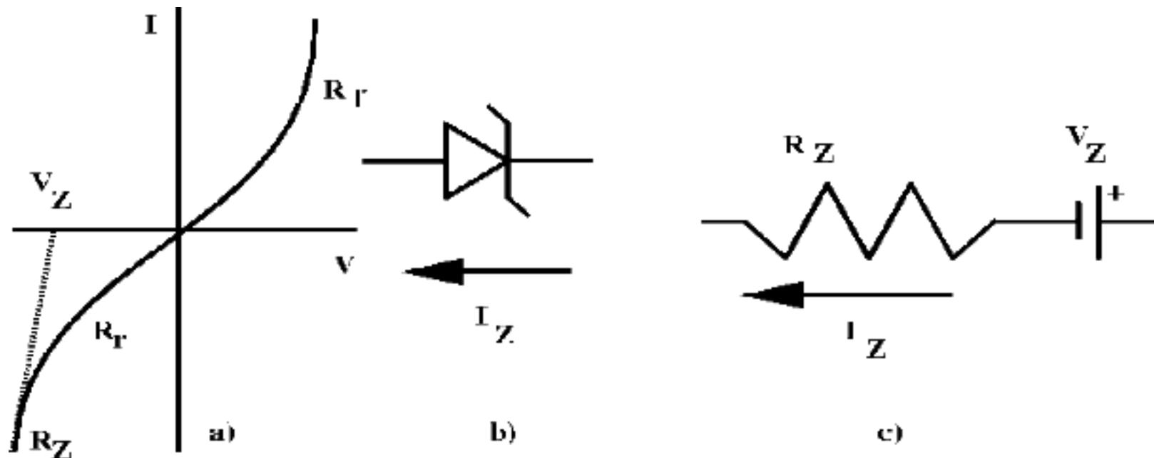
**Figure 6:** a) Current versus voltage of a zener diode, b) schematic symbol for a zener diode and c) equivalent circuit model of a zener diode in the reverse-bias direction.
