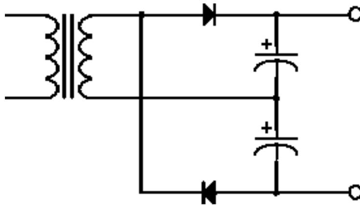
**Figure 10:** Voltage doubler circuit.
