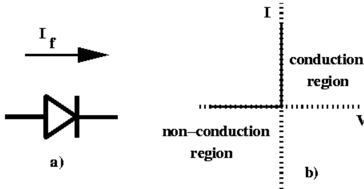
**Figure 4:** a) Schematic symbol for a diode and b) current versus voltage for an ideal diode.
