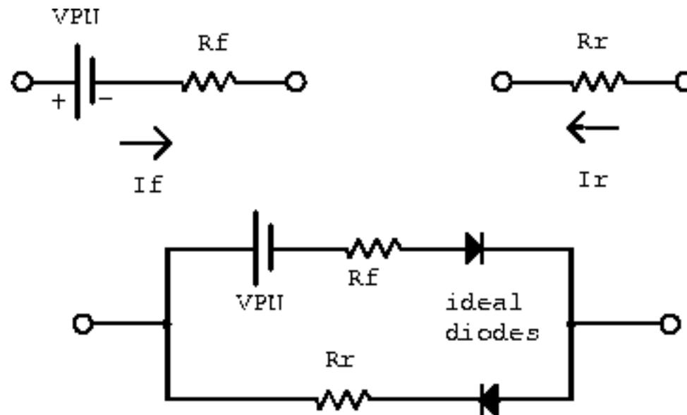
**Figure 5:** Equivalent circuit model of a junction diode.
