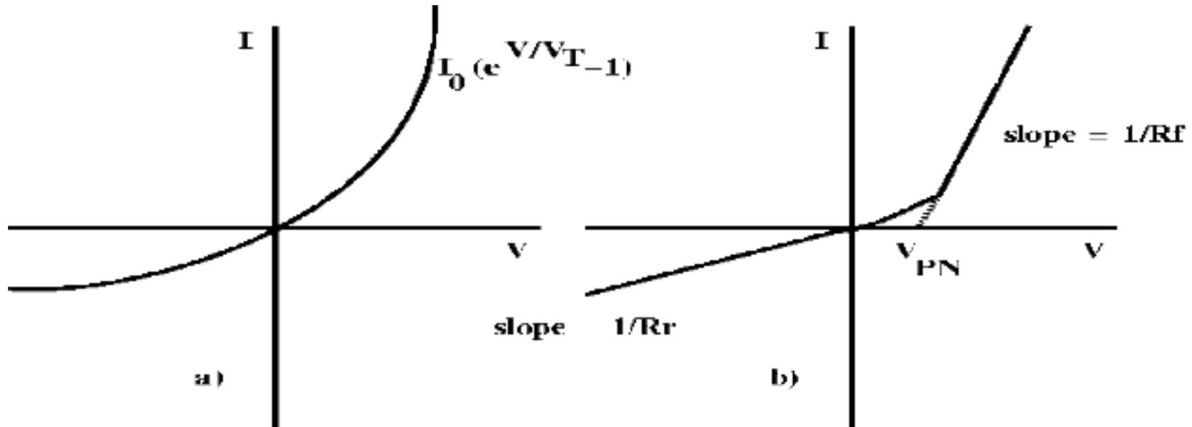
**Figure 3:** Current versus voltage a) in the PN junction region and b) for an actual PN diode.
