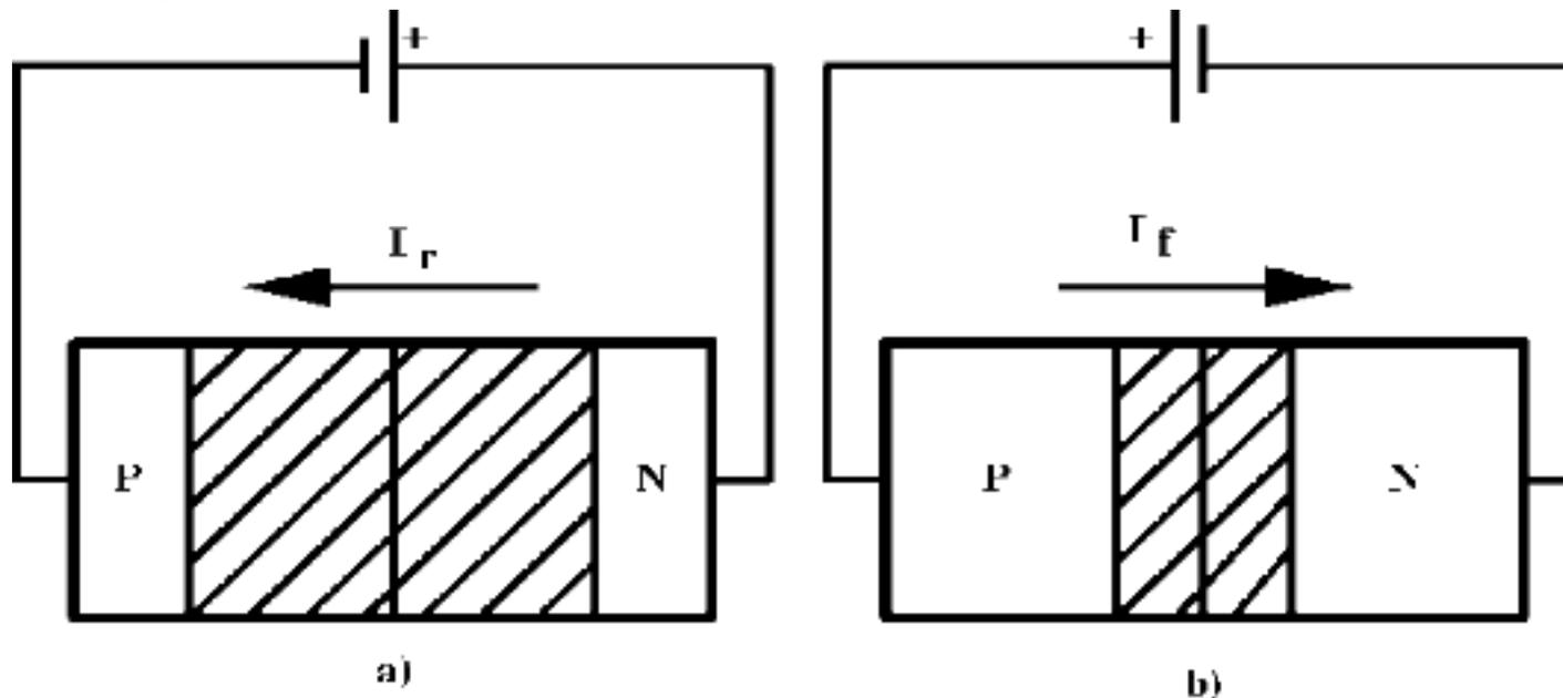
**Figure 2:** Diode circuit connections: a) reversed biased and b) forward biased.
