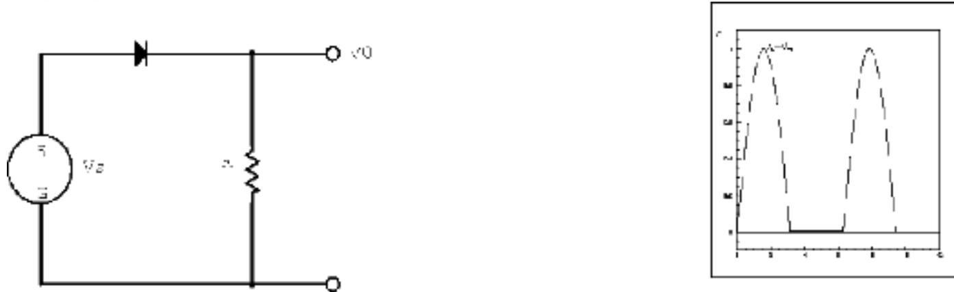
**Figure 7:** Half-wave rectifier and its output waveform.
