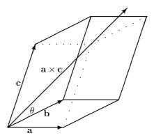
You notice the area of the base of the parallelepiped, the parallelogram determined by the vectors, **a** and **c** has area equal to  $|\mathbf{a} \times \mathbf{c}|$  while the altitude of the parallelepiped is  $|\mathbf{b}| \cos \theta$  where  $\theta$  is the angle shown in the picture between **b** and  $\mathbf{a} \times \mathbf{c}$ . Therefore, the volume of this parallelepiped is the area of the base times the altitude which is just
