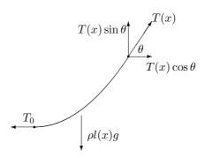
In this picture,  $\rho$  denotes the density of the chain which is assumed to be constant and g is the acceleration due to gravity. T(x) and  $T_0$  represent the magnitude of the tension in the chain at x and at 0 respectively, as shown. Let the bottom of the chain be at the origin as shown. If this chain does not move, then all these forces acting on it must balance. In particular,
