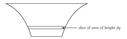
The reason you would be interested in that long thin slice of area having essentially the same depth, say at y feet is because the pressure in the water at that depth is constant and equals 62.5y pounds per square foot<sup>2</sup>. Therefore, the total force the water exerts on the long thin slice is
