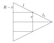
and so by similar triangles,  $l_1 = lr/(R-r)$ . Therefore, substituting this into the above, the area of this frustrum is
