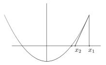
In this picture, a first approximation, denoted in the picture as  $x_1$  is chosen and then the tangent line to the curve y = f(x) at the point  $(x_1, f(x_1))$  is obtained. The equation of this tangent line is
