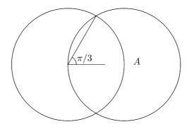
The circles bounding these disks are  $x^2 + y^2 = 1$  and  $(x - 1)^2 + y^2 = x^2 + y^2 - 2x + 1 = 1$ . Therefore, in polar coordinates these are of the form r = 1 and  $r = 2\cos\theta$ .
