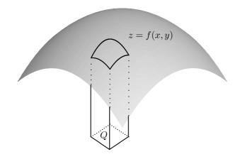
In this picture, the volume of the little prism which lies above the rectangle Q and the graph of the function would lie between  $M_Q(f) v(Q)$  and  $m_Q(f) v(Q)$  where
