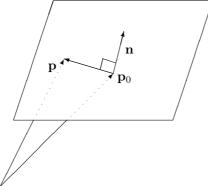
Expressed equivalently, the plane is just the set of all points  $\mathbf{p}$  such that the vector,  $\mathbf{p} - \mathbf{p}_0$  is perpendicular to the given normal vector,  $\mathbf{n}$ .
