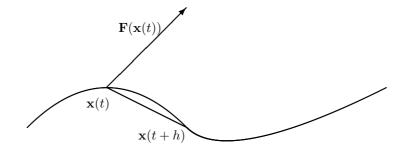
In this picture, the work done by a constant force,  $\mathbf{F}$  on an object which moves from the point  $\mathbf{x}(t)$  to the point  $\mathbf{x}(t+h)$  along the straight line shown would equal  $\mathbf{F} \cdot (\mathbf{x}(t+h) - \mathbf{x}(t))$ . It is reasonable to assume this would be a good approximation to the work done in moving along the curve joining  $\mathbf{x}(t)$  and  $\mathbf{x}(t+h)$  provided h is small enough. Also, provided h is small,
