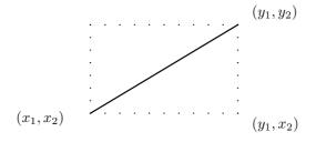
There are two points in the plane whose Cartesian coordinates are  $(x_1, x_2)$  and  $(y_1, y_2)$  respectively. Then the solid line joining these two points is the hypotenuse of a right triangle which is half of the rectangle shown in dotted lines. What is its length? Note the lengths of the sides of this triangle are  $|y_1 - x_1|$  and  $|y_2 - x_2|$ . Therefore, the Pythagorean theorem implies the length of the hypotenuse equals
