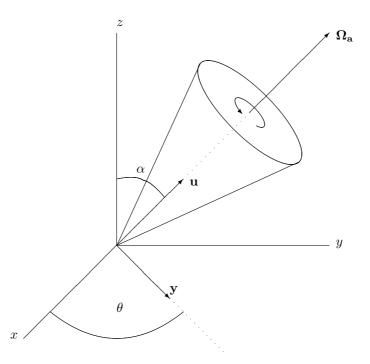
For the purpose of this discussion, consider the top as a large number of point masses,  $m_i$ , located at the positions,  $\mathbf{r}_i(t)$  for  $i = 1, 2, \dots, N$  and these masses are symmetrically arranged relative to the axis of the top. As the top spins, the axis of symmetry is observed to move around the z axis. This is called precession and you will see it occur whenever you spin a top. What is the speed of this precession? In other words, what is  $\theta'$ ?
