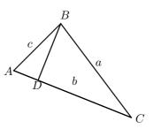
The area of this triangle would be the sum of the two right triangles formed. Thus this area would be  $\frac{1}{2}(\overline{BD})(\overline{AD} + \overline{CD}) = \frac{1}{2}(\overline{BD})b$ . In words, the area of the triangle equals one half the base times the height. This also holds if the height and base are chosen with respect to any other side of the triangle.
