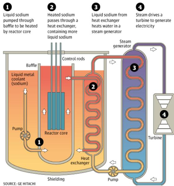
Fig-4.5-Fast breeder reactor
