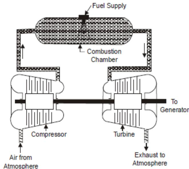
Fig-2.10-Open Cycle Gas Turbine
