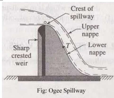
Fig-3.6- over flow spillway
