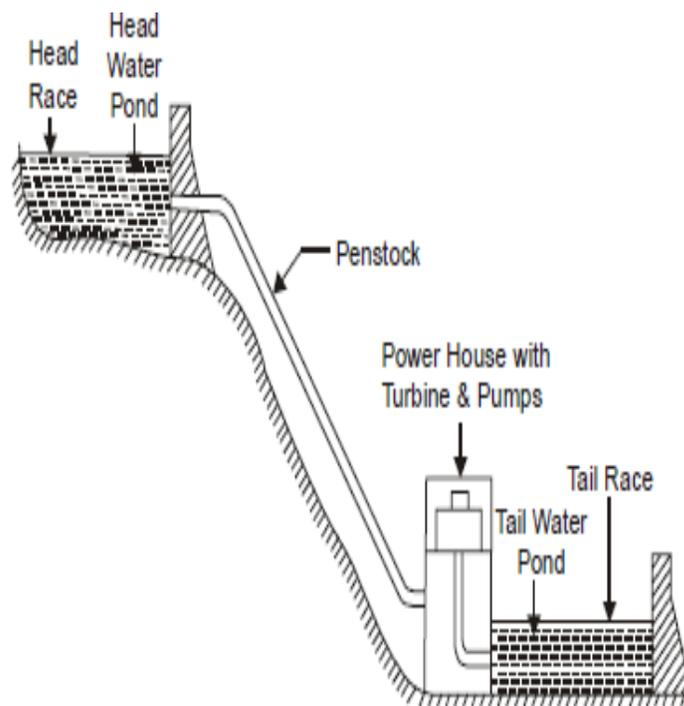
Fig-3.3-Pumped storage plant
