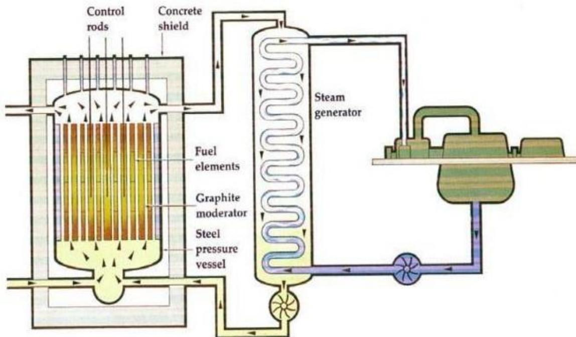
Fig-4.6- Gas cooled reactor
