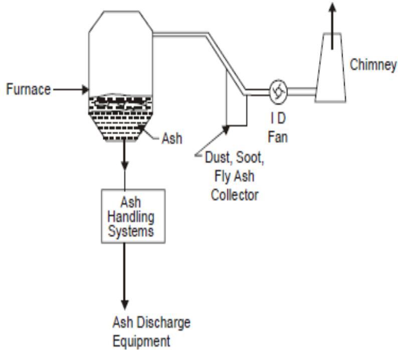
Fig-1.11-Ash handling system
