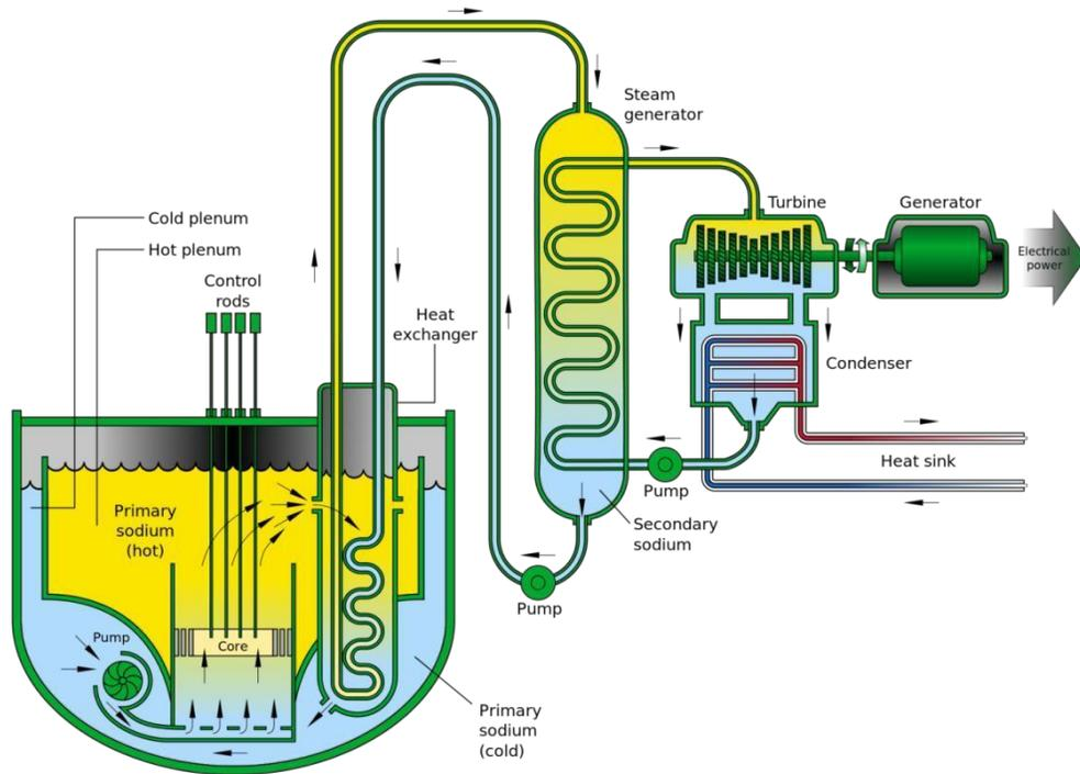
FIG.4.4-Sodium Graphite reactor
