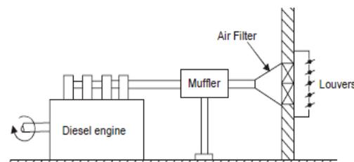
Fig-2.7-Air Intake System
