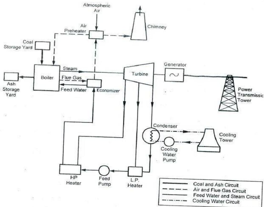
Fig-1.2-Layout of different circuits
