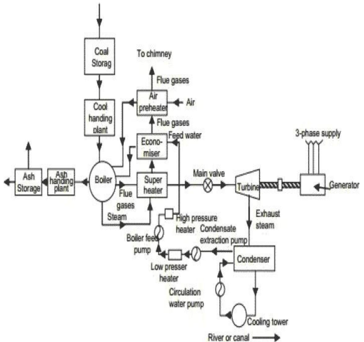
Fig-1.1- layout of steam power plant
