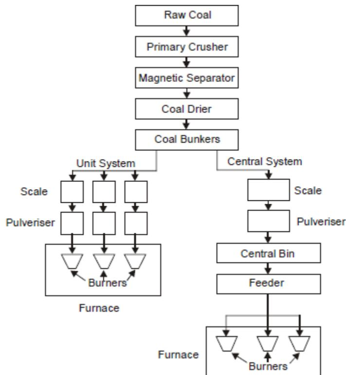
Fig-1.21- Components of pulverised fuel burning
