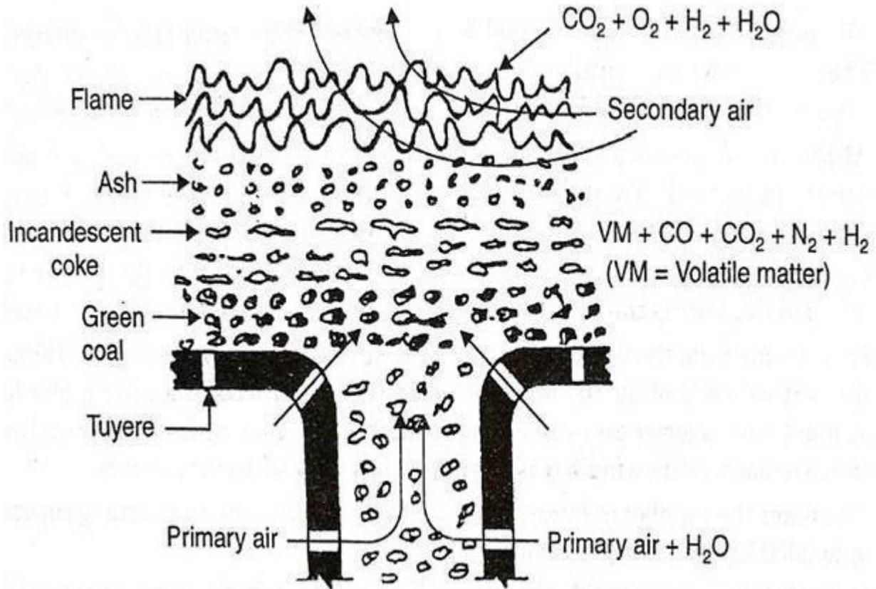
Fig-1.16- Underfeed Principle
