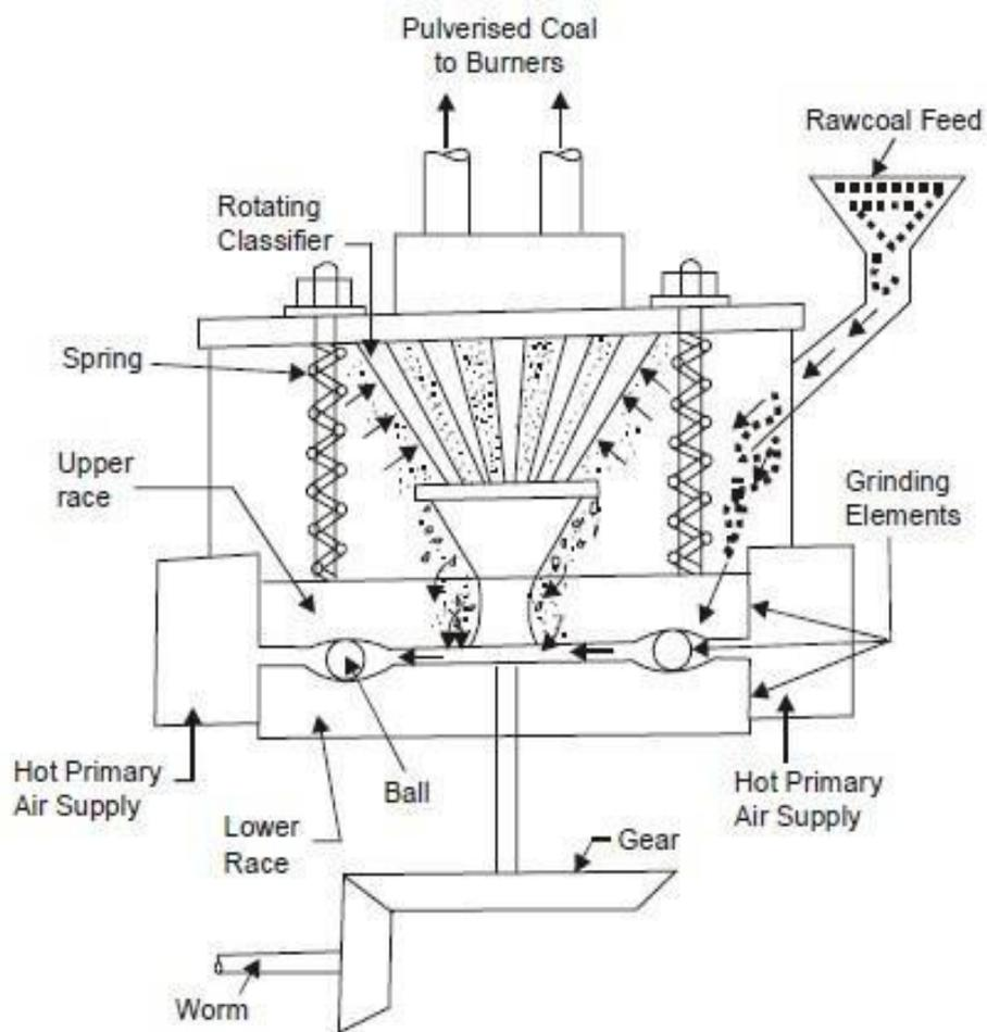
Fig-1.23-Ball and Race Mill
