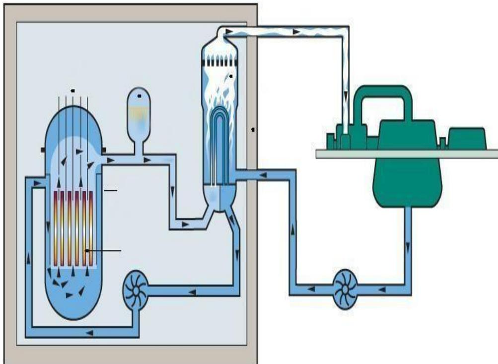
Fig-4.2- pressurized water reactor
