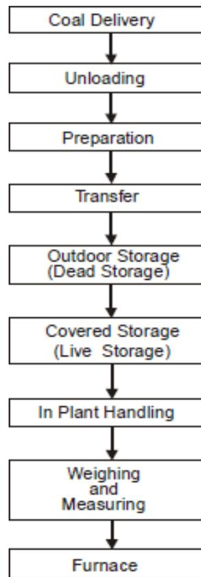
Fig-1.3-steps in coal handling
