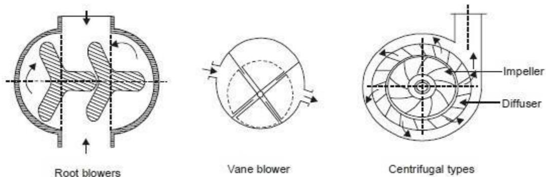
The blowers are usually driven from the engine cranks shaft by mean of Spur, helical or herringbone gears, silent chains or V-belts at a speed 2-3 times the engine speed. In the case of turbo-supercharger, the super charger is coupled to a gas turbine in which the exhaust of the engine is expanded.
