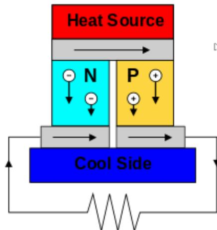
Fig-2.14- thermo electric system
