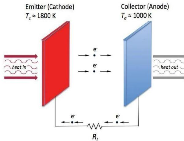
Fig-2.15- Thermo Ionic Converter
