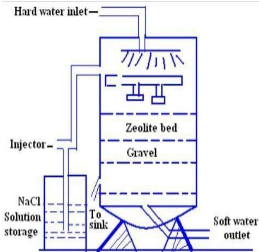
Fig-1.35- Zeolite Process
