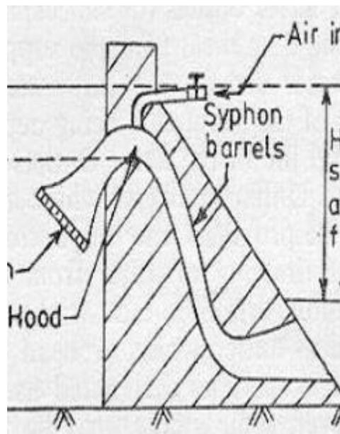
Fig-3.7- siphon spillway
