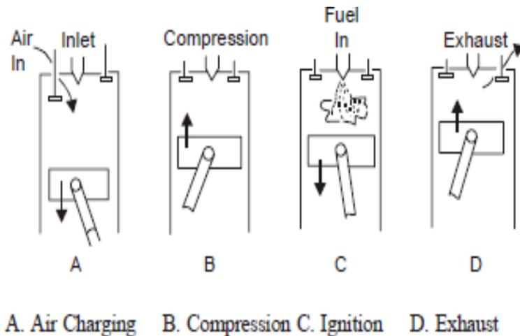
Fig-2.1-Illustrating operation of an IC Engine principle
