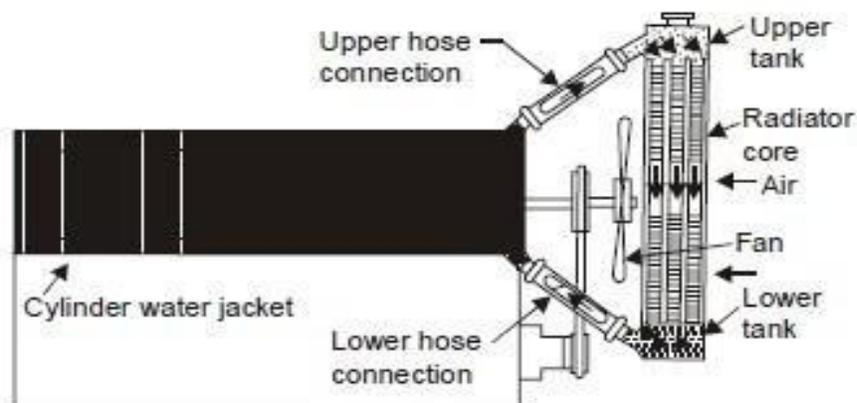
Fig-2.8-Natural Circulation Cooling System
