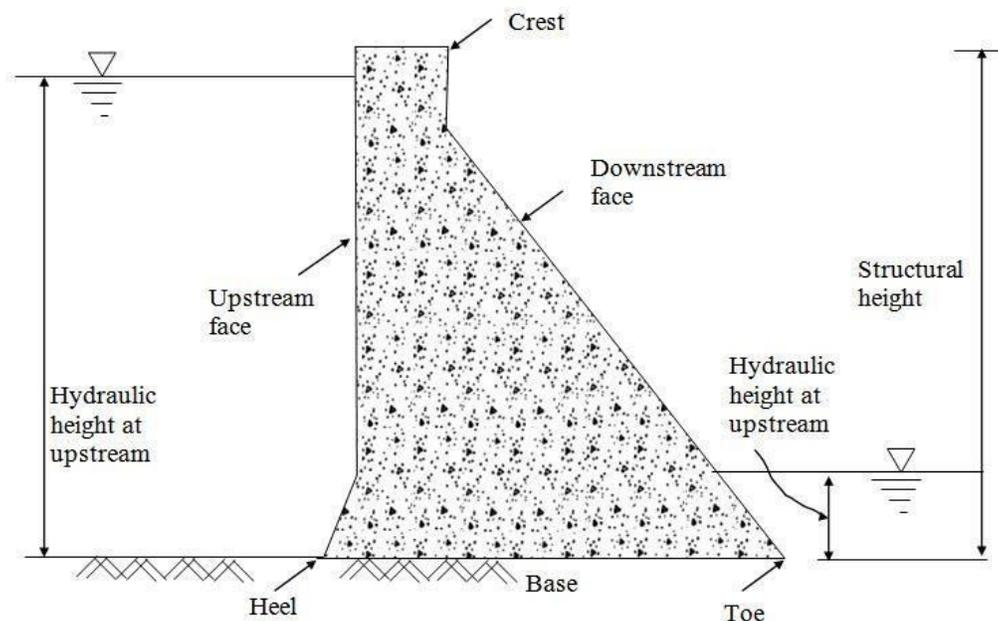
Fig-3.4- Gravity dam
